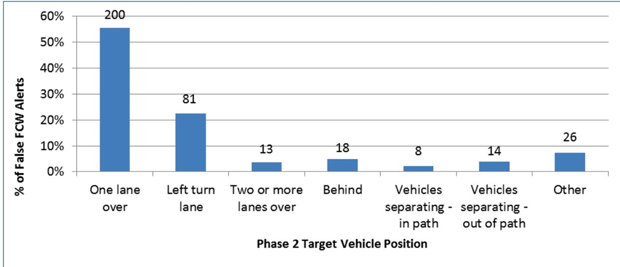
**Figure 13. Detailed Breakdown of Phase 2 False FCW Alerts**
