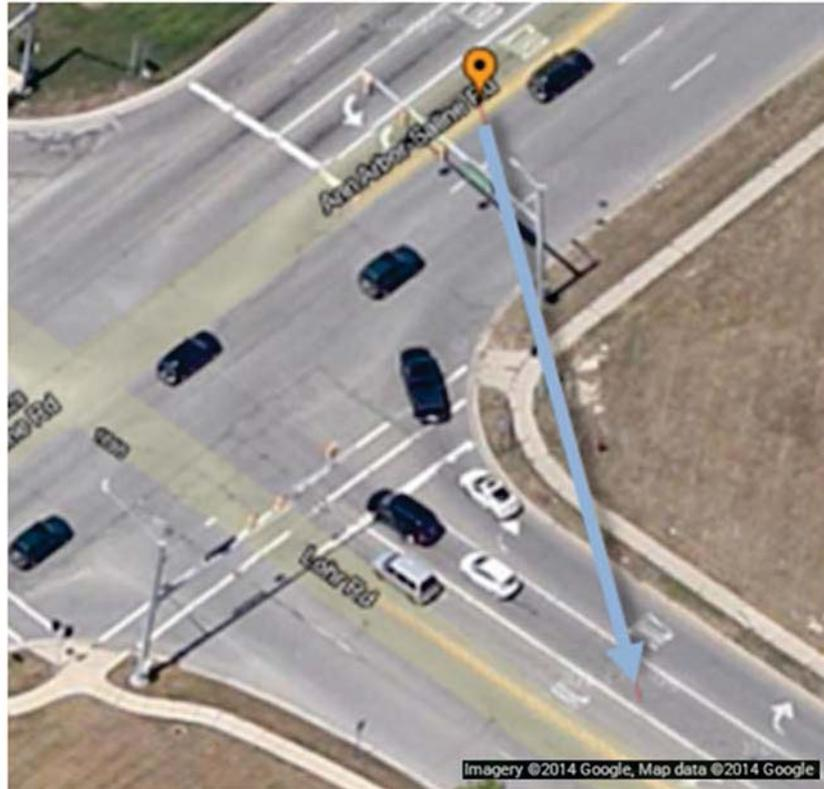
**Figure 32 – IMA Scenario Examples: RV and/or HV Are Traveling at Speeds Such That Collision Can Be Avoided Without Having to Brake**
