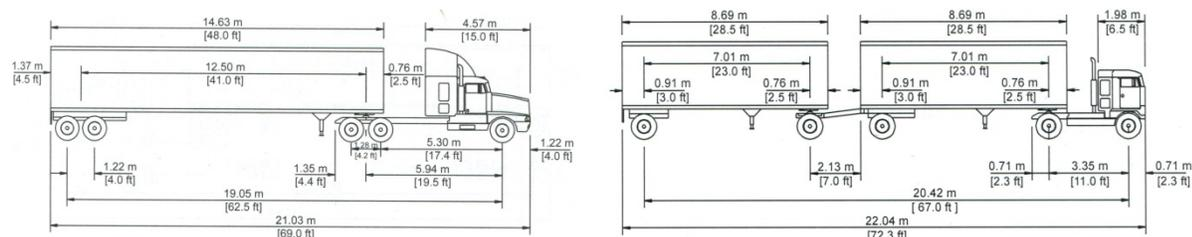
**Figure 12-12. Example tractor-semitrailer configurations (from AASHTO, 2011, *A policy on geometric design of highways and streets*, Washington, DC. Used with permission).**
