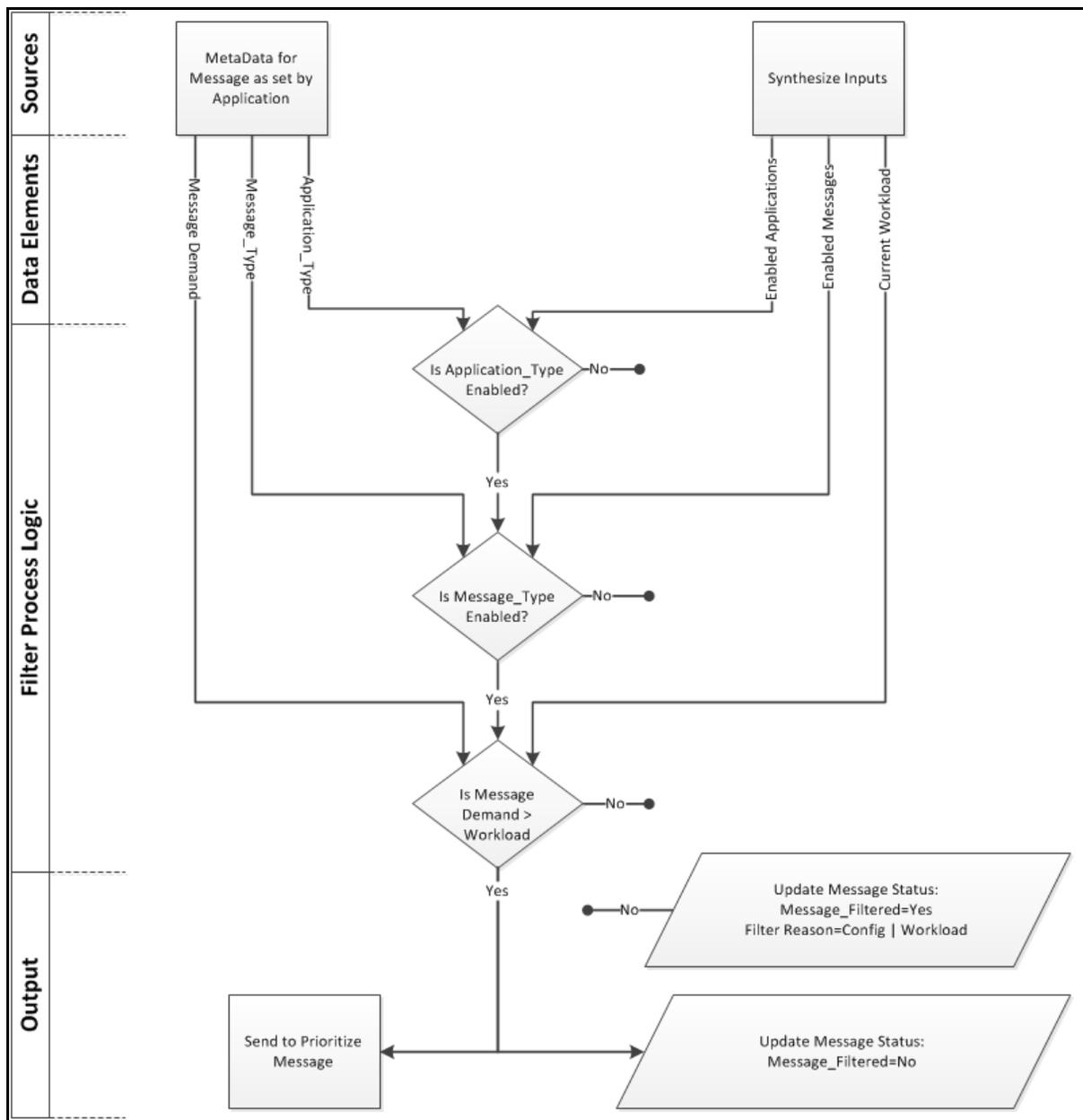
**Figure 12-8. Example of a Filtering process applied to messages that are intended for the driver.**
