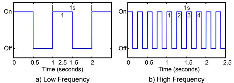
**Duty Cycle:** The percent of time within a cycle that the sign is in the “on” state. The example shows a signal with 80% duty cycle (“on” for 0.8s and “off” for 0.2s).
