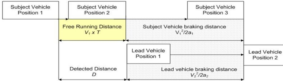
**Basic Equation:**  $D = V_1 \times T + (V_1^2/2a_1 - V_2^2/2a_2)$
