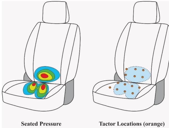
**Example of a detectable vibration measurements from seat pan and and back rest surfaces of a *vibrotactile seat display* [2]:**
