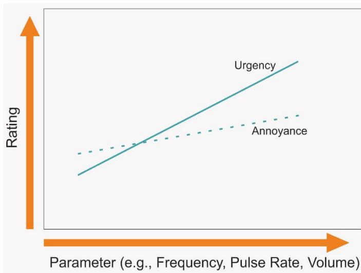
The figure on the left illustrates the relationship between urgency and annoyance when varying a signal characteristic, such as frequency, pulse rate, or volume, of an example auditory warning.
