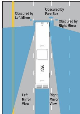
**Figure 12-15. Depiction of typical transit bus blind spots (adapted from Thorpe, Duggins, McNeil, & Mertz, 2002).**
