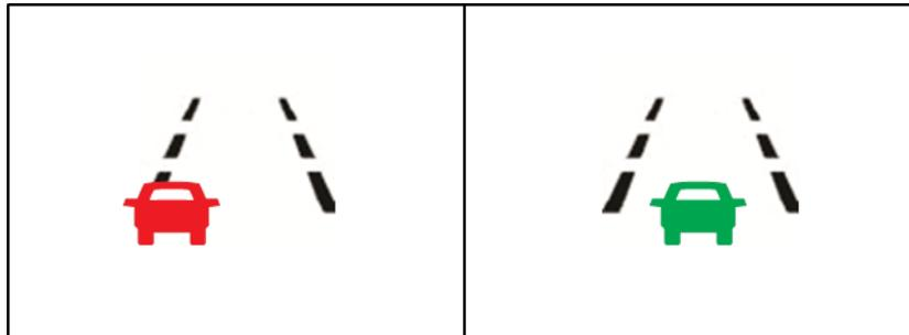
This image shows a hypothetical lane centering status display. The left image indicates that the car is not centered in the lane. The non-centered status is provided through position of the car on the lane display, as well as through the red color of the car. The right image indicates that the car is centered in the lane. The centered status is portrayed through showing the car in the center of the lane display and through the green color of the car.
