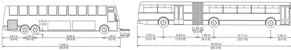
Figure 12-13. Example city transit bus configurations (from AASHTO, 2011, *A policy on geometric design of highways and streets, Washington, DC*. Used with permission).
