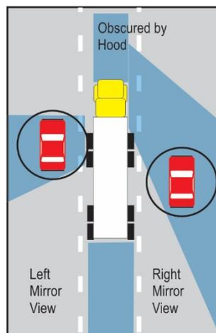
Figure 12-14. Depiction of heavy truck blind spots (adapted from FMCSA, n.d.).
