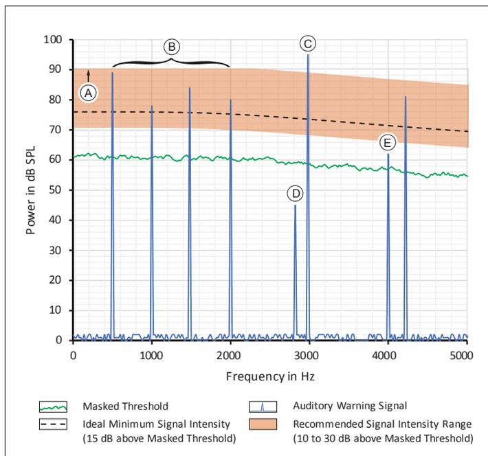
This graph shows the frequency domain of a hypothetical warning signal superimposed on the MT for noise conditions while driving<sup>1</sup>.
