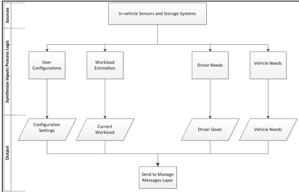
Figure 12-6. Overall framework for the Synthesize Inputs layer.
