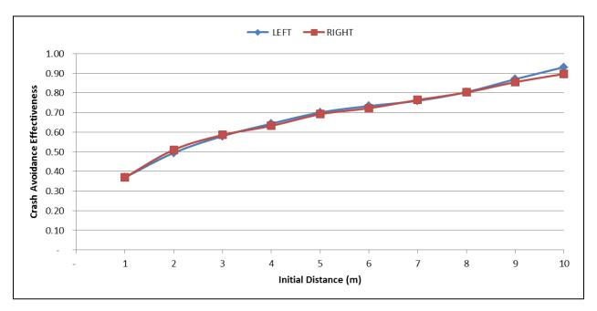
Figure 10. IMA-S Crash Avoidance Effectiveness versus HV Distance to Intersection
