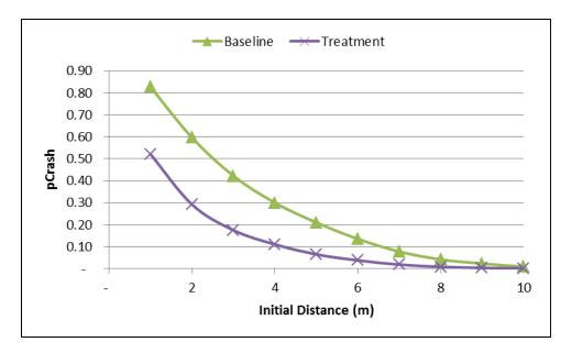
Figure 9. IMA-S Crash Probability versus HV Distance to Intersection – RV Approach (Right)
