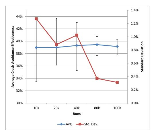
Figure 14. Average BSW/LCW Effectiveness Estimates versus Number of Simulated Runs
