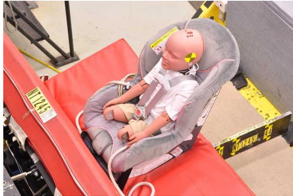
Figure 3. Hybrid III 3YO with lower legs removed.
