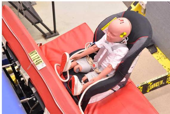
Figure 4. Hybrid III 3YO with lower legs attached alongside thighs.
