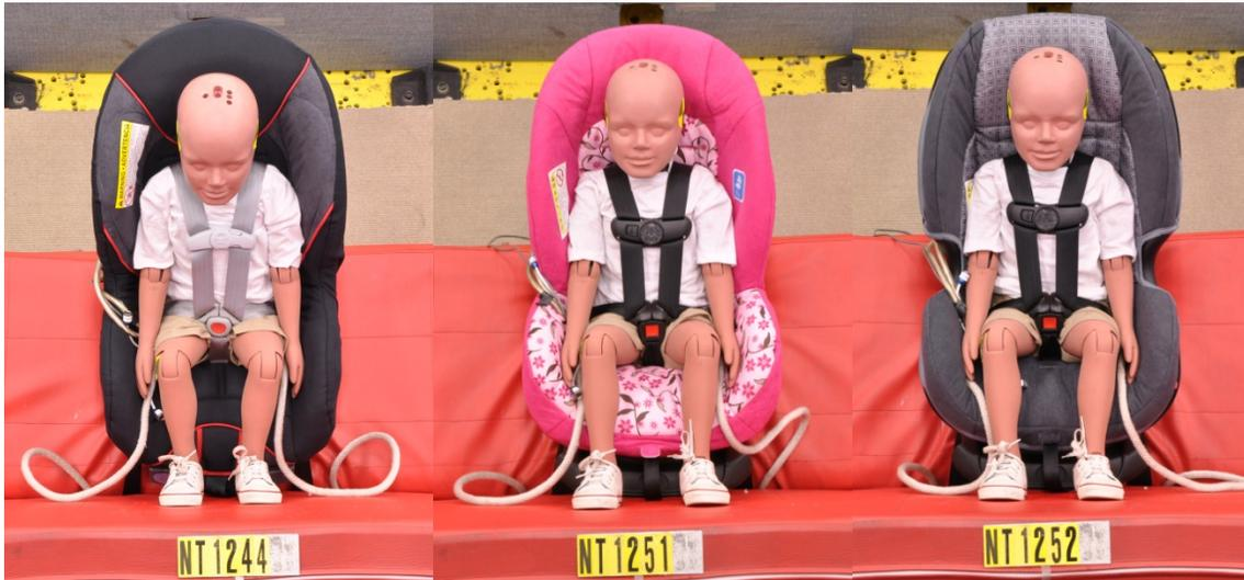
Figure A2. Bent leg posture evaluated in initial test series.
