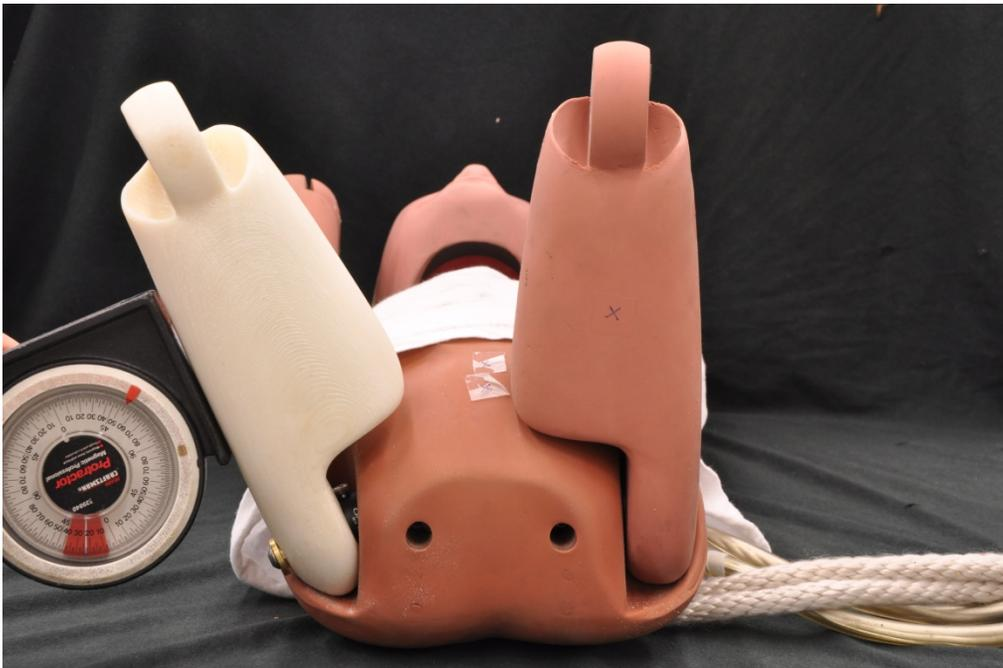
Figure A6. Modified thigh model with ball joint compared to standard thigh and standard joint.
