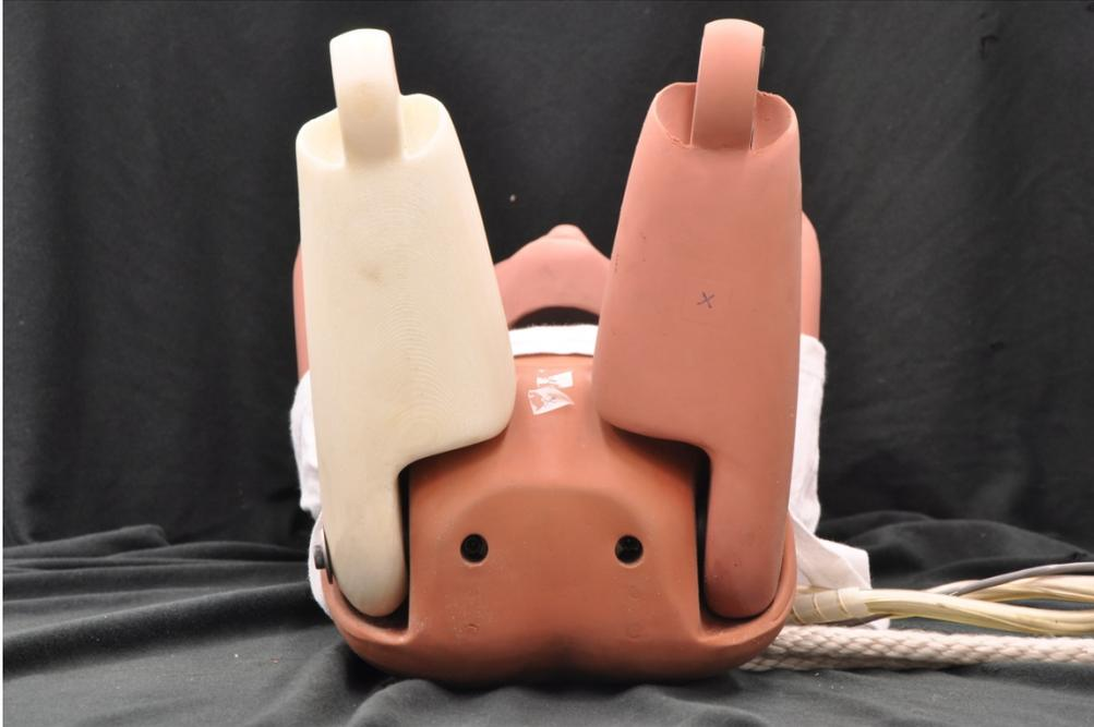
Figure A5. Modified thigh model compared to standard thigh, with standard joint used for each.
