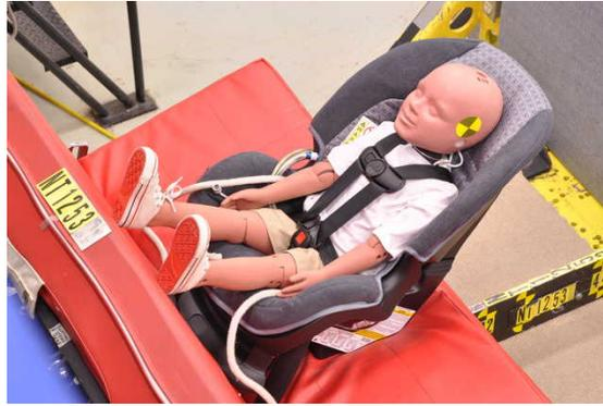
Figure 1. Intact Hybrid III 3YO in convertible CRS.
