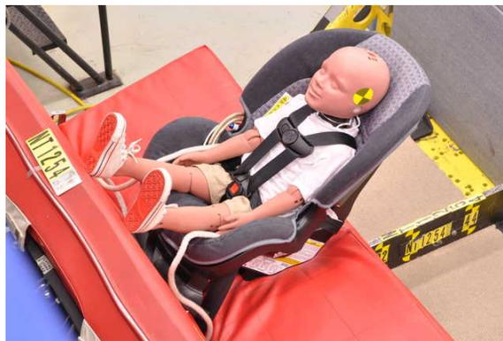
Figure 2. Hybrid III 3YO with knee joint stops removed.
