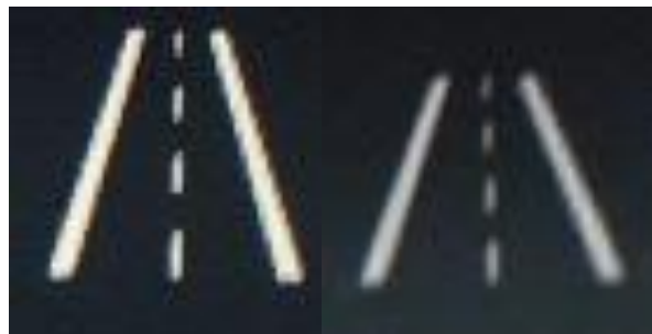
Figure 45. Lateral Control Features Active (Left) and in Standby (Right) in the Volvo XC90
