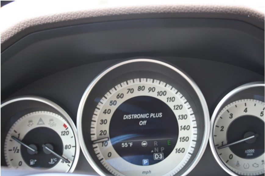
Figure 41. Both Lateral and Longitudinal Sytems Deactivated in the Mercedes E350
