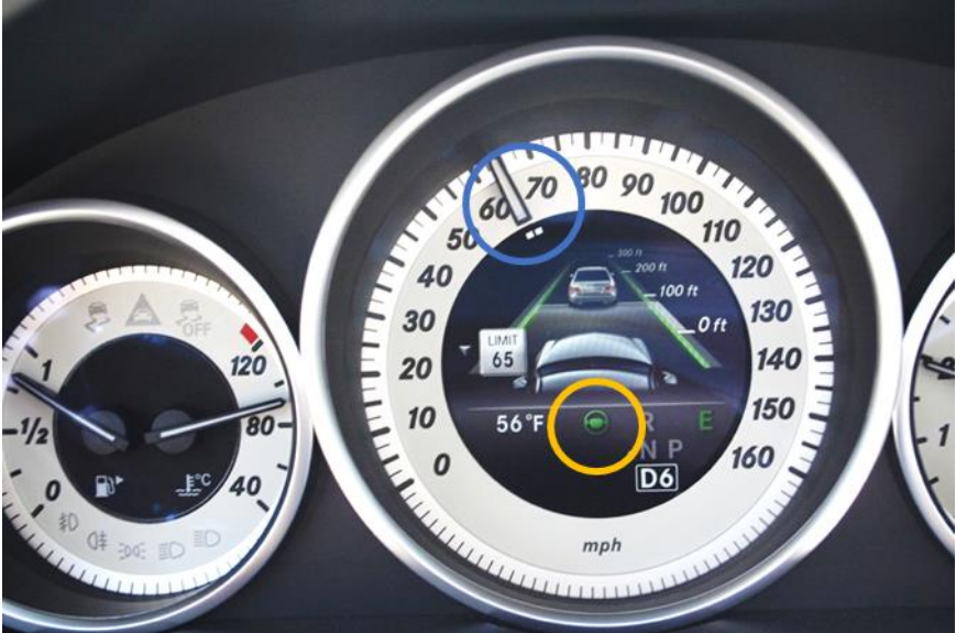
Figure 40. Lateral (Yellow Circle) and Longitudinal (Blue Circle) Systems Active in the Mercedes E350
