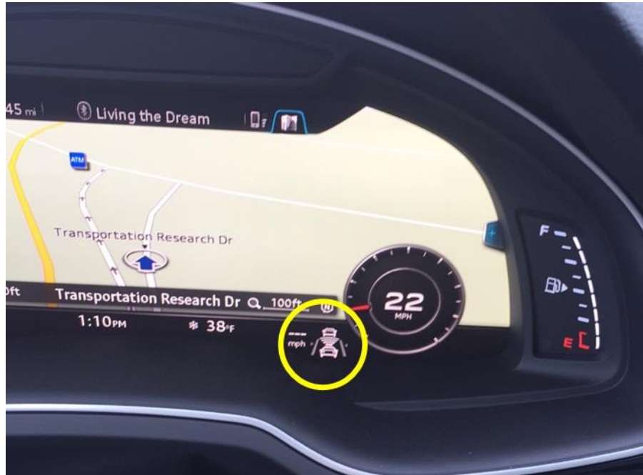
Figure 33. Instrument Cluster in the Audi Q7 Showing the Location of the Lateral and Longitudinal Icons (Yellow Circle)
