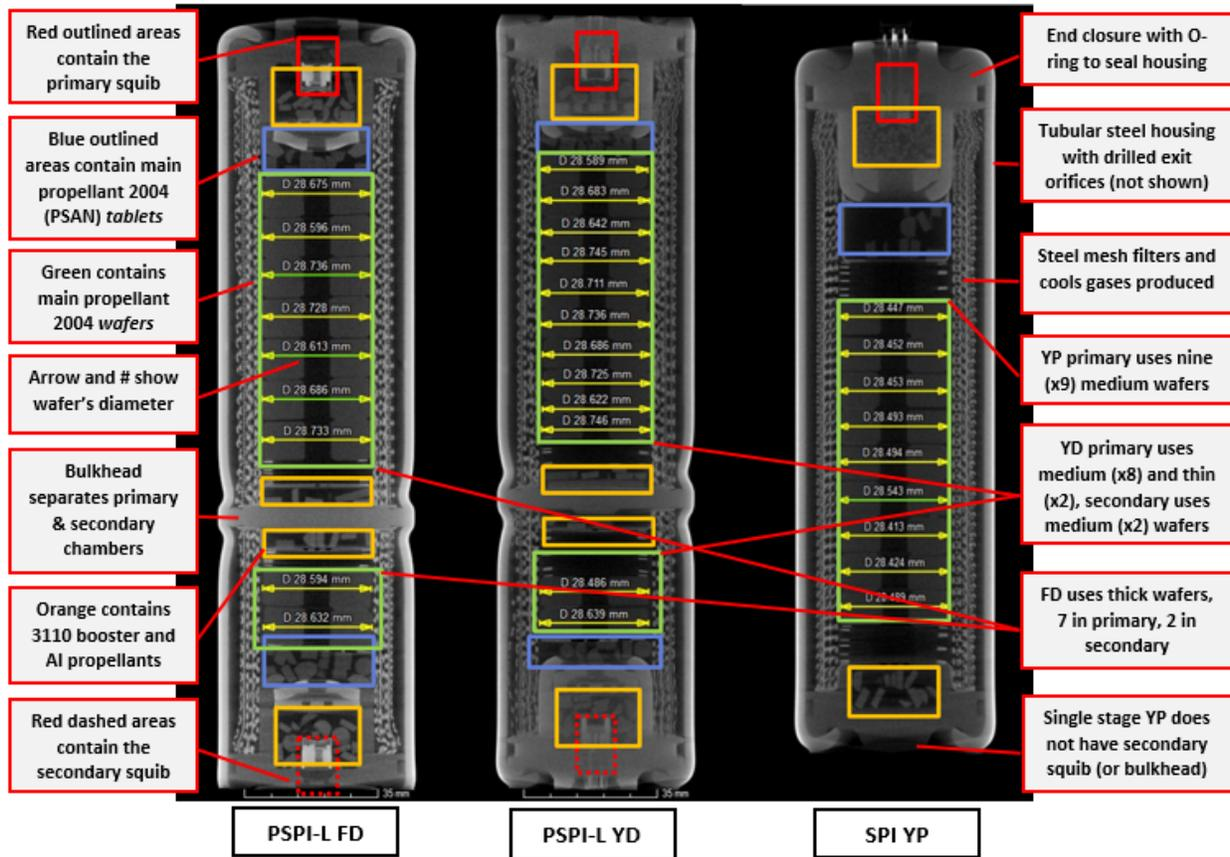
Figure 1. CT Scans of GM Inflators PSPI-L-FD, PSPI-L YD, and SPI YD <sup>20</sup>
