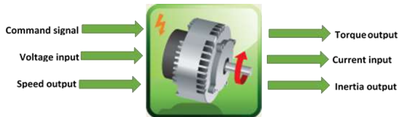
Figure 6-12 - Autonomie Electric Machine Model Input/Output
