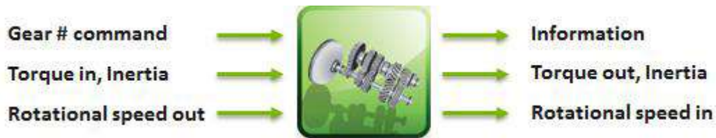
Figure 6-6 - Automatic Gearbox Model Input/Output
