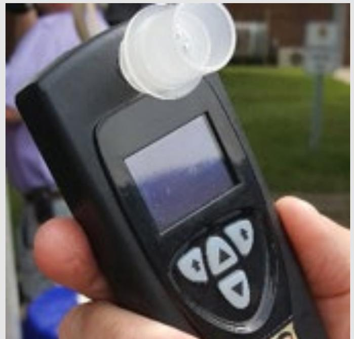
*A breath testing device used in Maryland's ignition interlock program.*
