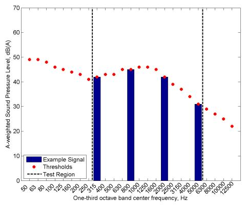
Figure 3. Example of a Four-Component Signal at Threshold at 0 km/h
