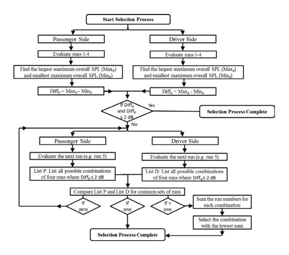
Figure 10. Selection process to determine "first four valid test run sound files within 2dBA"
