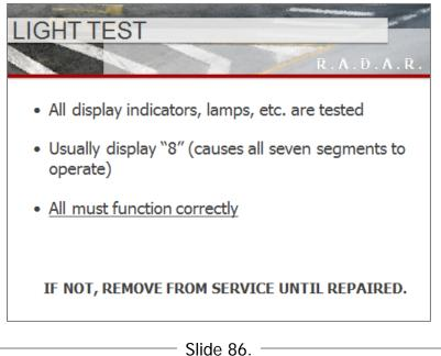
Manufacturer testing guidelines are an absolute minimum. Operator manual should be available.
