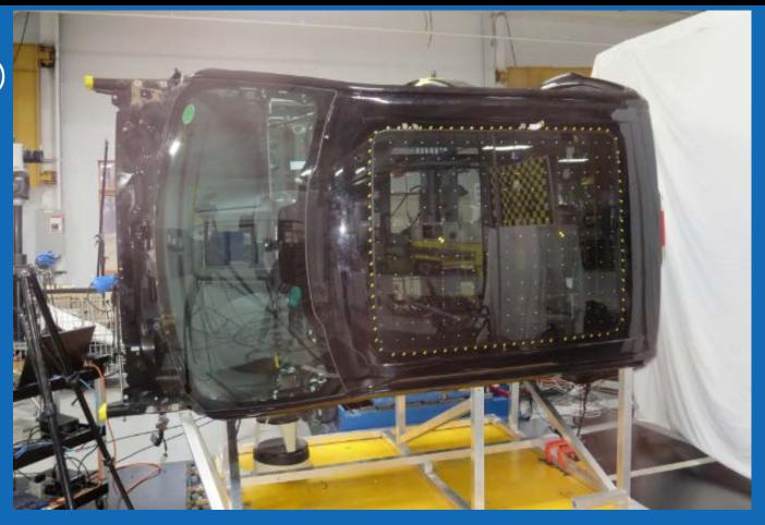
Mounted sideways Glass pre-broken on both sides (except ProTEC II) 75 mm offset pattern per FMVSS No. 226
