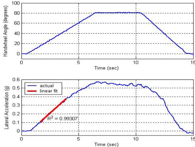
**Figure 2.** Sample steering wheel angle and lateral acceleration data recorded during a Slowly Increasing Steer test. The linear range used to define the lateral acceleration regression line is highlighted.
