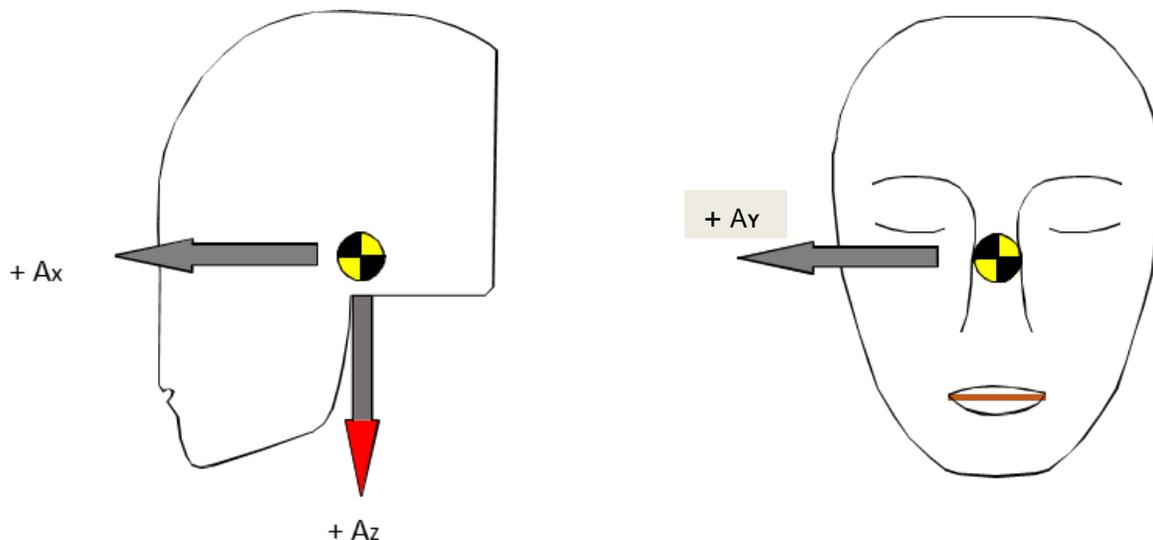
**Figure 5.** FMH Accelerometer Sign Convention
