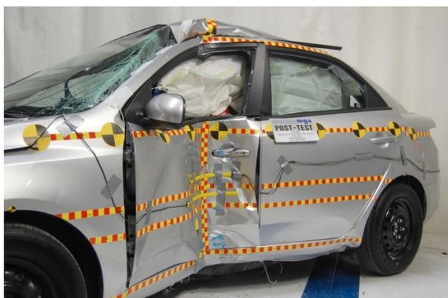
\_\_12 Post Test 3/4 Rear View of Impact Zone
