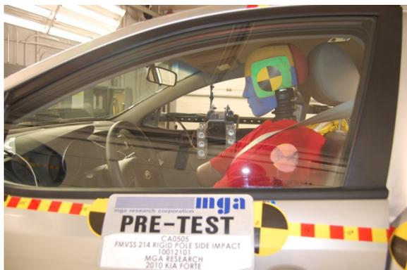
\_\_8 Test Dummy w/Door Open
