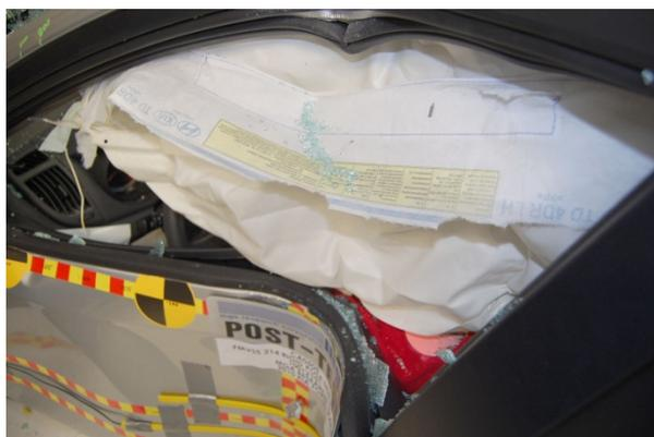
\_\_9 Post Test Interior of Front Door Showing Dummy Impact Locations (thru opposite window w/dummy removed)
