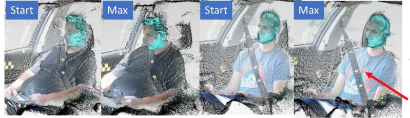
Head Tracking Output Showing Landmark and Head CG Trajectory
