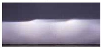
$\mathbf{B}$  – Headlights produce a fuzzy, less distinct cut-off (line) between the lighter area below and the darker area near the top of the picture.
