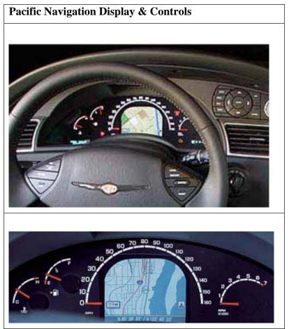
Figure 1. 2005 Chrysler Pacifica in-dash navigation system
