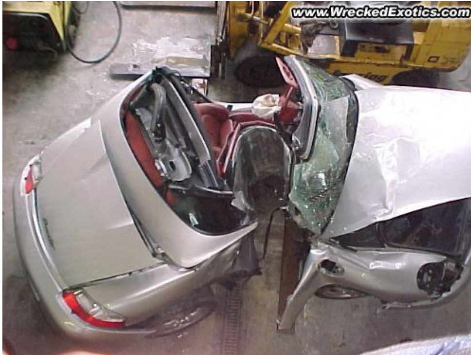
Figure 2-19. Porsche Boxster following extreme side intrusion [59] (used with permission).
