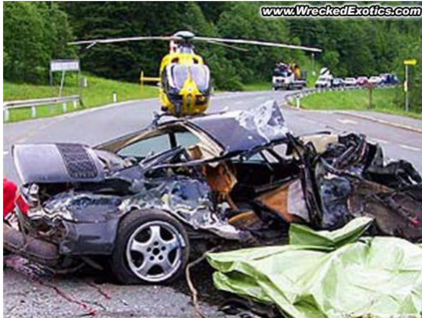
Figure 2-17. Porsche 911 following high speed crash [57] (used with permission).
