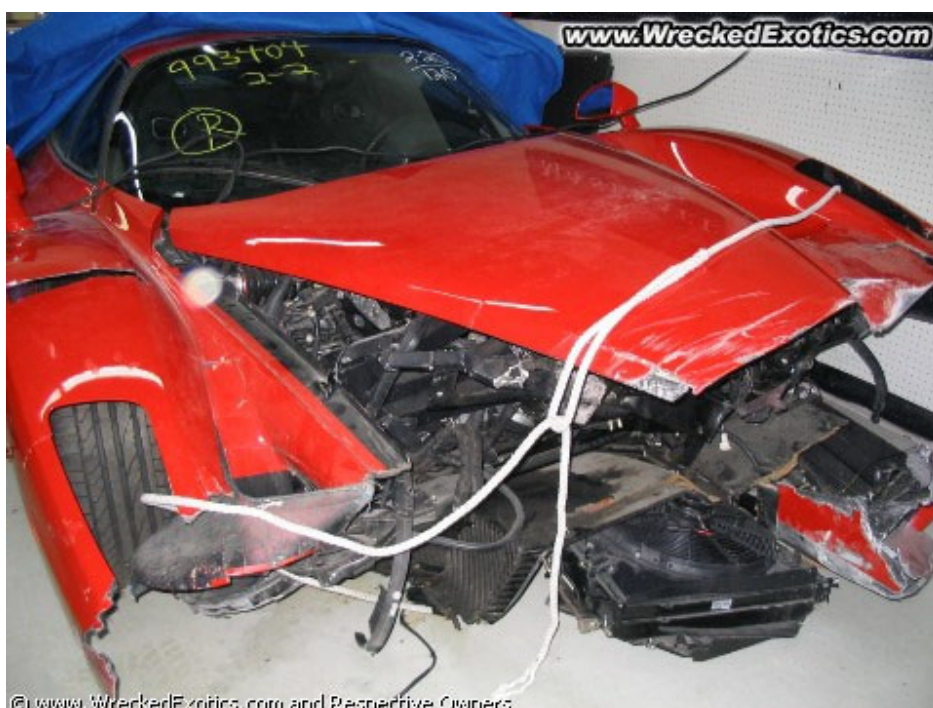
Figure 2-10. Ferrari Enzo following frontal impact [50] (used with permission).
