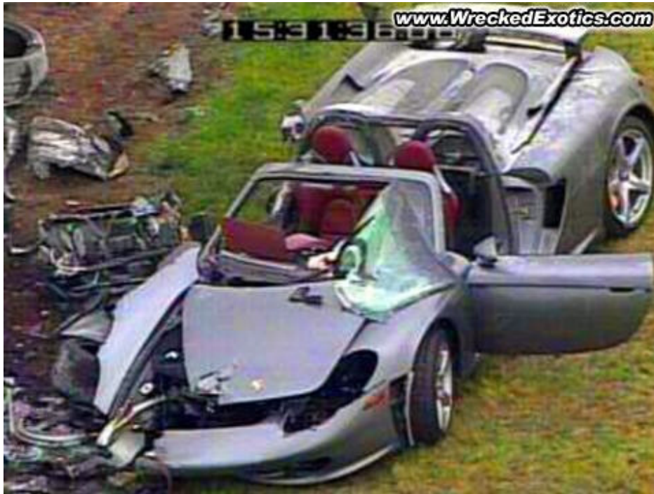
Figure 2-5. Porsche Carrera GT following side impact [45] (used with permission).
