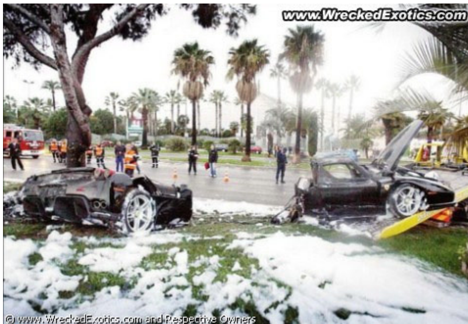
Figure 2-8. Ferrari Enzo following side impact [48] (used with permission).
