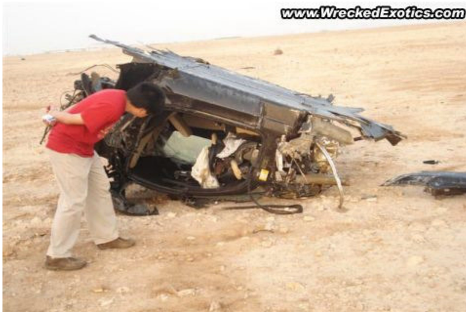
Figure 2-14. McLaren SLR following multiple rolls from high speed crash [54] (used with permission).
