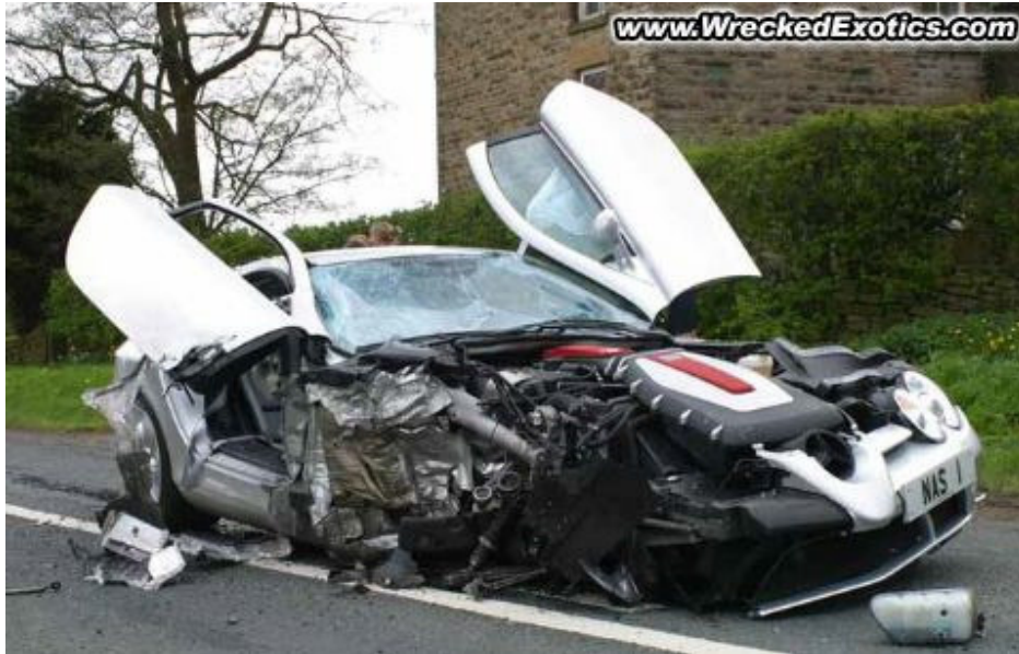
Figure 2-15. McLaren SLR following high speed front offset impact [55] (used with permission).
