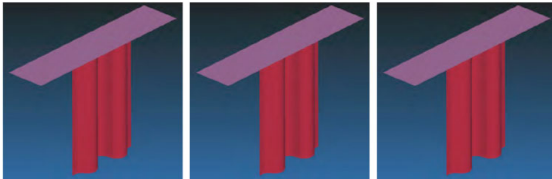
a. Progressive crushing.
