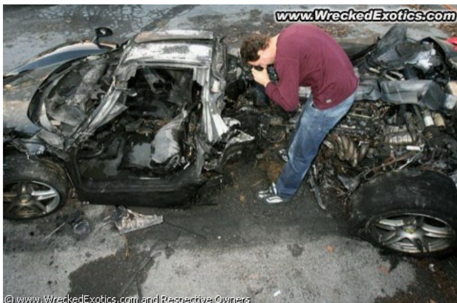
Figure 2-9. Ferrari Enzo “loosely re-assembled” after side impact [49] (used with permission).
