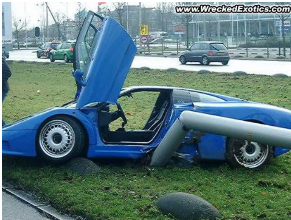
Figure 2-7. Bugatti EB110 following side impact [47] (used with permission).
