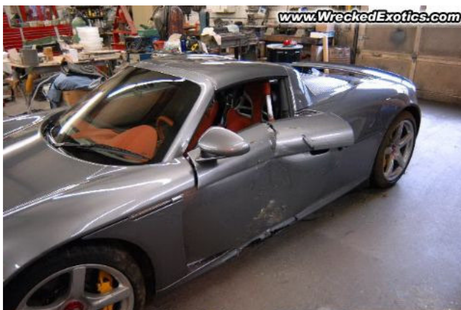
Figure 2-4. Porsche Carrera GT following side impact [44] (used with permission).
