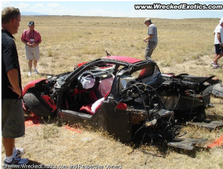
Figure 2-12. Ferrari Enzo following multiple flips and rollovers [52] (used with permission).
