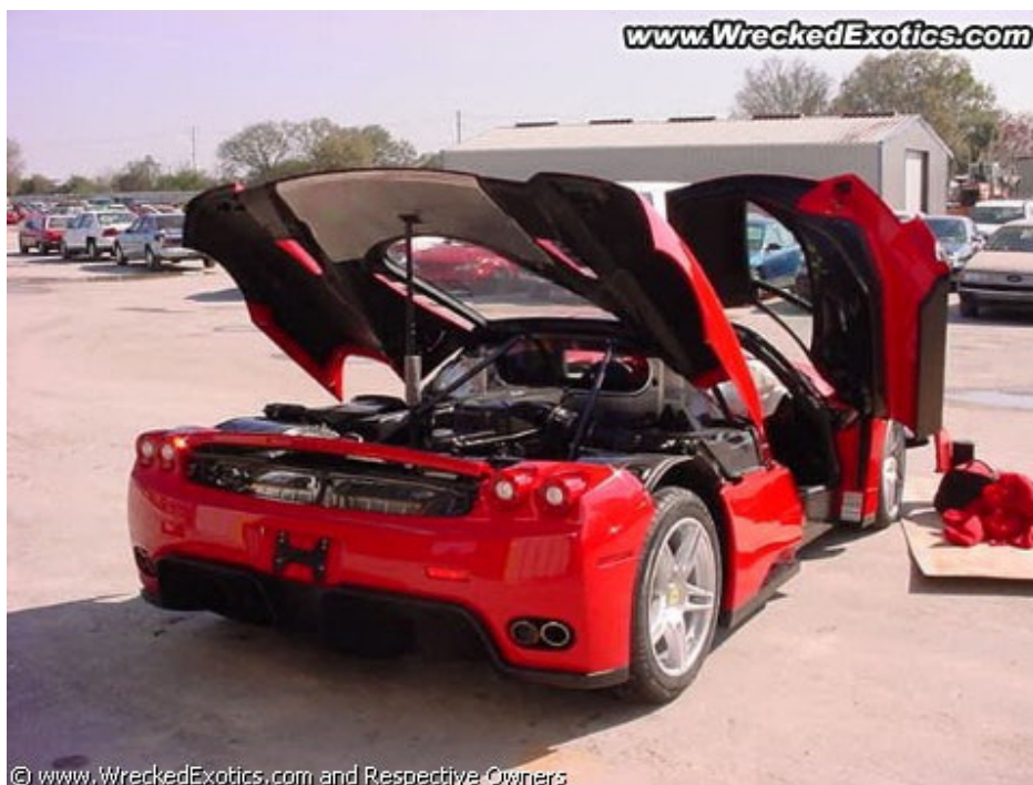
Figure 2-11. Ferrari Enzo following frontal impact. Note functioning closures [51] (used with permission).
