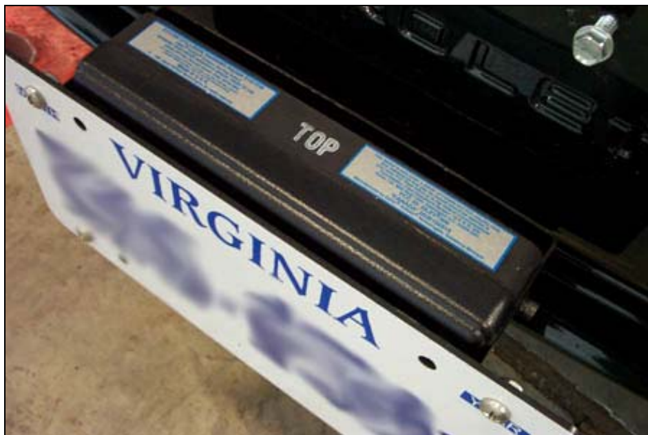
Figure 12. Doppler Radar Antenna Mounted on the Front of a Vehicle
