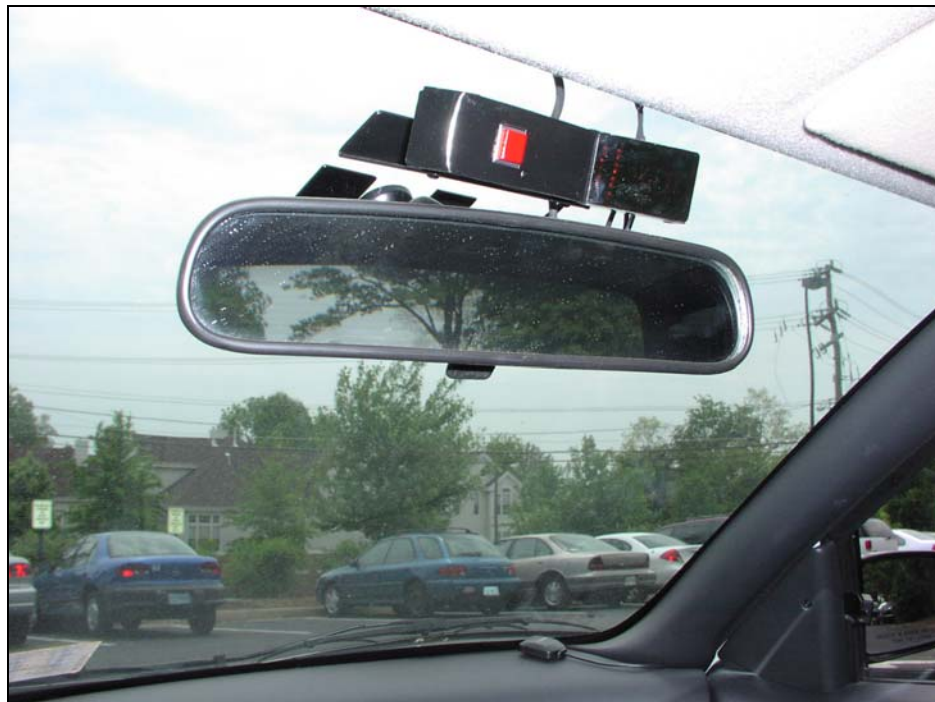
Figure 13. The Incident Push Button and Camera Box Mounted Above the Rearview Mirror
