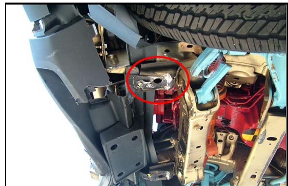
Figure 13. The post-test picture showing the deformed PEAS and SEAS
