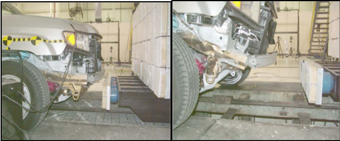
Figure 8. The pre and post-test pictures of the ORB with the align PEAS and deformed PEAS- SEAS respectively.
