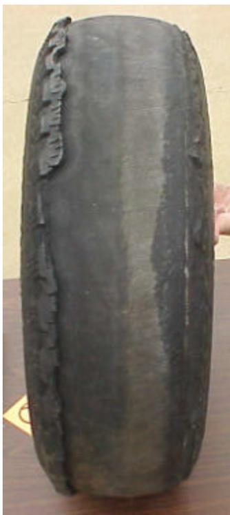
**Figure 10 – Separation pattern on the tire carcass of a failed Wilson P235/75R15 Wilderness AT tire, manufactured in Sep 96 (W2 396).**
