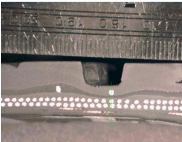
**Figure 29 – Pinched inter-belt gauge under tread groove, Joliette P235/75R15 Wilderness AT tire, manufactured in Nov 97 (VN 457).**
