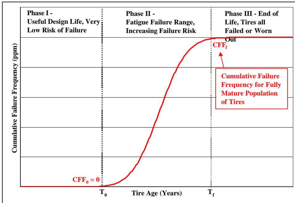
**Figure 12 – Fatigue failure theoretical model.**
