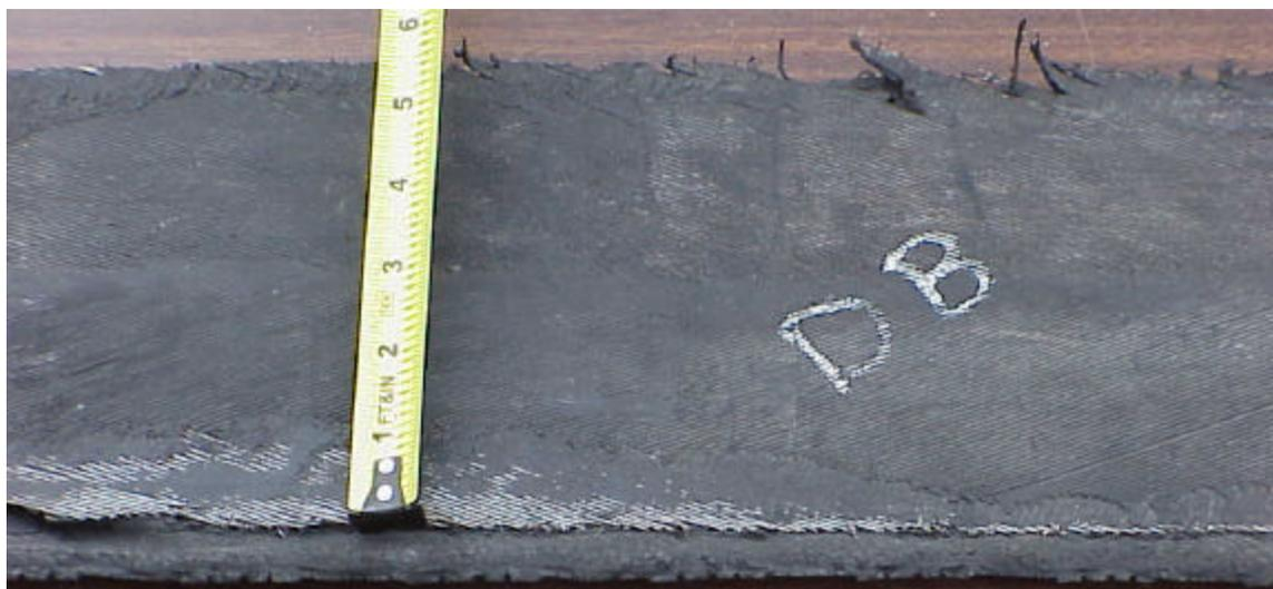
**Figure 11 – Separation pattern on the tread of the same failed Wilderness AT tire.**
