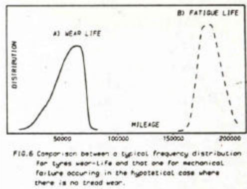
“Curve A represents the frequency distribution for the tyre’s wear life in its various uses. Curve B represents product life distribution for mechanical failure occurring in the hypothetical case where there is no tread wear.
