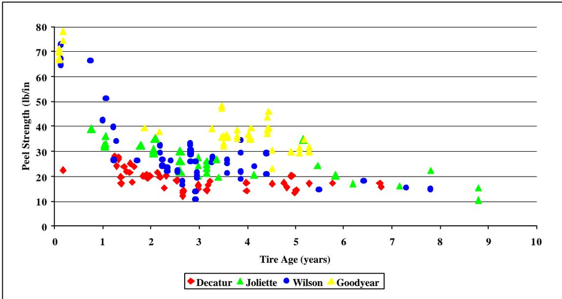
**Figure 40 – Hot state peel adhesion vs. age; Firestone tires (recalled and focus tires, ATX and Wilderness AT by plant) and Goodyear Wrangler RT/S.**
