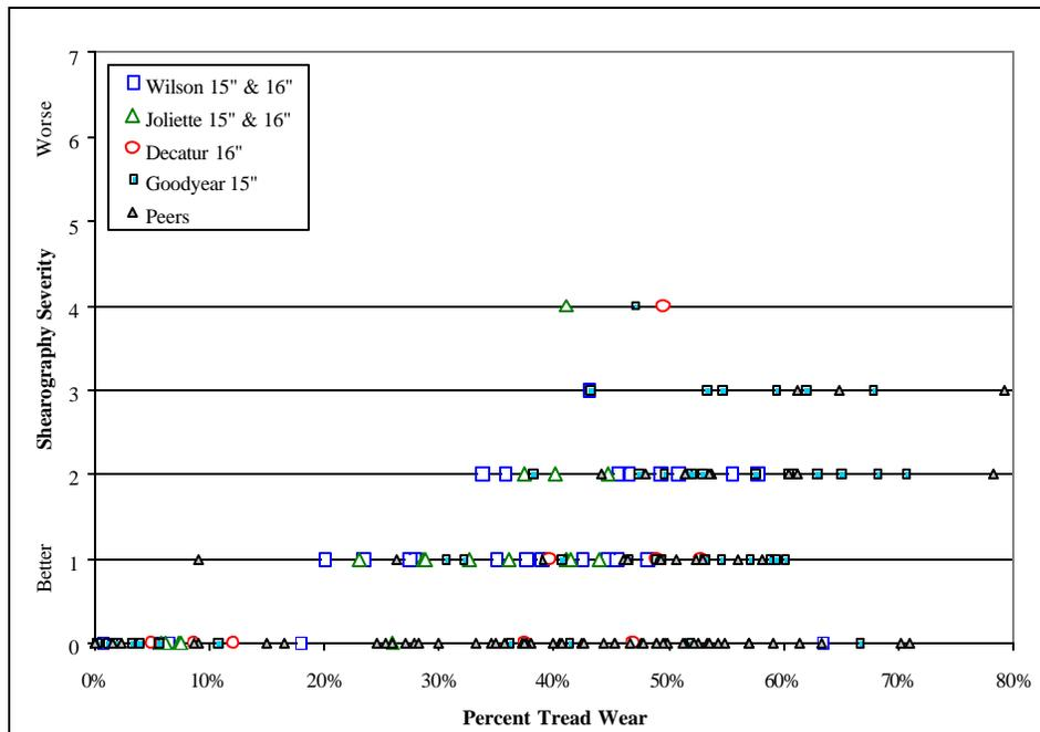
**Figure 24 – ODI shearography analysis comparing all post-wedge change focus tire to their peers by belt edge separation severity.**
