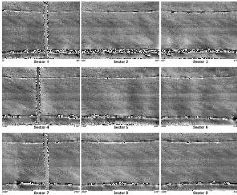
**Figure 32 – Shearography showing more advanced belt-edge separations, Wilson P255/70R16 Wilderness AT tire, manufactured in Apr 98 (W2 148).**
