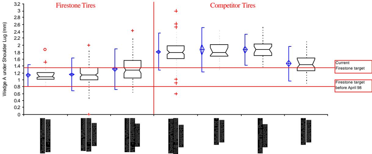
**Figure 25 – Wedge gauge under shoulder lugs, Focus tires (prior to 1998 design change) vs. peers.**
