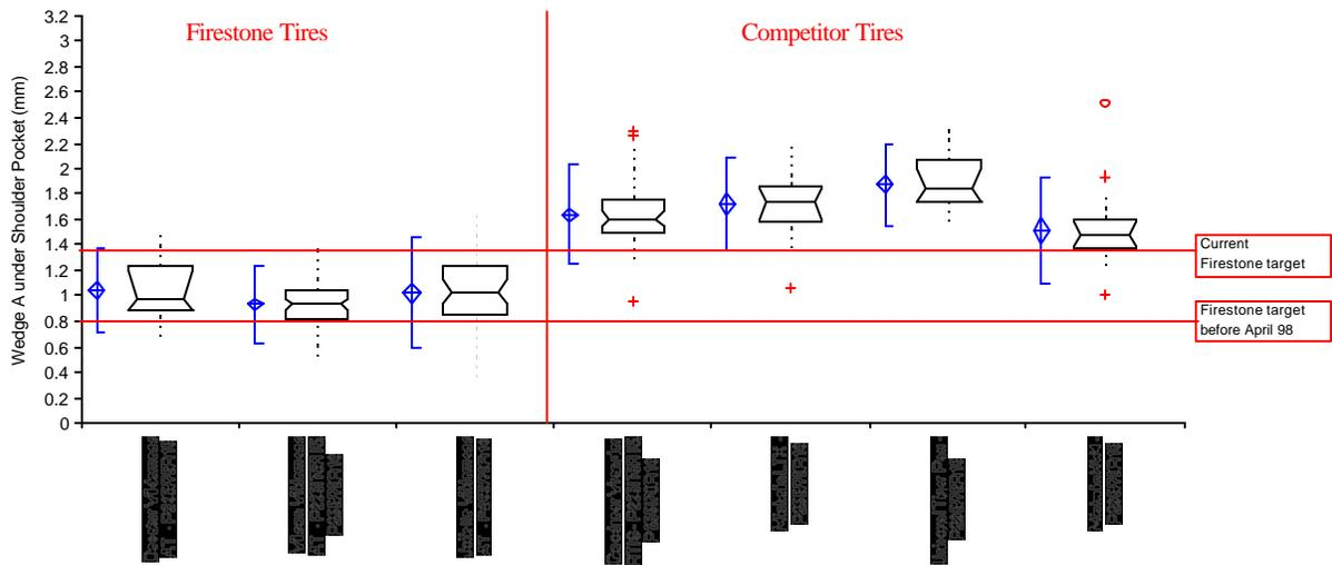
**Figure 35 – Wedge gauge under shoulder pocket, Focus tires (prior to 1998 design change) vs peers.**
