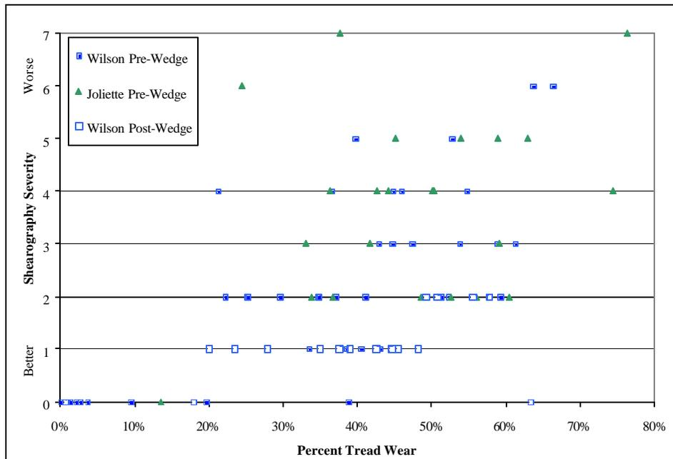
**Figure 22 – ODI shearography analysis comparing P235/75R15 pre- and post-wedge change focus tires by belt edge separation severity.**
