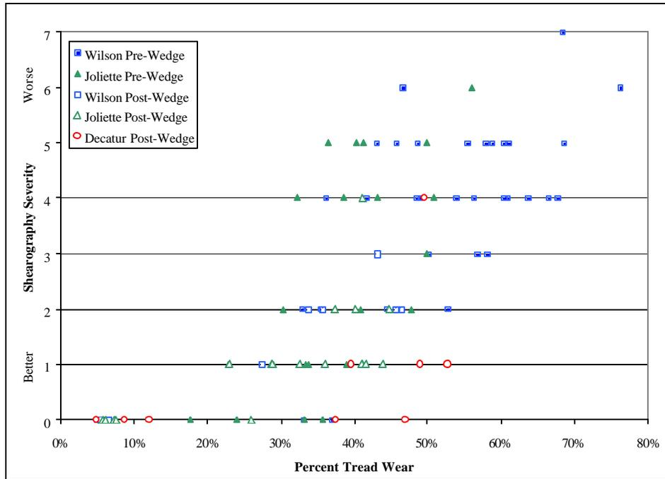
**Figure 23 – ODI shearography analysis comparing P255/70R16 pre- and post-wedge change focus tires by belt edge separation severity.**
