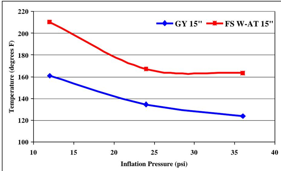
**Figure 41 - Tire operating temperature, P235/75R15 tires Firestone Focus vs. Goodyear Wrangler RT/S (Ford probe testing).**
