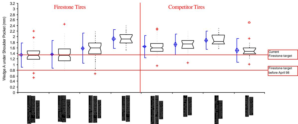
**Figure 36 – Wedge gauge under shoulder pocket, Focus tires (after the 1998 design change) vs peers.**
