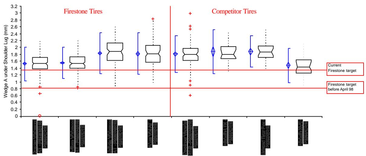
**Figure 26 – Wedge gauge under shoulder lugs, Focus tires (after 1998 design change) vs. peers.**
