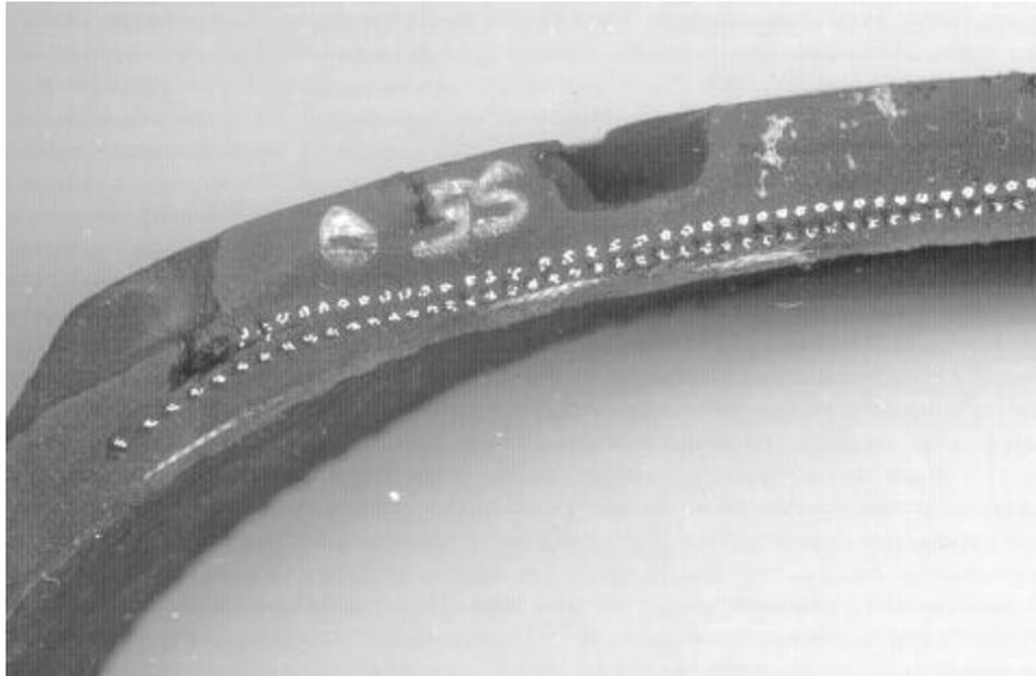
**Figure 20 – Wilderness AT pocket crack growth to edge of No. 2 belt
