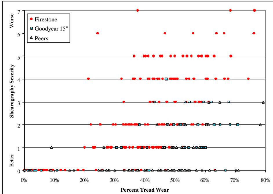
**Figure 21 – ODI shearography analysis comparing Firestone focus tires and their Goodyear and non-Goodyear peers by belt edge separation severity.**
