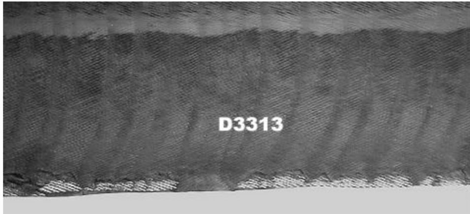
**Figure 38 – Tread-pull from test program tire with belt edge separation;
