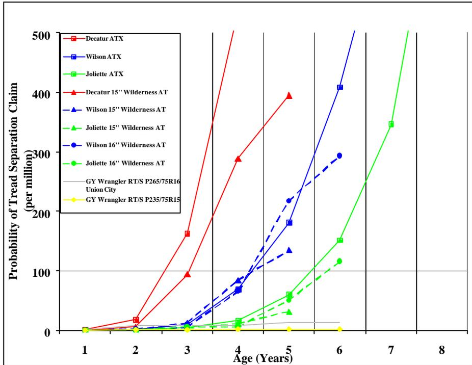
**Figure 19 – Cumulative hazard function, recalled tires, with focus tires, and two peer tires.**
