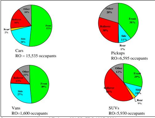
FIGURE 2: Seriously Injured Non-Fatal Rollover Occupants by Vehicle Type
