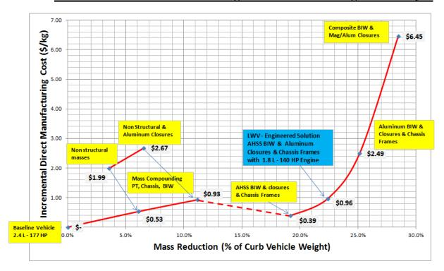
Figure 3-34 Mass Reduction Cost with Allowance for Powertrain Downsizing
