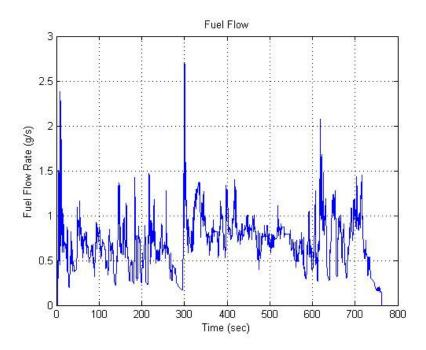
Figure 5-16 Fuel Flow Trace during FTP Cycle with Start-Stop
