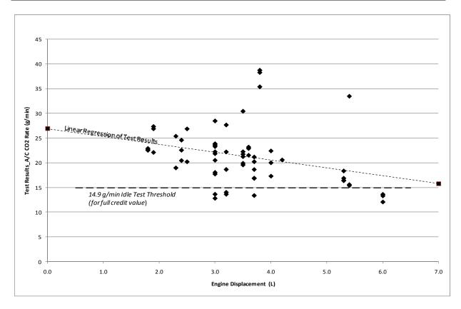
Figure 5-4 Relationship Between EPA A/C Idle Test Results and Engine Displacement.
