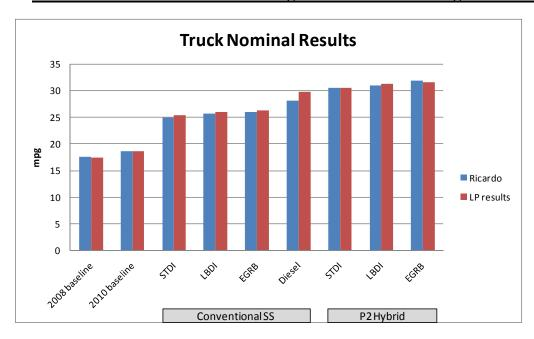
Figure 3-19: Comparison of LP to simulation results for Truck class
