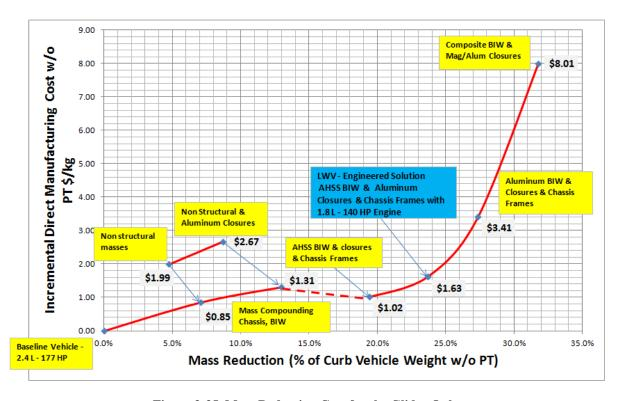
Figure 3-35. Mass Reduction Cost for the Glider Only
