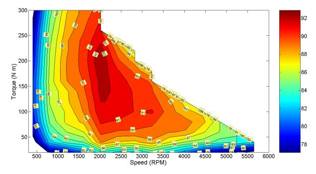
Figure 3-5: 2007 Camry Hybrid motor-inverter efficiency map (Burress, et al, 2008<sup>34</sup>)
