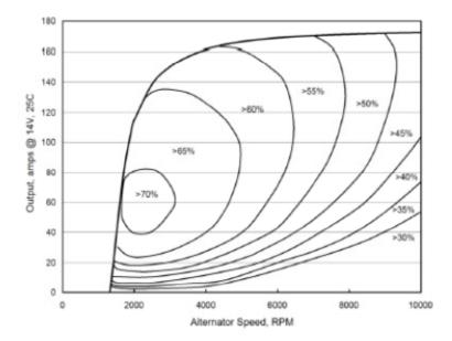
Figure 5-9: Alternator efficiency map (Delco-Remy, 2008<sup>40</sup>)
