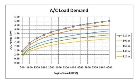
Figure 5-2 Representative A/C Compressor Load Curves
