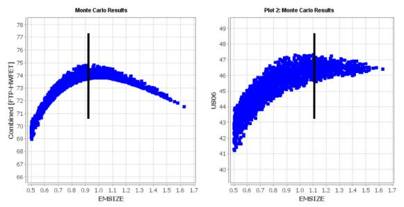
Figure 3-9: Electric motor sweeps for Standard Car class, P2 hybrid with stoichiometric GDI engine (left = FTP/HWFE test; right = US06 test)
