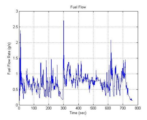
Figure 5-15 Fuel Flow Trace during Highway Cycle without Start-Stop
