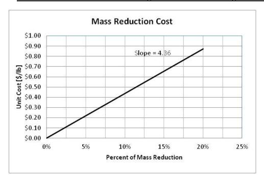
Figure 3-33 NPRM and FRM Mass Reduction Direct Manufacturing Cost
