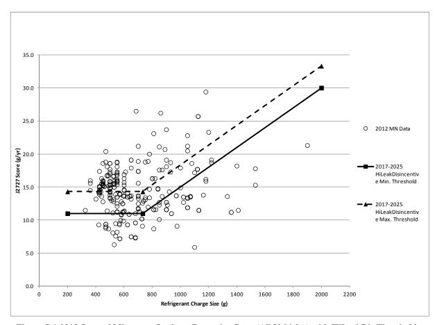
Figure 5-1 2012 State of Minnesota Leakage Reporting Data (All Vehicles) with HiLeakDis Thresholds
