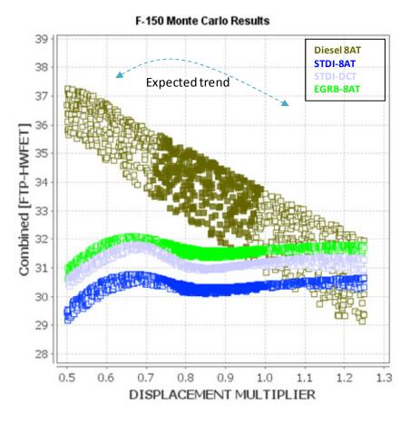
Figure 3-10: Example displacement sweep for Truck class in complex systems tool
