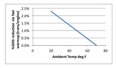
Figure 5-18 Relationship showing linear decay of GHG improvement as a function of ambient temperature.
