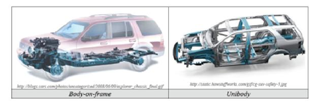
Figure 3-31 Illustration of Body-on-Frame (BoF) and Unibody vehicle construction
