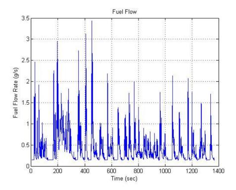
Figure 5-13 Fuel Flow Trace during FTP Cycle without Start-Stop
