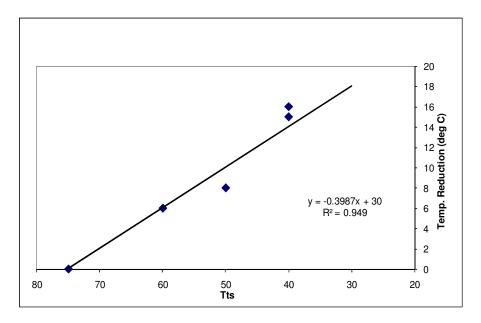
Figure 5-20 Correlation between Tts and Estimated Interior Temperature Reduction
