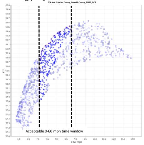
Figure 3-8: "Efficient Frontier" function in complex systems tool
