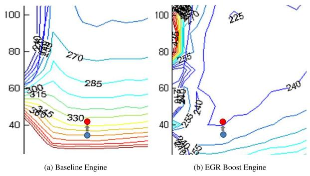
Figure 5-3 Average Engine Operating Conditions with A/C Off and A/C On over Fueling Maps for Baseline and EGR Boost Engines
