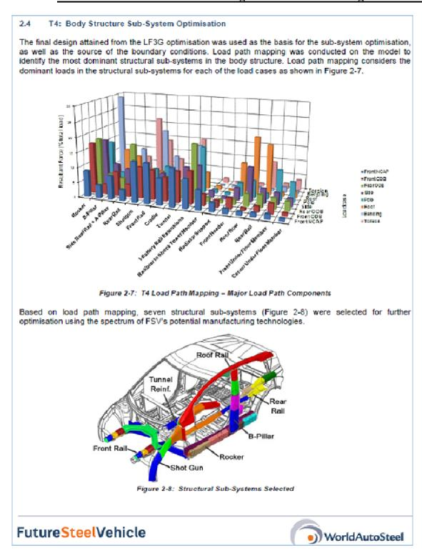
Figure 3-32 Example of vehicle body load path mapping for mass optimization
