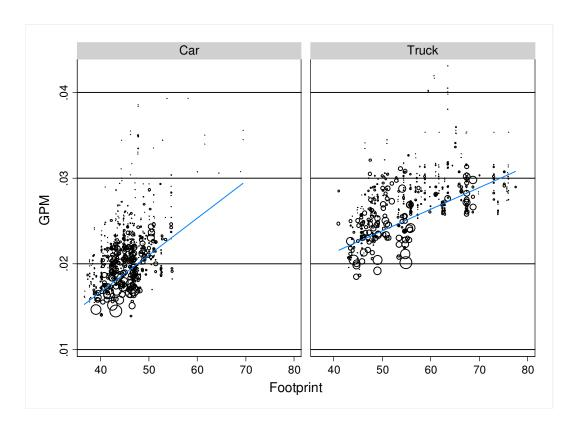
Figure 2-8 HP/WT Adjusted Fuel Consumption v. Footprint
