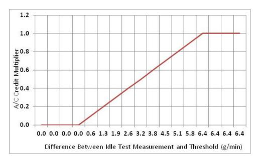
Figure 5-6 EPA A/C Credit Multiplier as a Function of the Difference Between Idle Test Measured and Threshold at any given engine displacement
