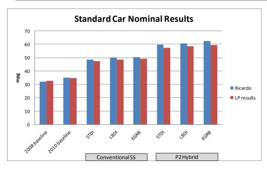
Figure 3-15: Comparison of LP to simulation results for Standard Car class
