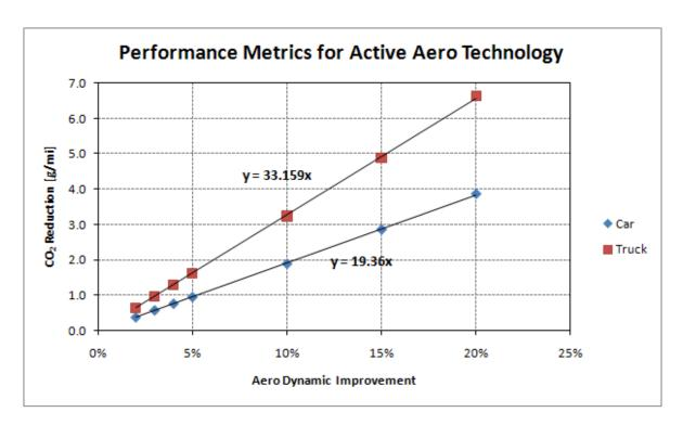
Figure 5-11 Simulated GHG Reduction Benefits of Active Aerodynamic Improvements
