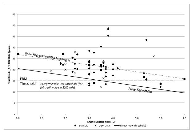
Figure 5-5 EPA A/C Idle Test Results with Results from Various Manufacturers
