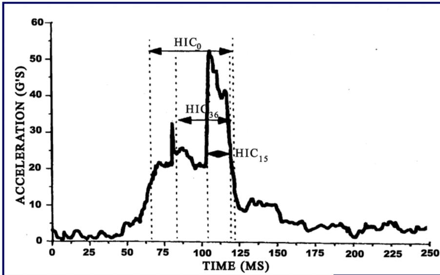
$$HIC = \max \left[ \frac{1}{t_2 - t_1} \int_{t_1}^{t_2} a(t) dt \right]^{2.5} (t_2 - t_1)$$
