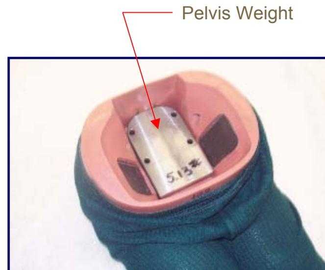
Fig. 2. Location and shape of pelvis weight
