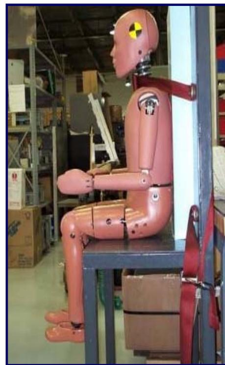
The 10-Year-Old Hybrid III Dummy First Prototype
