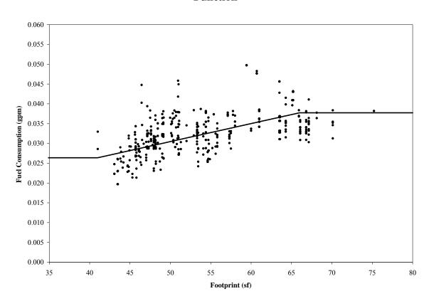
Figure V-5 "Maximum Technology" Light Truck with Fitted Constrained Linear Function
