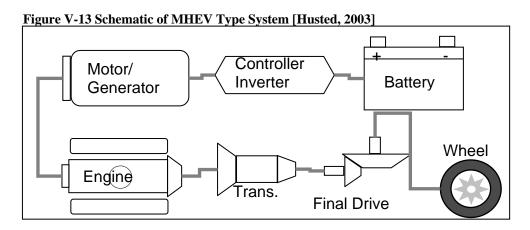
Higher Voltage Stop-Start/Belt Integrated Starter Generator (BISG)
