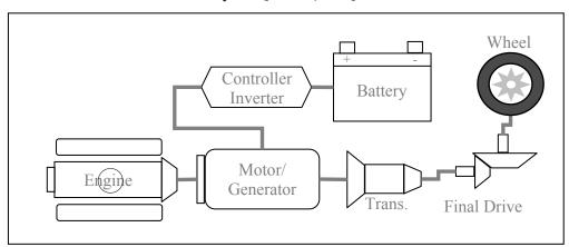
Figure V-14 Schematic of Honda IMA System [Husted, 2003]
