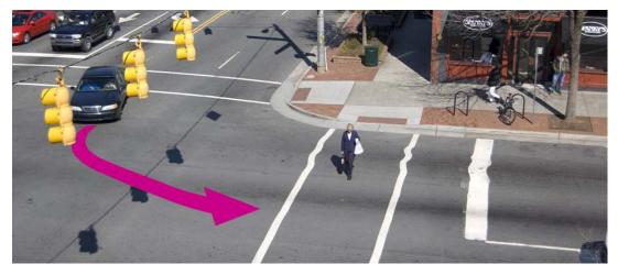
Here, the pedestrian and the driver of the left-turning vehicle both have traffic signals telling them it is their turn.
