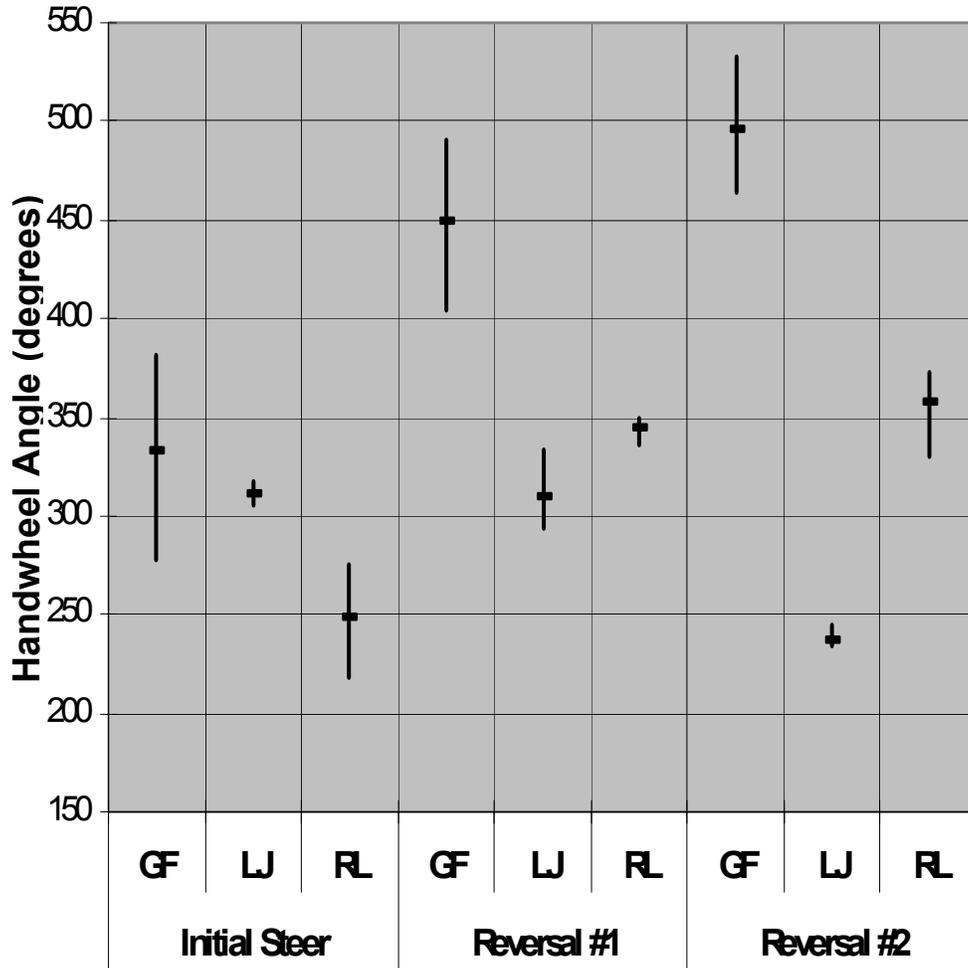
Figure 15: Handwheel input repeatability observed during Consumers Union Short Course Double Lane Change testing performed with the Chevrolet Blazer
