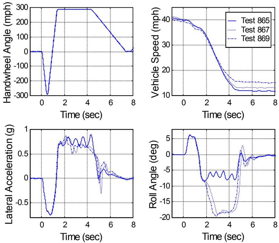
**Figure 8: Roll Rate Feedback Fishhook test inputs and outputs for three tests performed with the Toyota 4Runner with vaw stability control disabled**
