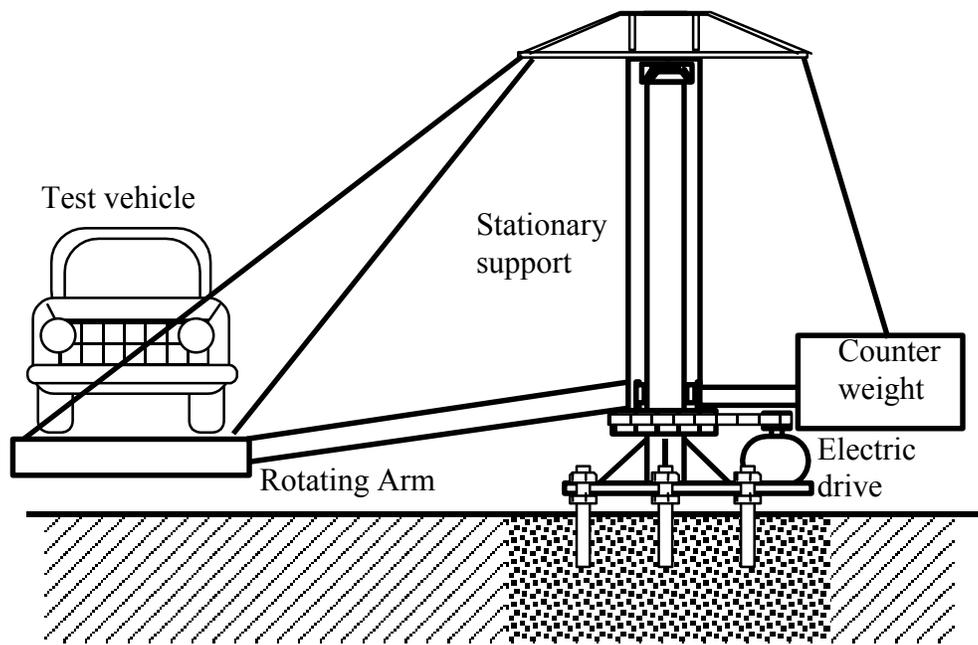
**Figure 3. Centrifuge Test**
