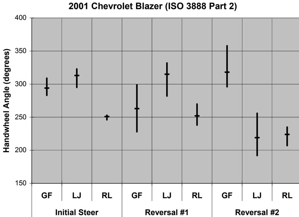
**Figure 12: Handwheel input repeatability observed during ISO 3888 Part 2 Double Lane Change testing performed with the Chevrolet Blazer**
