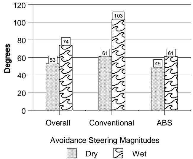
**Figure 4.** Magnitude of avoidance steering inputs.
