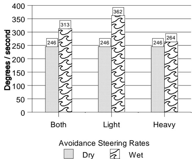
**Figure 8.** Avoidance steering rates by brake pedal feedback.
