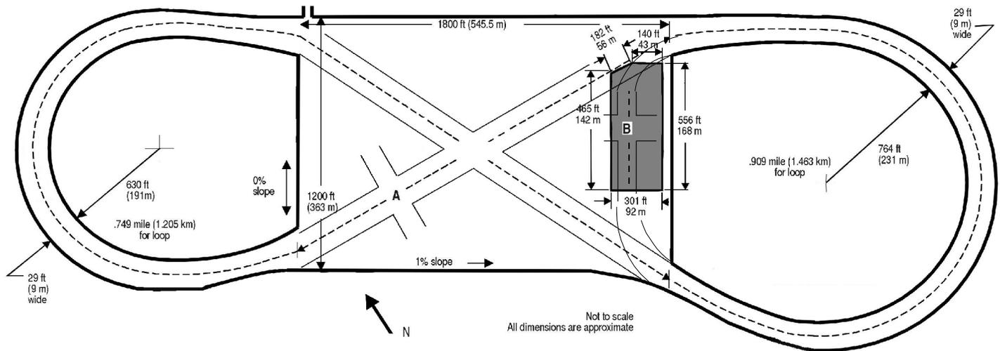
**Figure 1.** Illustration of location and layout of course used in the dry and wet pavement intersection incursion studies.
