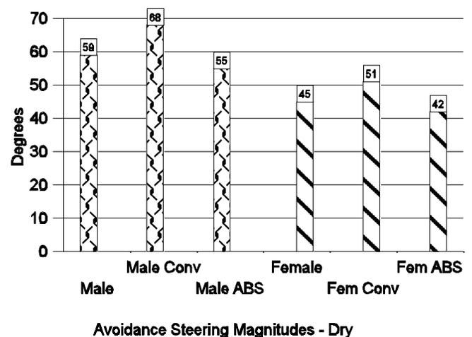
**Figure 10.** Magnitude of the avoidance steering input by gender and brake system - dry study.
