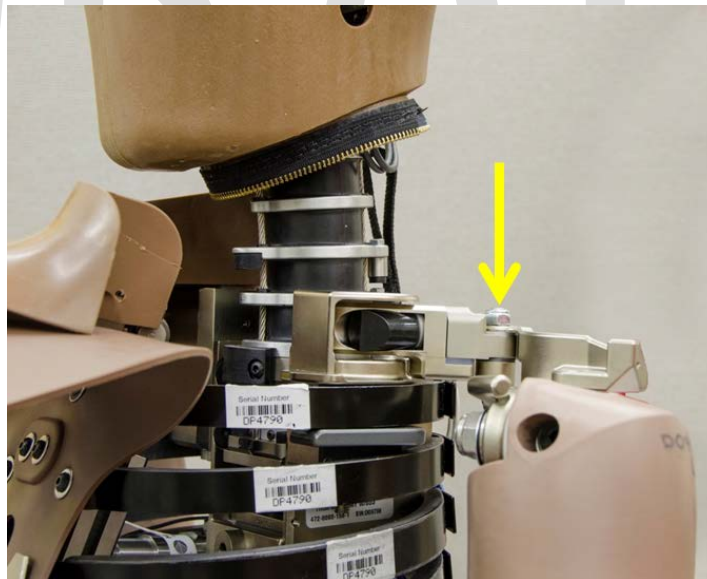
Figure 3-11. Locknut on joint connecting shoulder support assembly to arm link.
