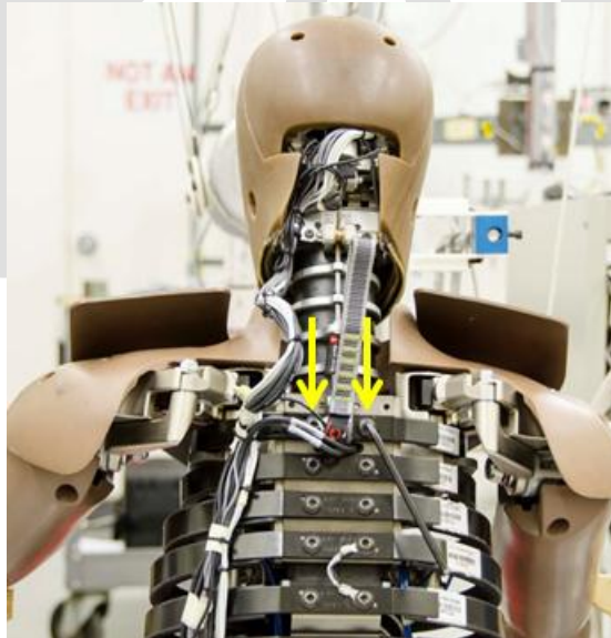
Figure 6-13. Two posterior bolts attaching rib #1 to the spine
