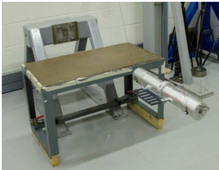
Figure 10-2. Seat setup for upper leg qualification test
