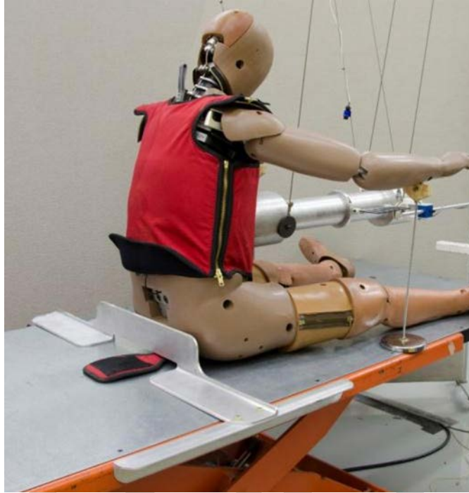
Figure 8-4. Alignment of the frontal plane perpendicular to the impact direction using a right-angled guide.
