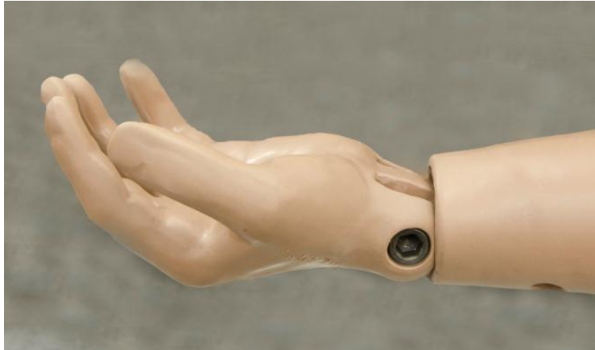
Figure 3-7. Wrist orientation for setting joint torque to 1G
