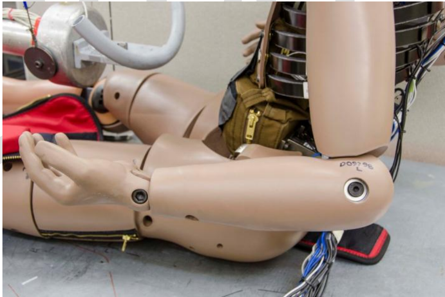
Figure 3-8. Elbow orientation for setting joint torque to 1G
