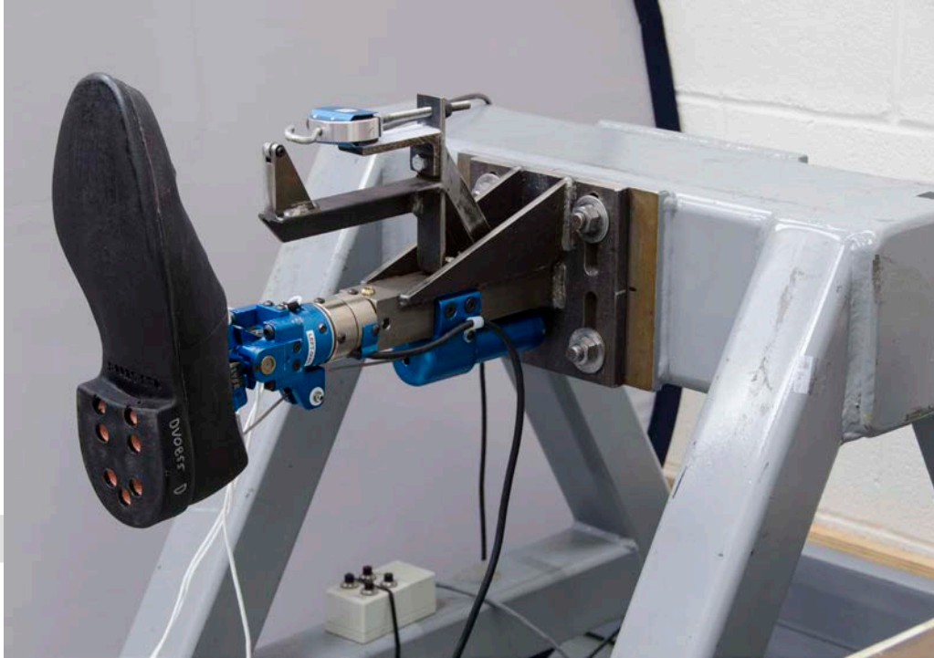
Figure 3-24. Lower leg assembled to Achilles fixture
