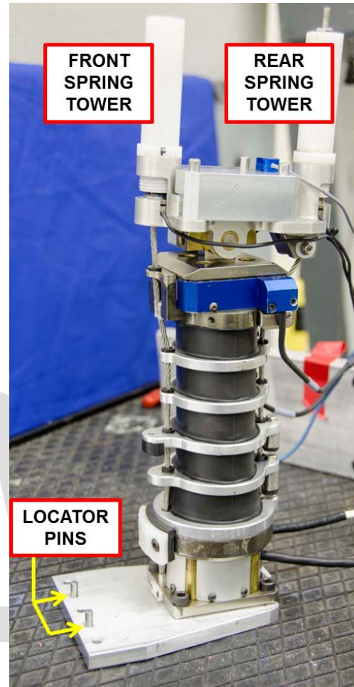
Figure 6-27. Orientation of neck relative to locator pins
