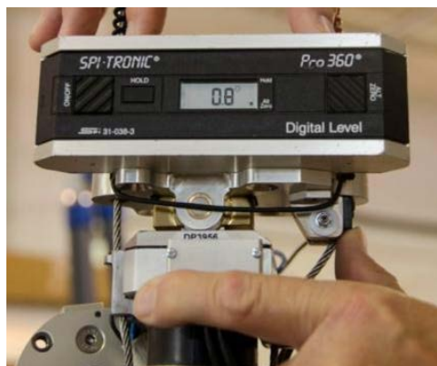
Figure 6-4. Inclinometer placement on top surface of neck mounting platform ( NeckMountPlatform ®)
