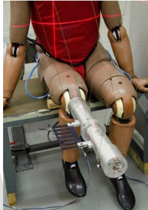
Figure 10-7. Lateral alignment of impact location
