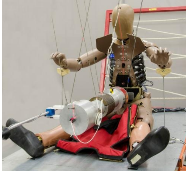
Figure 9-3. Lateral alignment of impact location
