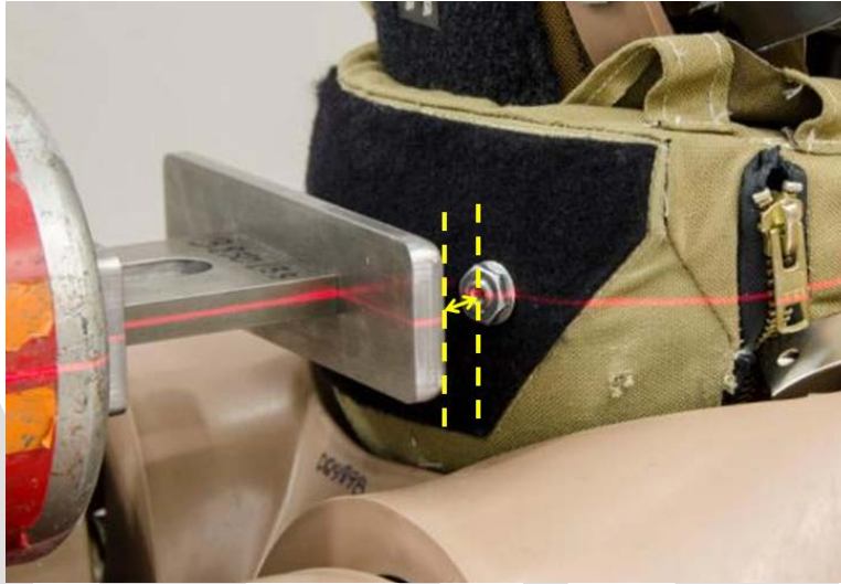
Figure 9-6. Measurement of distance from IR-TRACC attachment nuts to impactor
