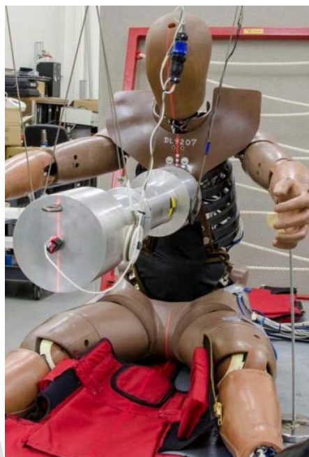
Figure 7-3. Lateral alignment of impact location
