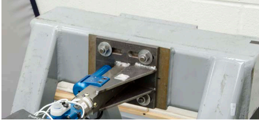
Figure 12-4. Orientation of lower leg mounting bracket for inversion tests
