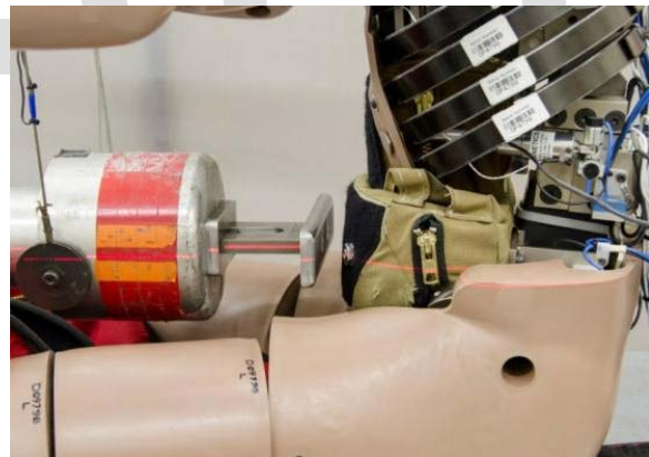
Figure 9-5. Vertical alignment of impact location
