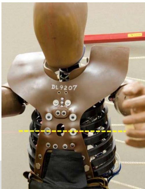
Figure 7-2. Vertical alignment of impact location
