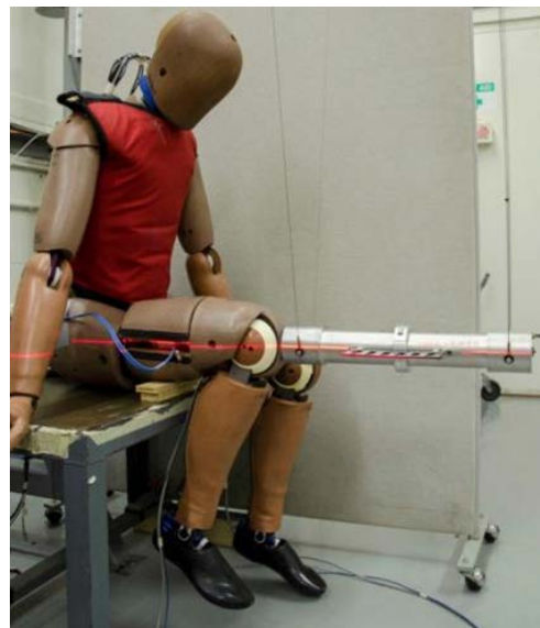
Figure 10-3. Initial setup for the upper leg qualification test
