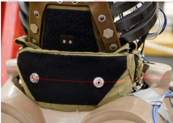
Figure 9-4. Horizontal alignment of IR-TRACC attachment nuts
