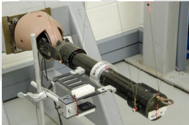
Figure 11-4. Lateral alignment of impact location
