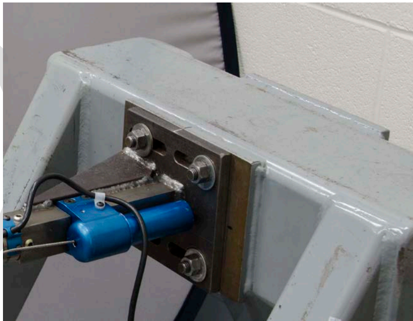
Figure 12-5. Orientation of lower leg mounting bracket for eversion tests
