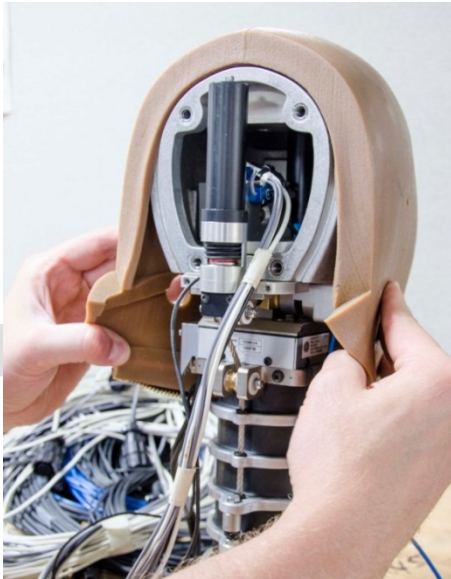
Figure 6-19. Separation of head skin from grooves at posterior of skull assembly
