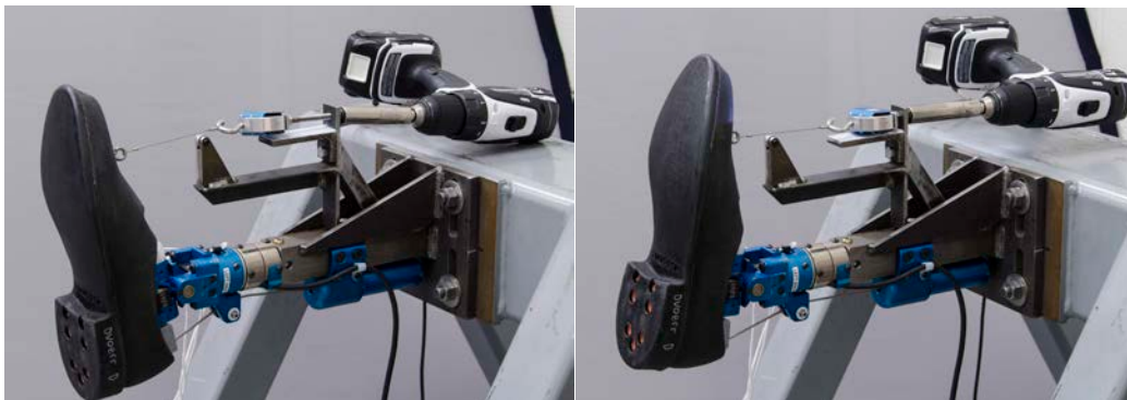
Figure 3-26. Collecting force and angle data to determine Achilles load
