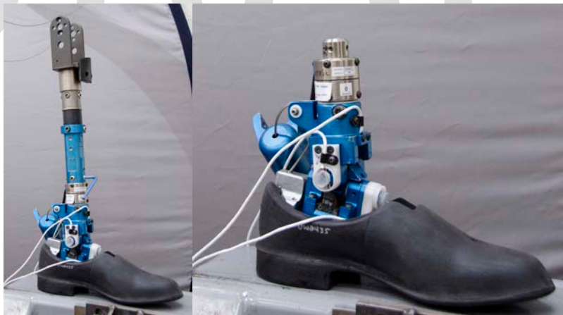
Figure 12-3. Separate the ankle assembly from the lower tibia load cell
