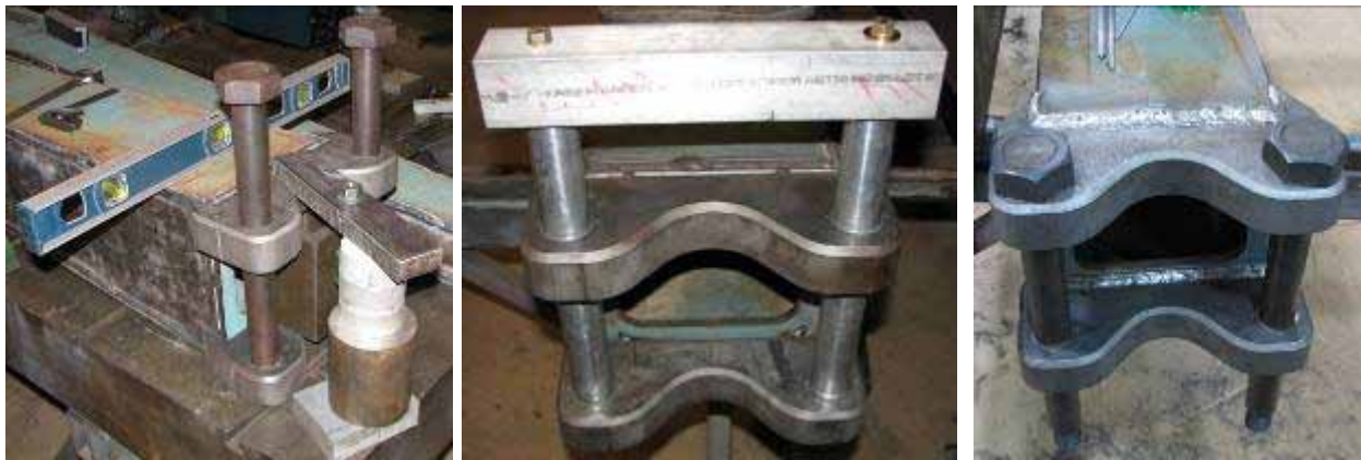
Figure 4.4: Left: clamping and jigging of Hinge Brackets. Middle: aluminum jig used to assure alignment. Welding was performed with jig in the holes. Right: finished Hinge Brackets with shoulder bolts in. The bolts should easily slide through holes when finished.
