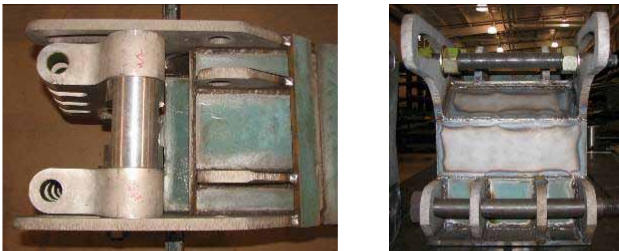
Figure 4.20: Left: 8 th and 9 th steps have been completed and jigging has been removed. Right: 12 th step has been completed; cover plates were welded in place. Note: Jigs holding the Lower Adjustment Brackets should be left in when welding is taking place on the Inboard Beam. Free play tolerances were lost when those jigs were removed and welding operations performed.
