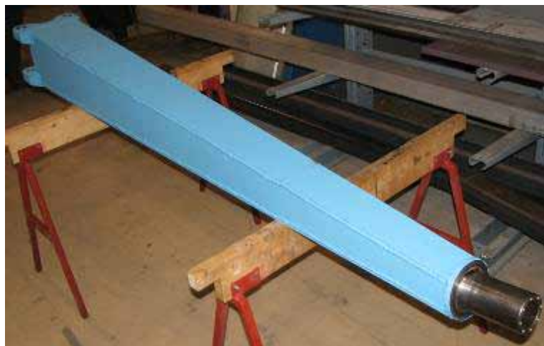
Figure 4.7: Finished welded and painted Outboard Beam.
