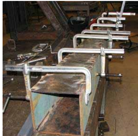
Figure 4.2: Pictures of the fabrication of the outboard beam. Clamps and 90° angle iron pieces are used to jig the plates that form the tapered beam (outer edges are aligned and tacked into place). All outside seams were continuously welded. Inner seams were welded according to what the welder could reach.
