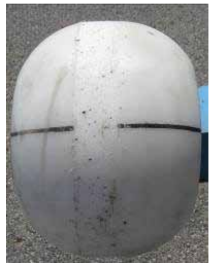
Figure 5.7: Wear after 14 strikes between wheel and test surface. Diameter change is estimated at \sim 1/32 inch or less.
