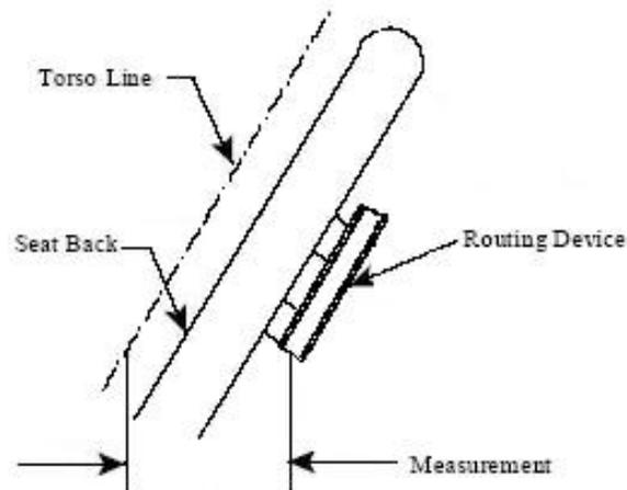
Figure 6 – Measurement of Tether Routing Device
