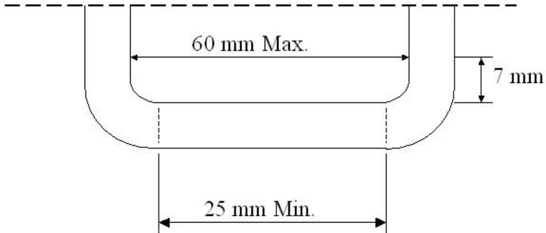
Figure 8 – Measurement of Lower Anchor Bar Length
