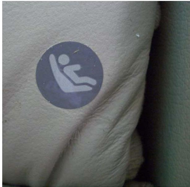
Figure 11 – Example of Lower Anchor Bar location marking
