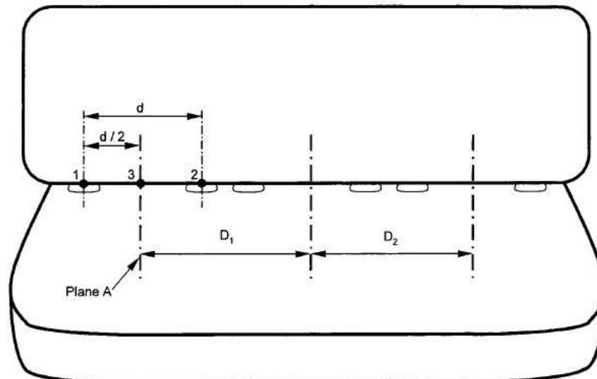
$d$  = center to center distance between lower anchorages for a given seating position (nominally 280 mm).
