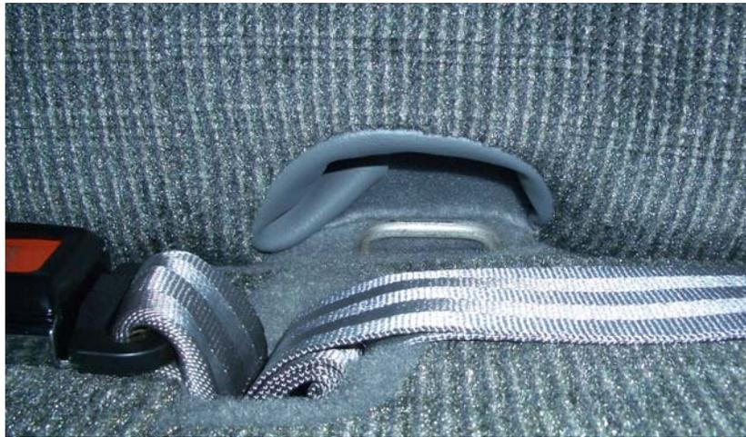
Figure 12 – Example of Lower Anchor Bar Visibility
