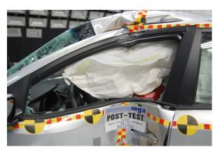
\_\_8 Test Dummy Shoulder and Door Top View
