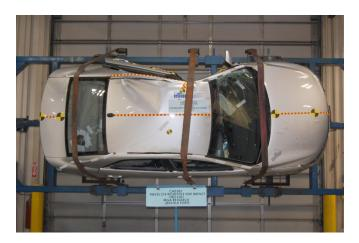
\_\_17 301 Static Rollover Test – 360 degree
