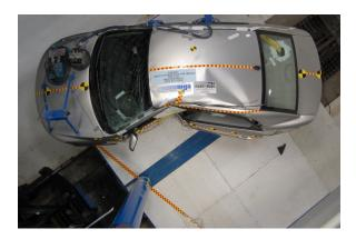
Test Dummy Through the Opposite Side Window \_\_6
