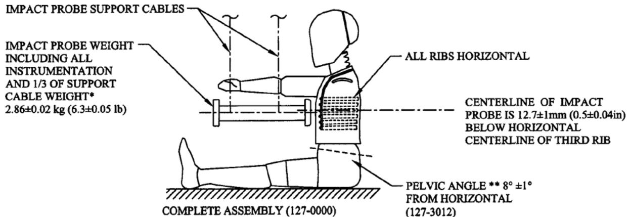
\* 1/3 CABLE WEIGHT NOT TO EXCEED 5% OF THE TOTAL IMPACT PROBE WEIGHT
