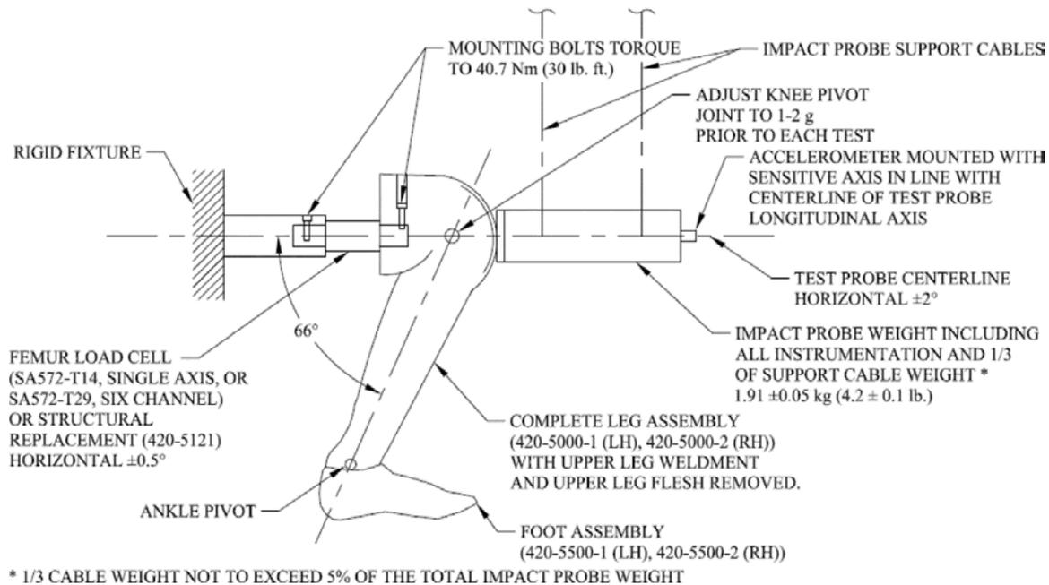
FIGURE 8. KNEE IMPACT TEST SET-UP SPECIFICATIONS
