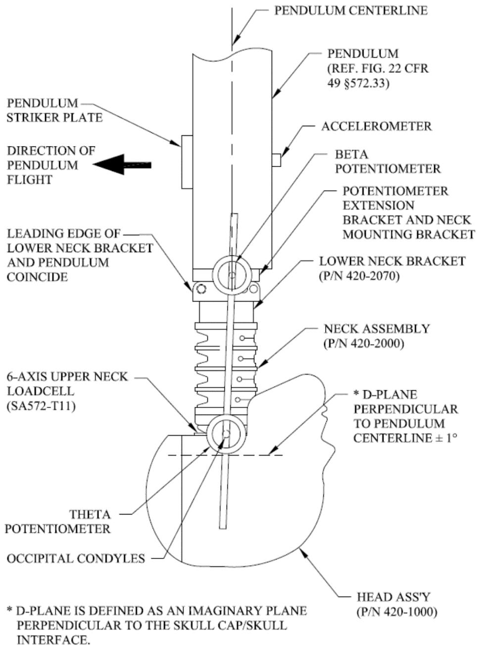
FIGURE 5. NECK EXTENSION TEST SET-UP SPECIFICATIONS
