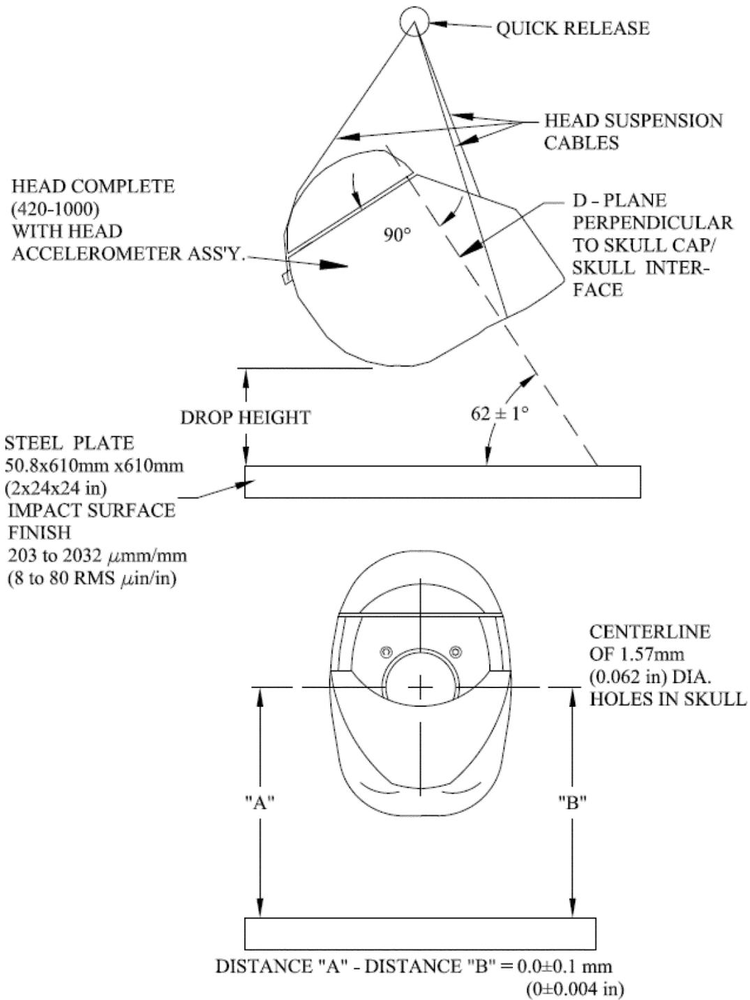
FIGURE 2. HEAD DROP TEST SET-UP SPECIFICATIONS
