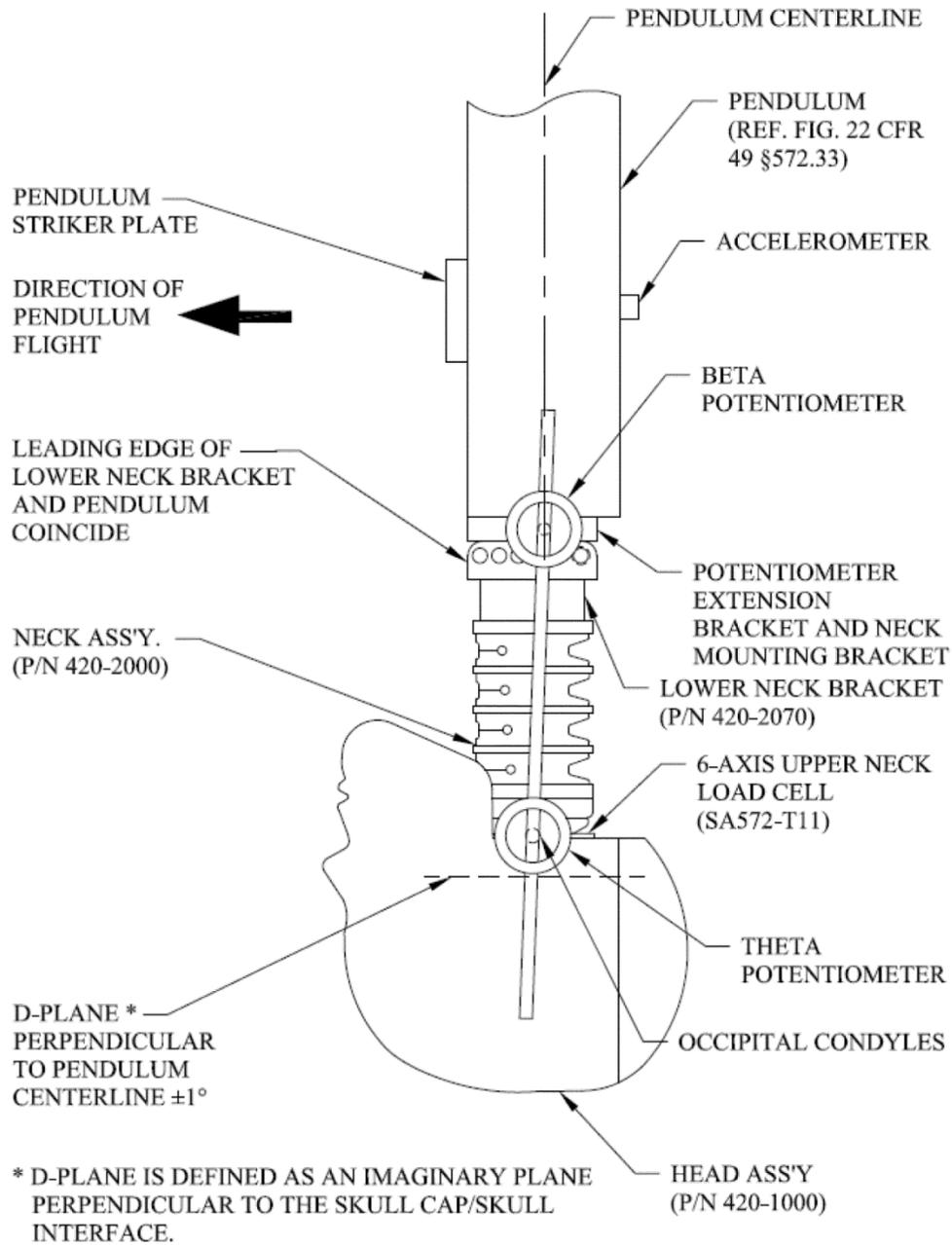
FIGURE 4. NECK FLEXION TEST SET-UP SPECIFICATIONS
