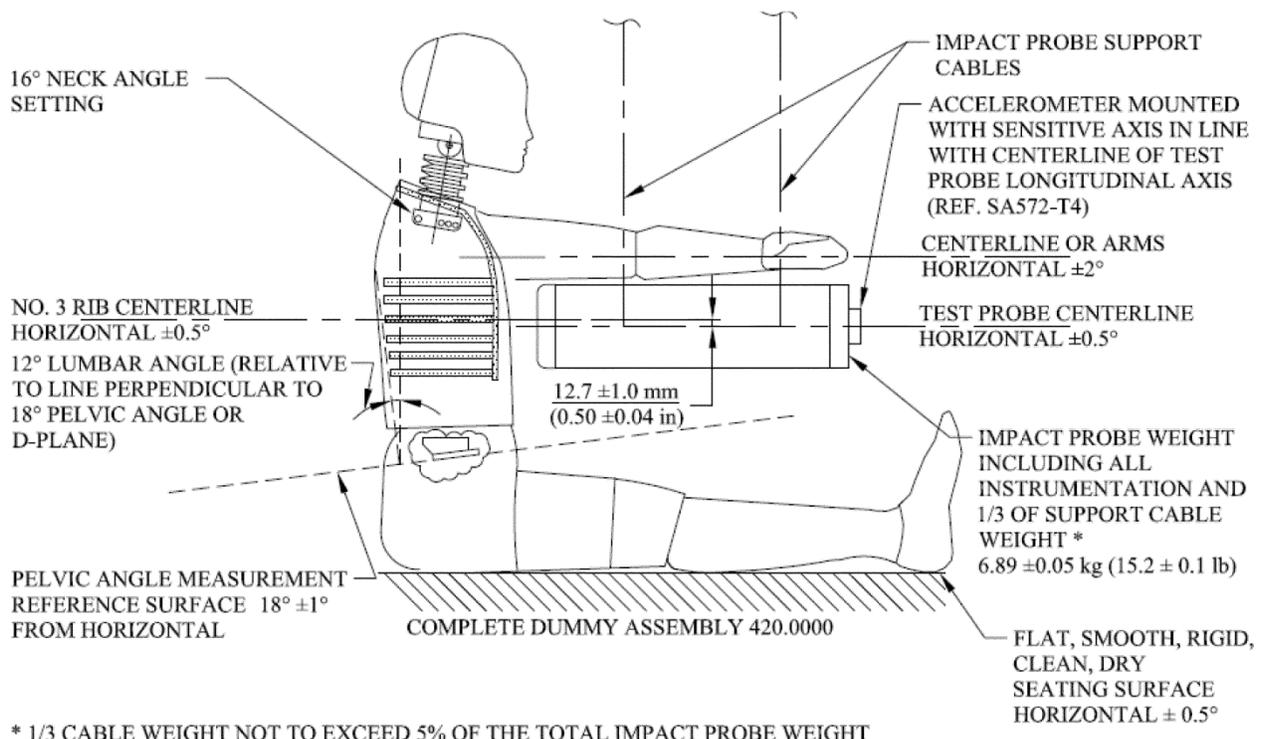
FIGURE 6. THORACIC IMPACT TEST SET-UP SPECIFICATIONS
