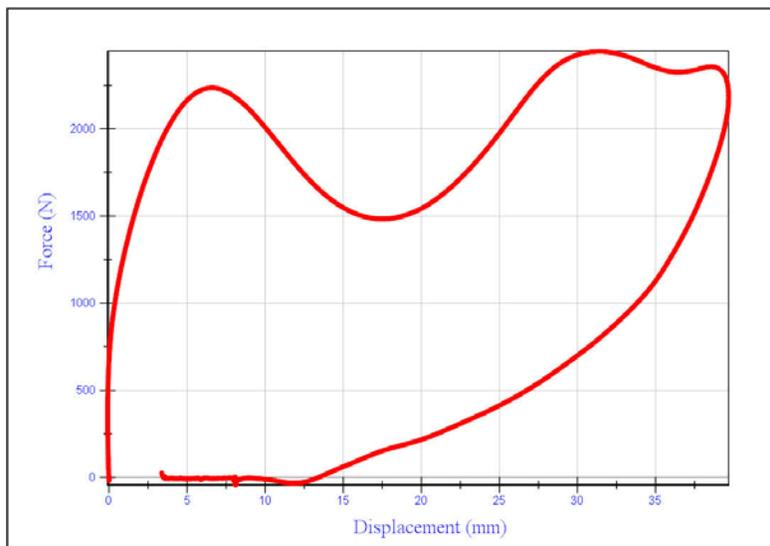
FIGURE 10. PART 572T HYBRID III-10C THORAX CALIBRATION – HYSTERESIS
