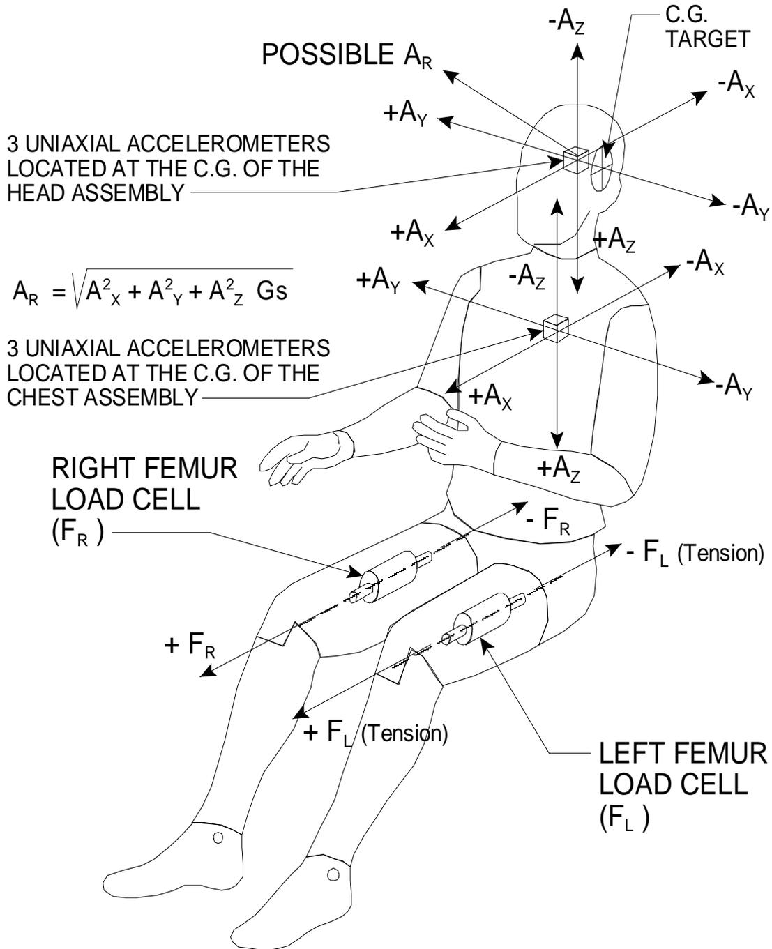
FIGURE 1. SIGN CONVENTION FOR PART 572 TEST DUMMIES
