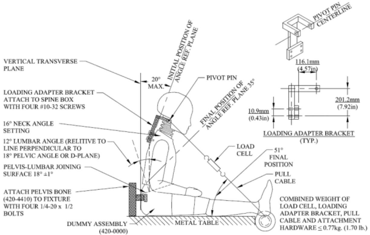
FIGURE 7. TORSO FLEXION TEST SET-UP SPECIFICATIONS
