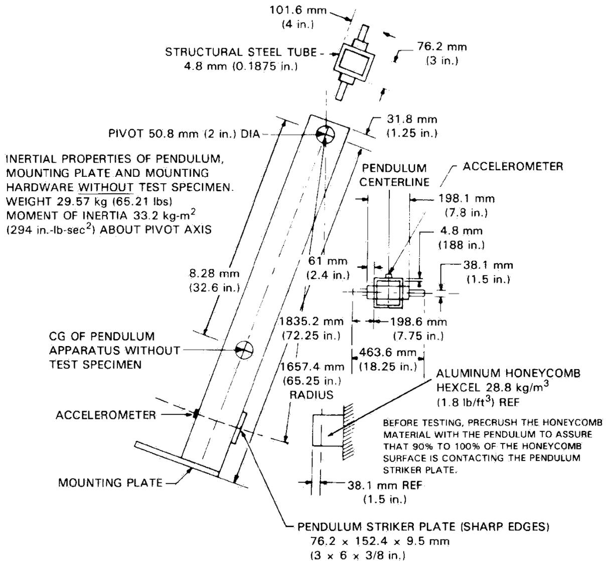
FIGURE 3. NECK PENDULUM SPECIFICATIONS
