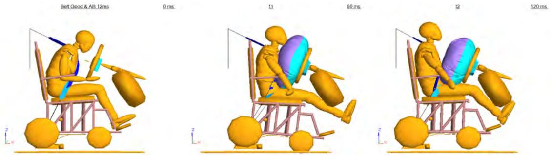
(a) - good belt fit with deployment of the steering-wheel air bag
