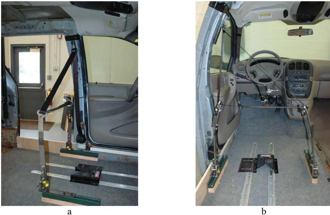
Figure 2.23 – Photos of a prototype of the pivoting-bar lap/shoulder belt restraint system installed in the static minivan buck
