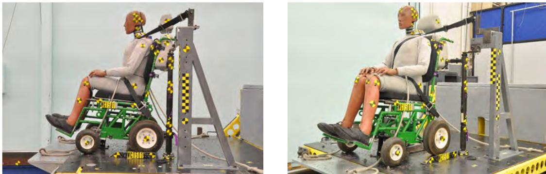
Figure 2.77 - Pre-test photos of the manufacturer' revised design of the Swedish deployable vehicle-anchored head-and-back restraint system
