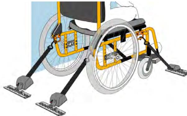
Illustration of a wheelchair secured by a four-point, strap-type tiedown
