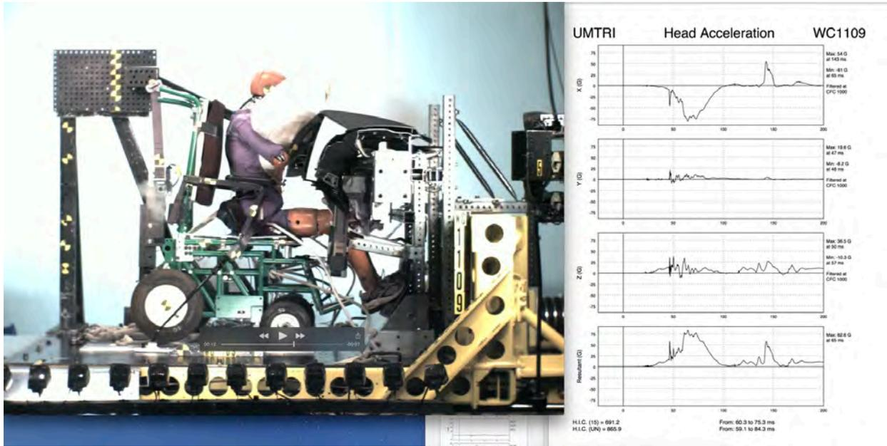
Figure 3.6 - Side-view photo at PEAK RESULTANT HEAD ACCELERATION from high-speed video for Test No. WC1109 with the small-female ATD restrained by a loosely fitting lap/shoulder belt and 42-ms an air-bag deployment time of 42 ms
