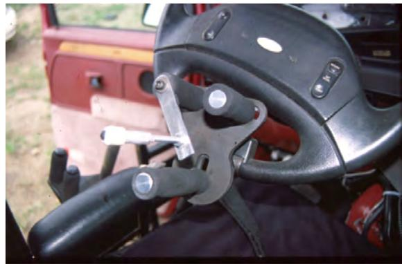
Tri-pin attached to lower steering-wheel rim
