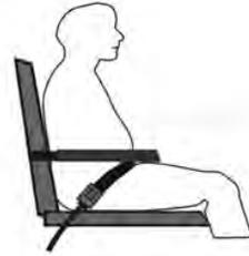
Proper positioning of a vehicle-anchored lap belt with wheelchair arm supports that are attached to the back-support posts and completely open at the front and underneath
