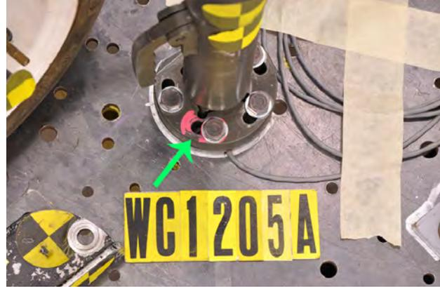
Figure 2.70 - Broken plastic drive nut (upper part of photo on left) on screw-motor actuator and slippage in curved slots at the base of the Swedish head-and-back restraint post (right) that were significant contributors to the poor performance of the Swedish deployable vehicle-anchored head-and-back restraint system in the second sled test
