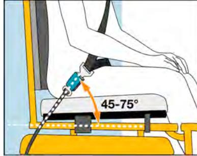
Buckle receptacle attached to rigid cable stalk to keep receptacle off floor and more accessible
