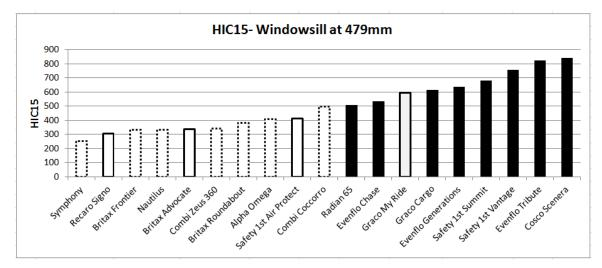
Figure 8 – HIC<sub>15</sub> outcome for each CRS design @ 479 mm (18.8 in) windowsill (solid outline=good design, dashed outline=average design, filled-in black=poor design)
