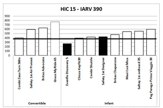
Figure 6 – HIC<sub>15</sub> Values in Tests with CRABI Dummy in Rear Facing CRSs (Solid Black Outline=good side coverage and padding, Dashed Black Outline=good side coverage or padding, Solid Black=poor side coverage and padding)
