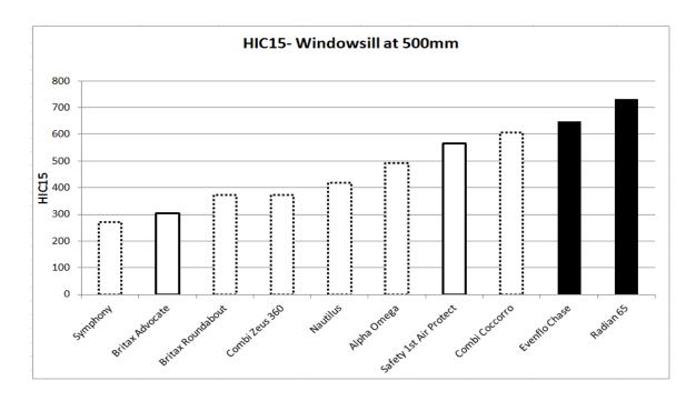
Figure 9 – HIC<sub>15</sub> outcome for each CRS design @ 500 mm (19.6 in) windowsill (solid outline=good design, dashed outline=average design, filled-in black=poor design)
