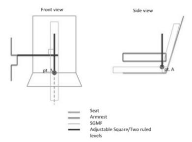
Figure 4 - Tool Placement when measuring lateral and vertical distance of armrest and windowsill to point A.
