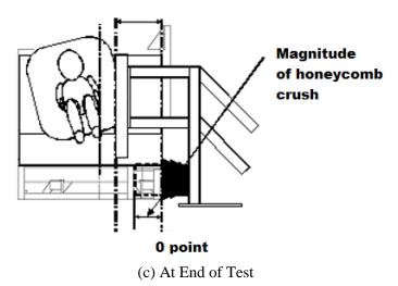
Figure 1 - Takata Side Impact Sled System--(a) Pre-test condition, (b) At time of door contact with CRS, (c) At end of test (final travel of door).
