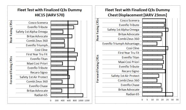
Figure 7 - Fleet Test Results: HIC<sub>15</sub> (left) and Chest Displacement (right)
