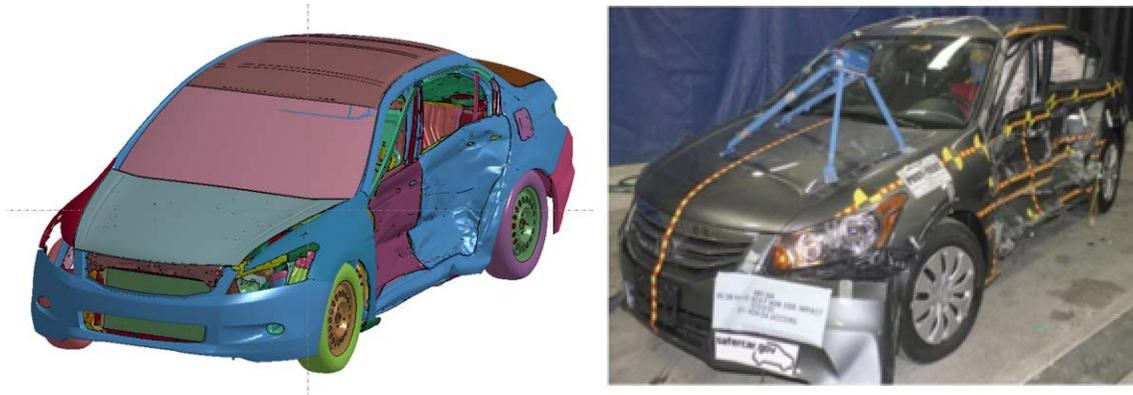
**Figure 49: Model and Test #7098 Lateral NCAP MDB Post Test**
