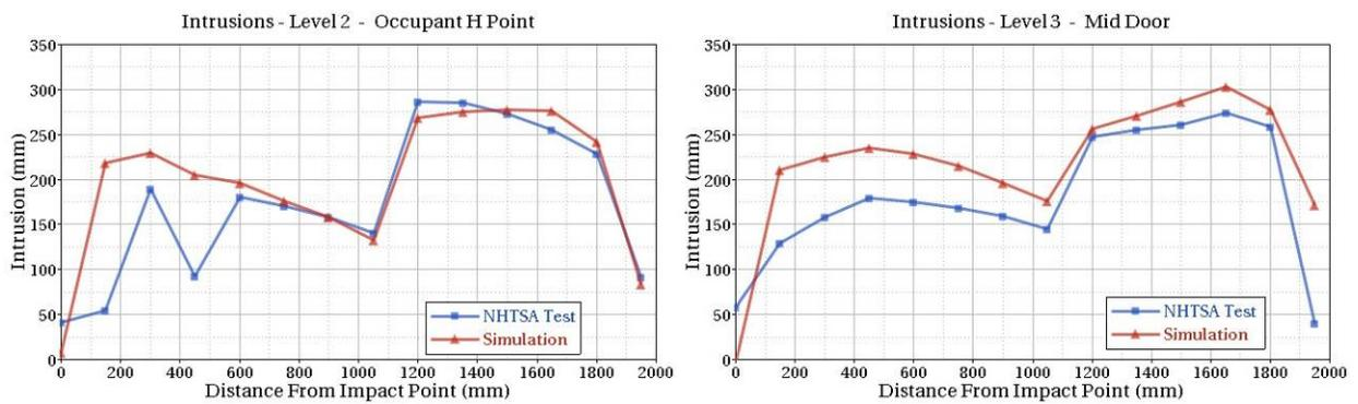
**Figure 50: Model and Test #7098 Level 2 and 3 Struck-Side Intrusion Profile**
