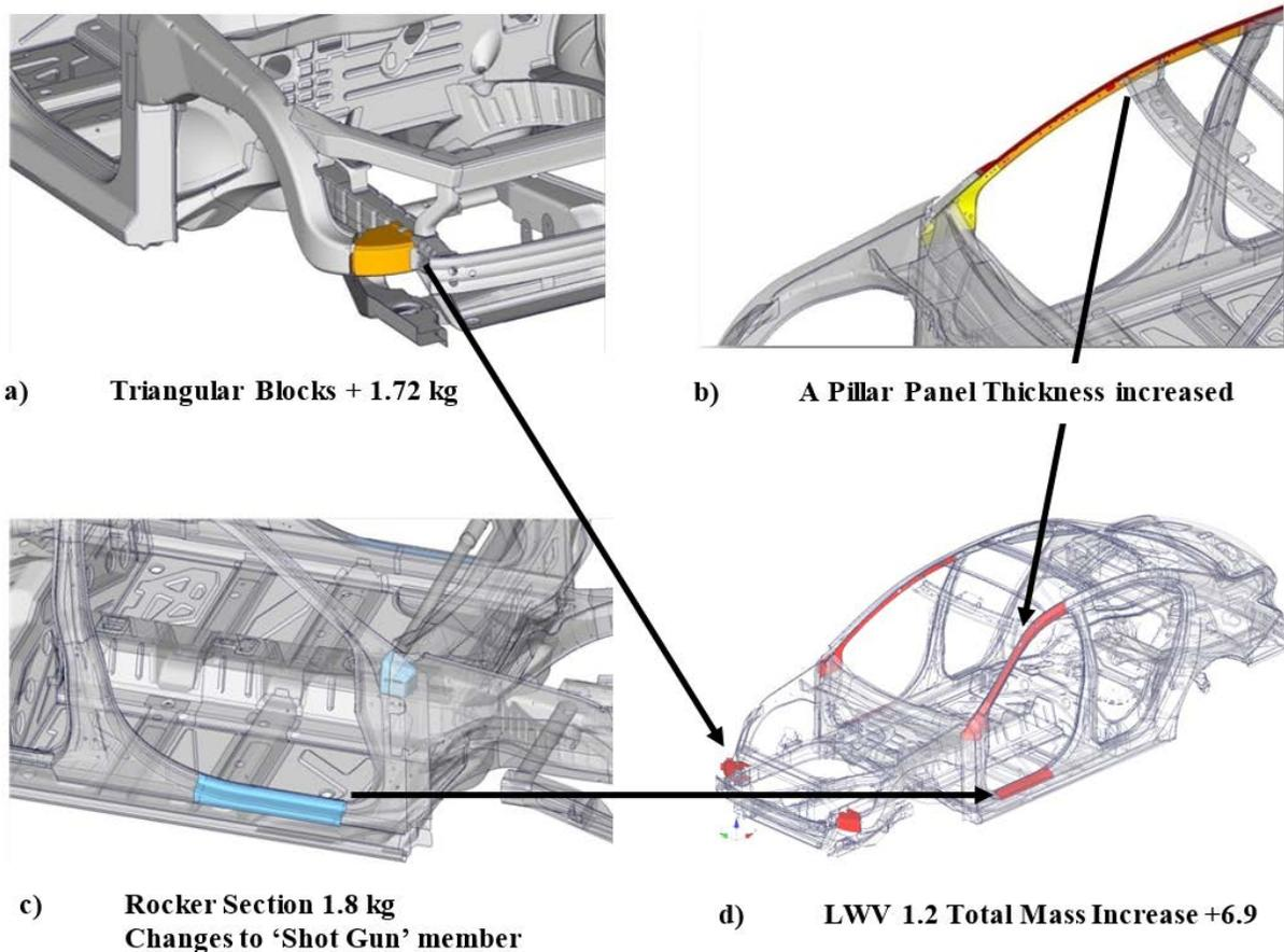
**Figure 95: Recommended changes to meet SOL test requirements**
