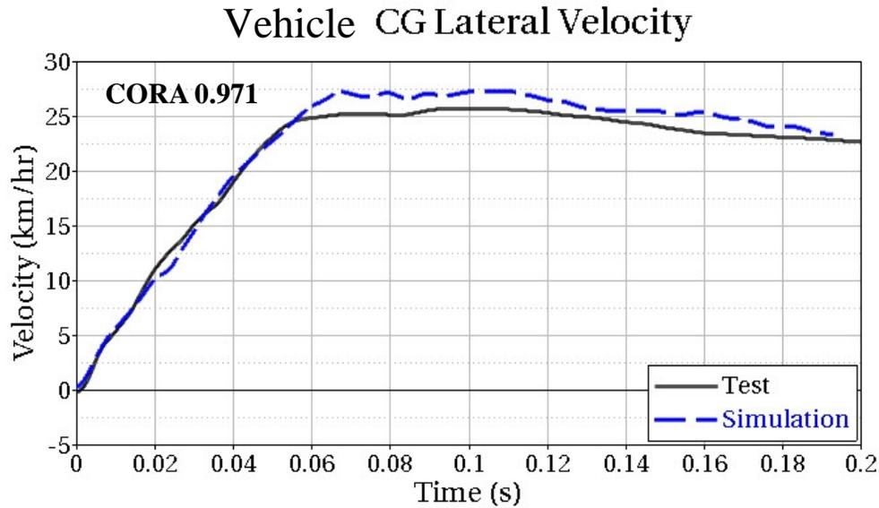
**Figure 52: Model and Test #7098 Center-of-Gravity Lateral Velocity**
