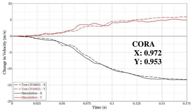
**Figure 81: Comparison of velocity at the center of gravity for laboratory test and simulation for IIHS SOL test**
