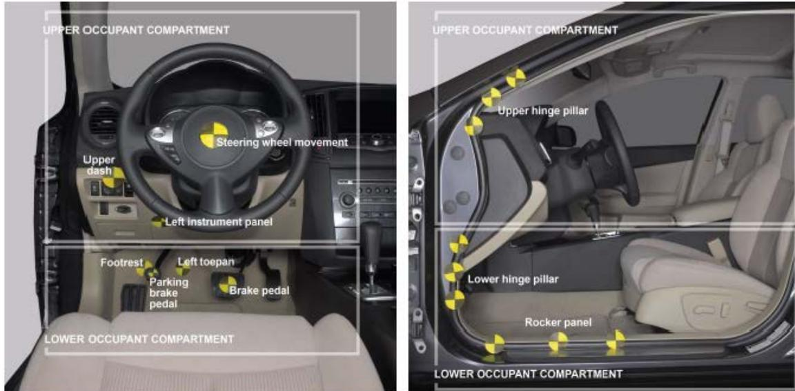
**Figure 34: Locations used for measuring vehicle intrusion**
