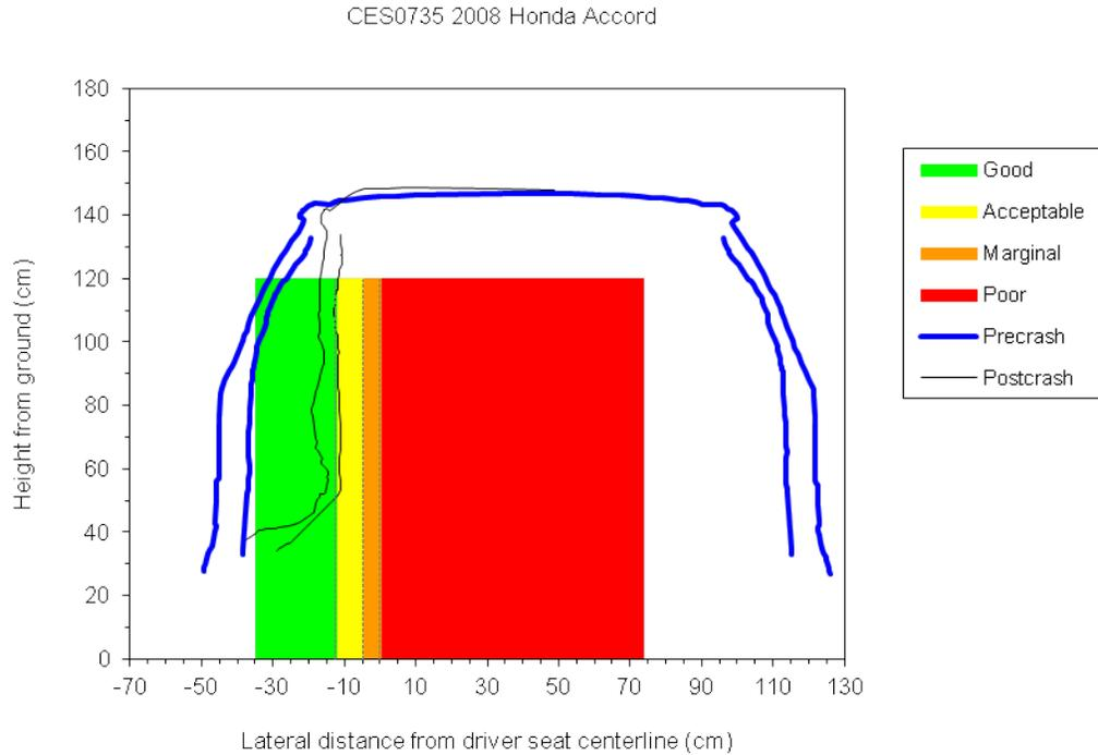
**Figure 27: Honda Accord was rated “Good” in the IIHS side impact test<sup>42</sup>**
