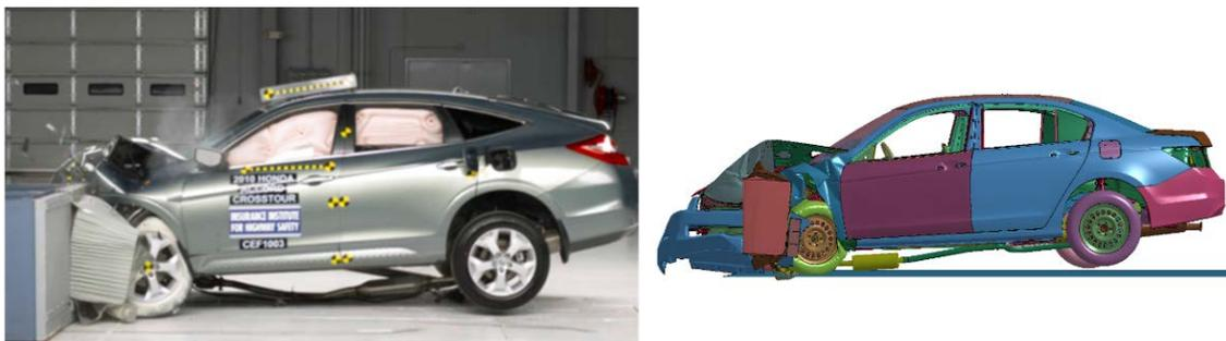
**Figure 72: Post-test laboratory vehicle and model of the 2011 Honda Accord for IIHS deformable barrier test**
