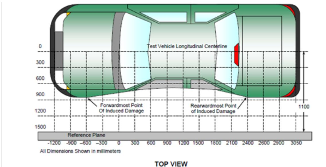
**Figure 12: Diagram used for recording crush in side impact with moving barrier<sup>20</sup>**
