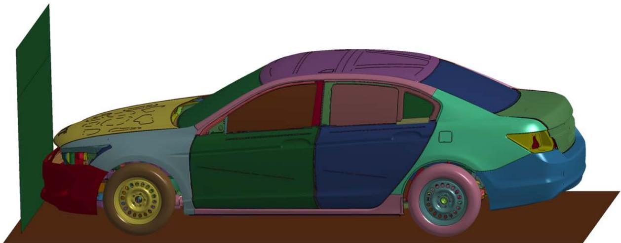
**Figure 107: LS-DYNA set-up for frontal rigid wall test**
