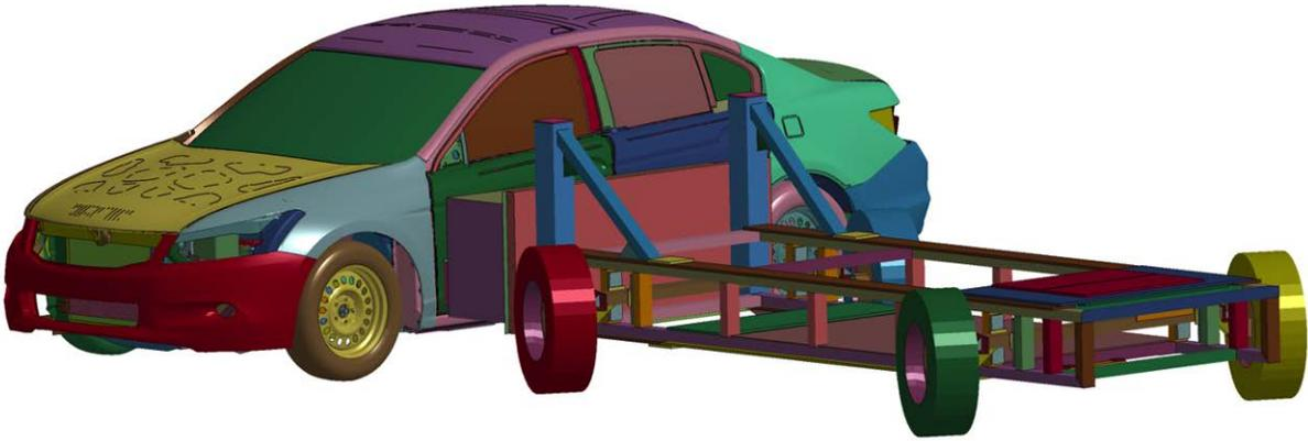
**Figure 115: LS-DYNA set-up for the NCAP moving deformable barrier lateral test**
