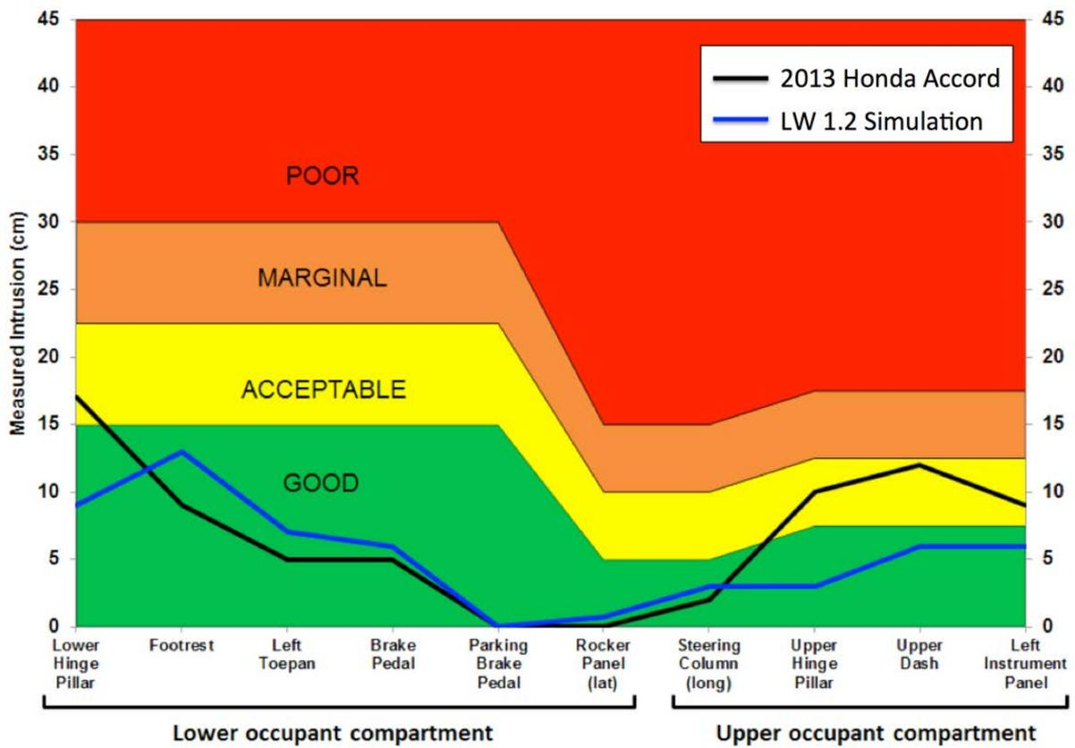
Figure 106: Intrusions of MY2013 Accord and the LWV 1.2 on the IIHS structural measuring scheme
