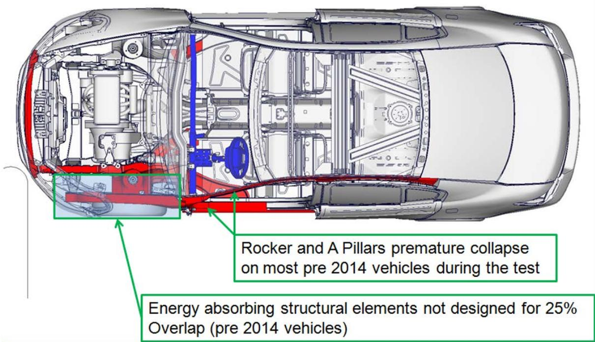
**Figure 94: Typical pre-2014 vehicle design structure**
