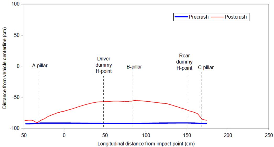
Figure 26: Crush profile at mid-door level for 2008 Honda Accord<sup>41</sup>
