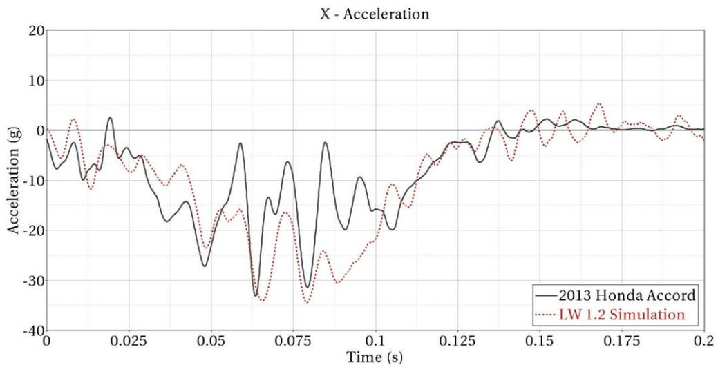
**Figure 102: Crash pulse in the x-direction for the center of gravity of the MY2013 Honda Accord and the LWV 1.2 in IIHS small-overlap impact**
