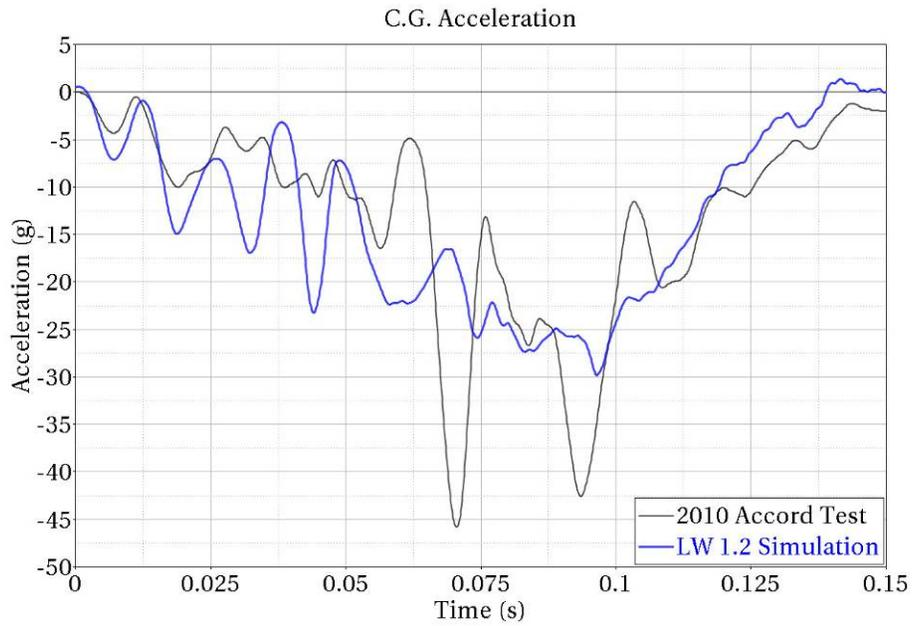
**Figure 139: Crash pulse in the x-direction for the center of gravity of the MY2011 Crosstour and the LWV 1.2 in IIHS frontal test**
