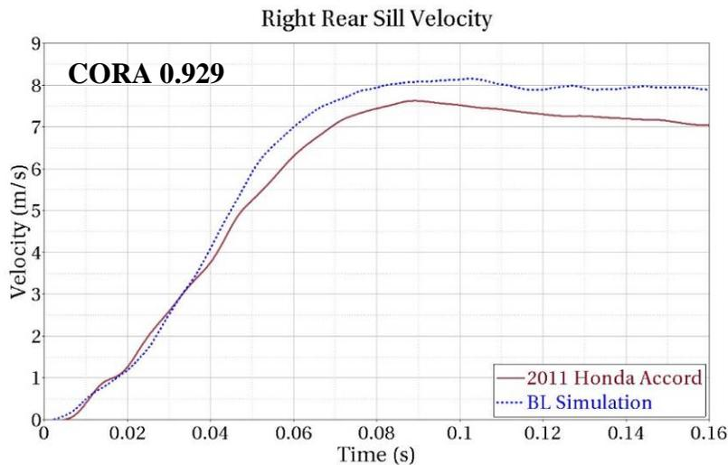
**Figure 69: Model and Test #CES 0735 Vehicle Right Rear Sill Velocity**
