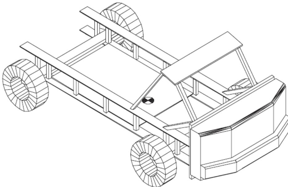
**Figure 24: IIHS deformable barrier used in side impact test<sup>38</sup>**
