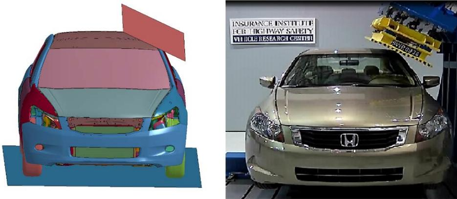
Figure 60: Model and Test #SWR 0936 IIHS Roof Crush Test Setup
