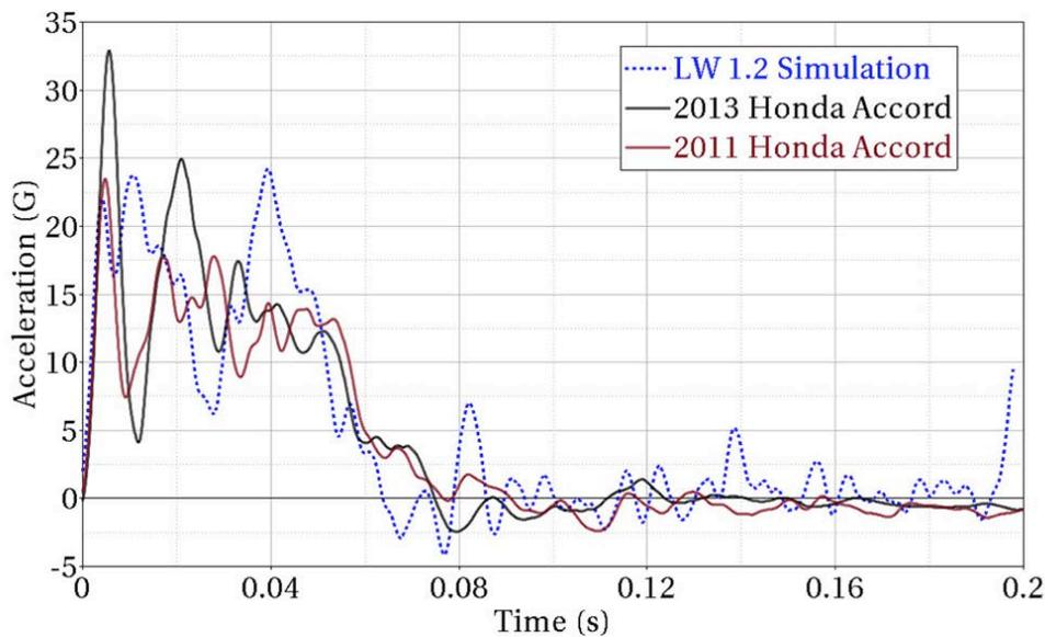
**Figure 121: Lateral acceleration at the center of gravity of MY2011 and MY2013 Accord and LWV 1.2 in NCAP side barrier test**
