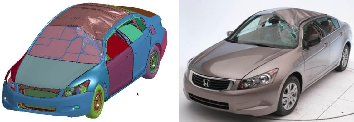
Figure 61: Model and Test #SWR 0936 IIHS Side Post Test
