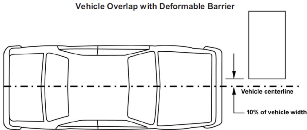
Figure 28: Set-Up of the IIHS frontal 40 percent offset barrier test<sup>44</sup>
