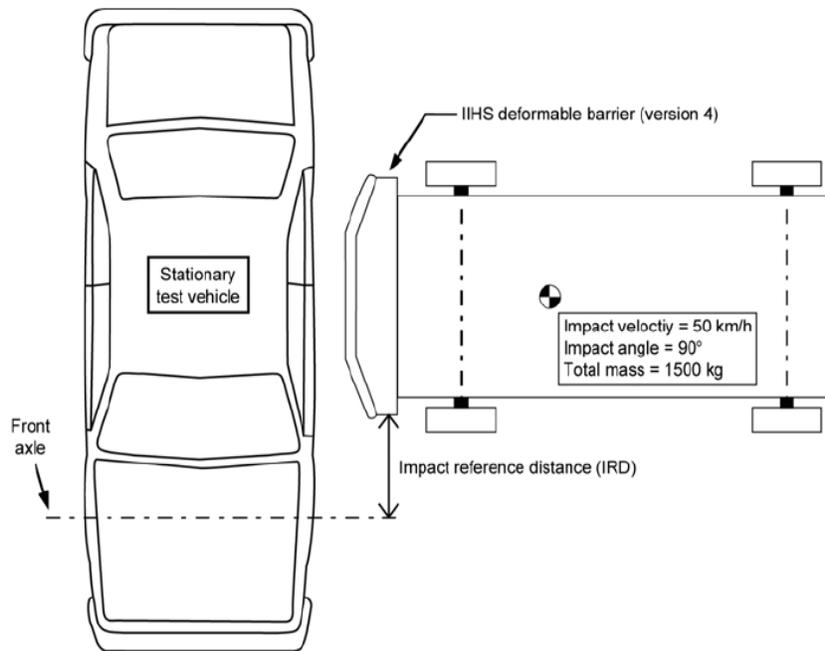
**Figure 23: IIHS moving deformable barrier aligned with vehicle to be tested<sup>37</sup>**
