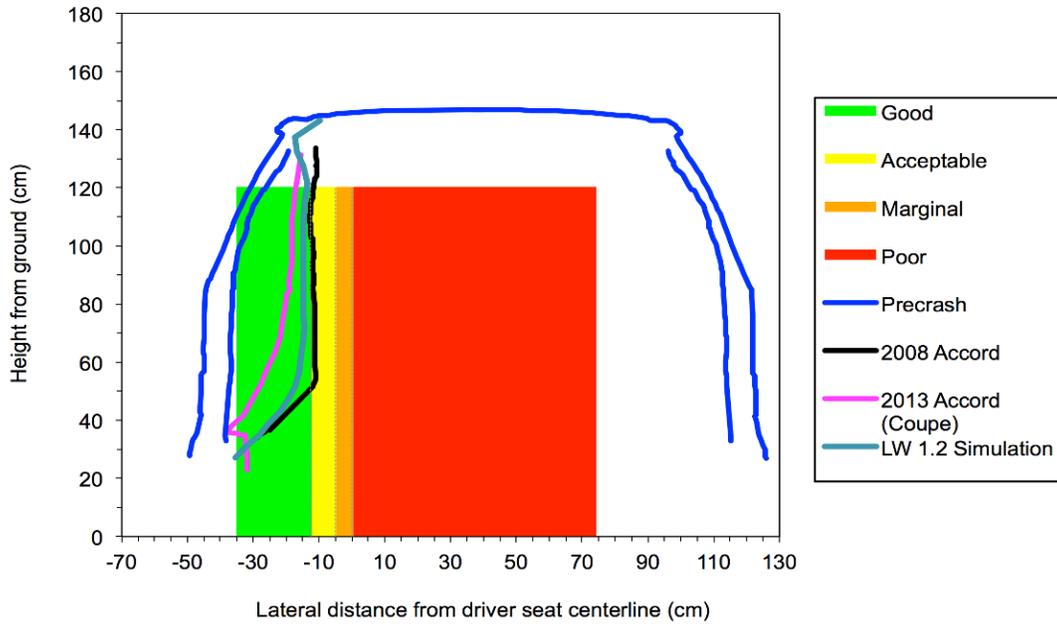
**Figure 120: LWV 1.2 is in the “Green” region for the NCAP side barrier test**
