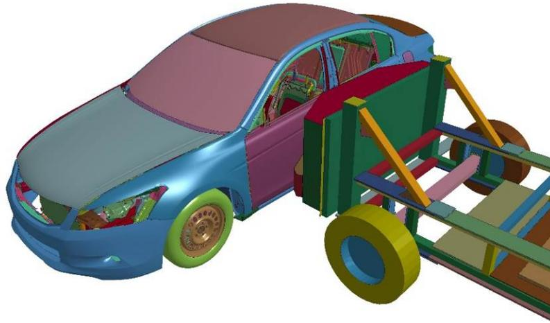
Figure 65: Model and Test #CES 0735 IIHS Lateral MDB Test Setup
