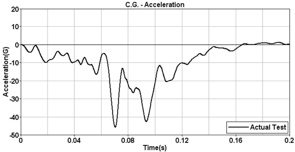
Figure 30: 2010 Honda Crosstour crash pulse in IIHS frontal offset test<sup>47</sup>
