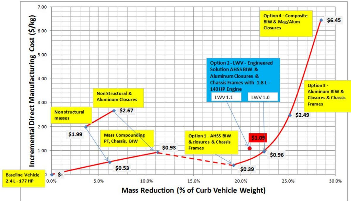
Figure 93: LWV 1.0 and LWV 1.1 mass savings versus costs premium (with Powertrain costs) curve
