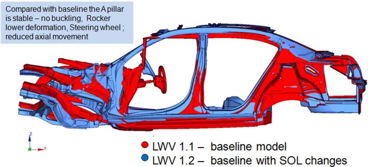
**Figure 97: Comparison structural deformation Baseline LWV 1.1 versus LWV 1.2 with SOL design changes**
