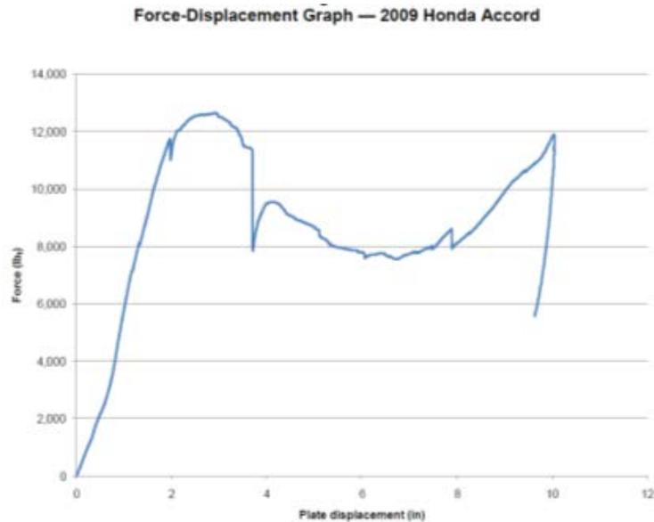
Figure 21: Force versus crush of the platen for Honda Accord 2009<sup>34</sup>
