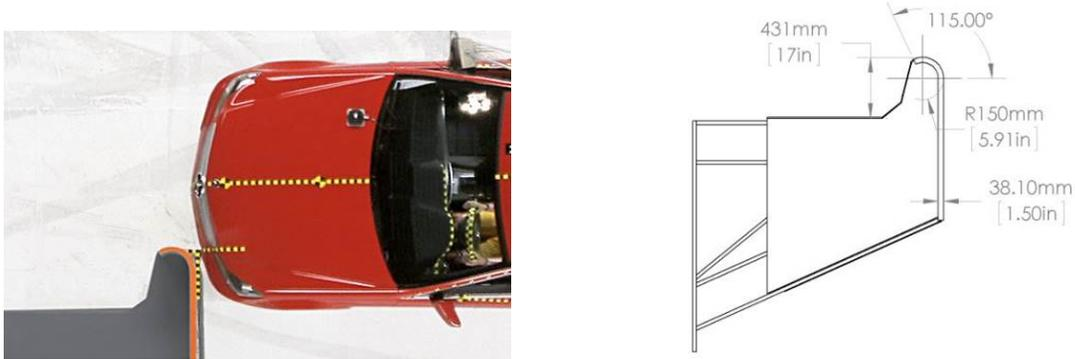
**Figure 32: Configuration of the IIHS SOL test**
