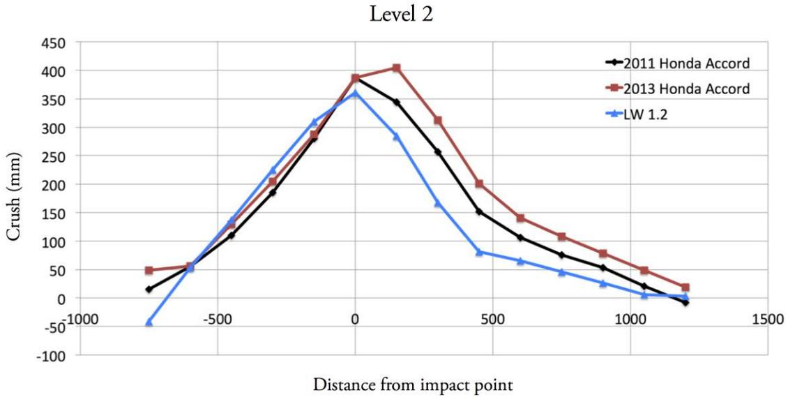
**Figure 127: Exterior crush for level 2, approximately the H-point level in the lateral pole test**
