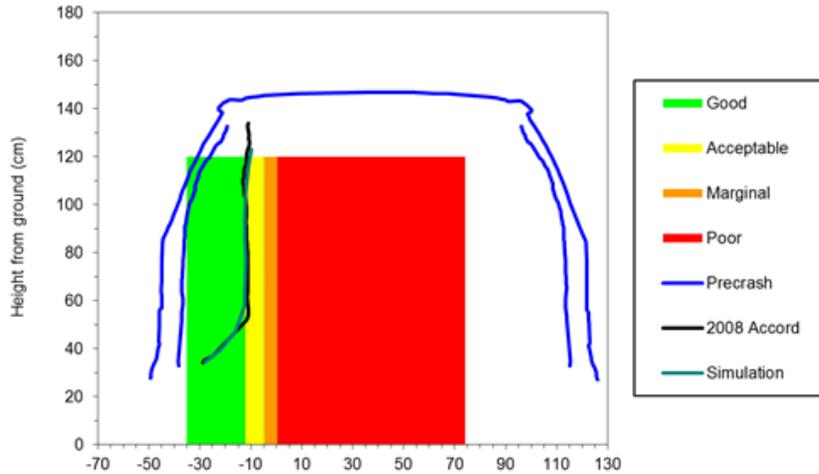
**Figure 68: Model B-Pillar Intrusion Relative to Seat Centerline Test Versus FEA Model**
