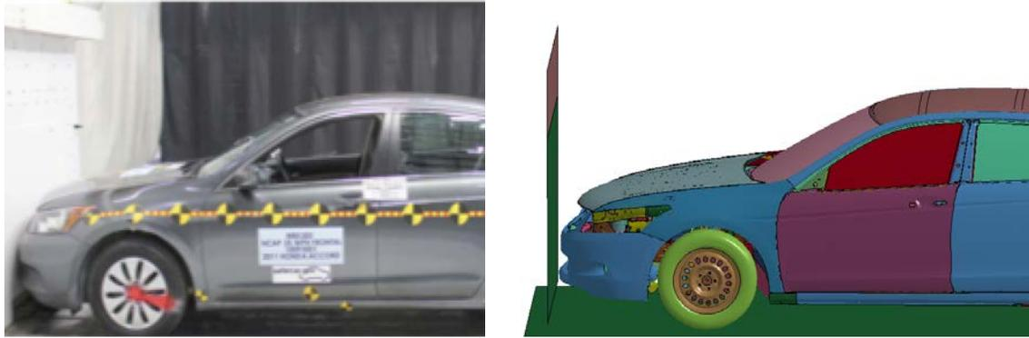
**Figure 42: Pre-test laboratory vehicle and model of the 2011 Honda Accord for NCAP frontal barrier test**
