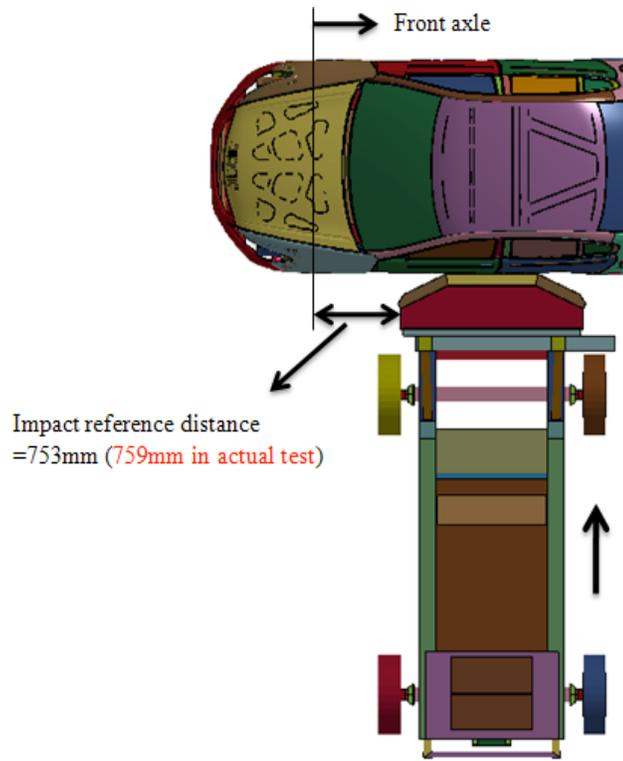
**Figure 133: LS-DYNA set-up for the IIHS lateral impact test**
