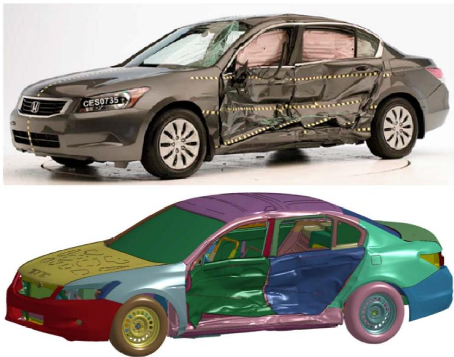
**Figure 134: Post-crash vehicles for the actual laboratory crash and the simulation in IIHS lateral impact test**
