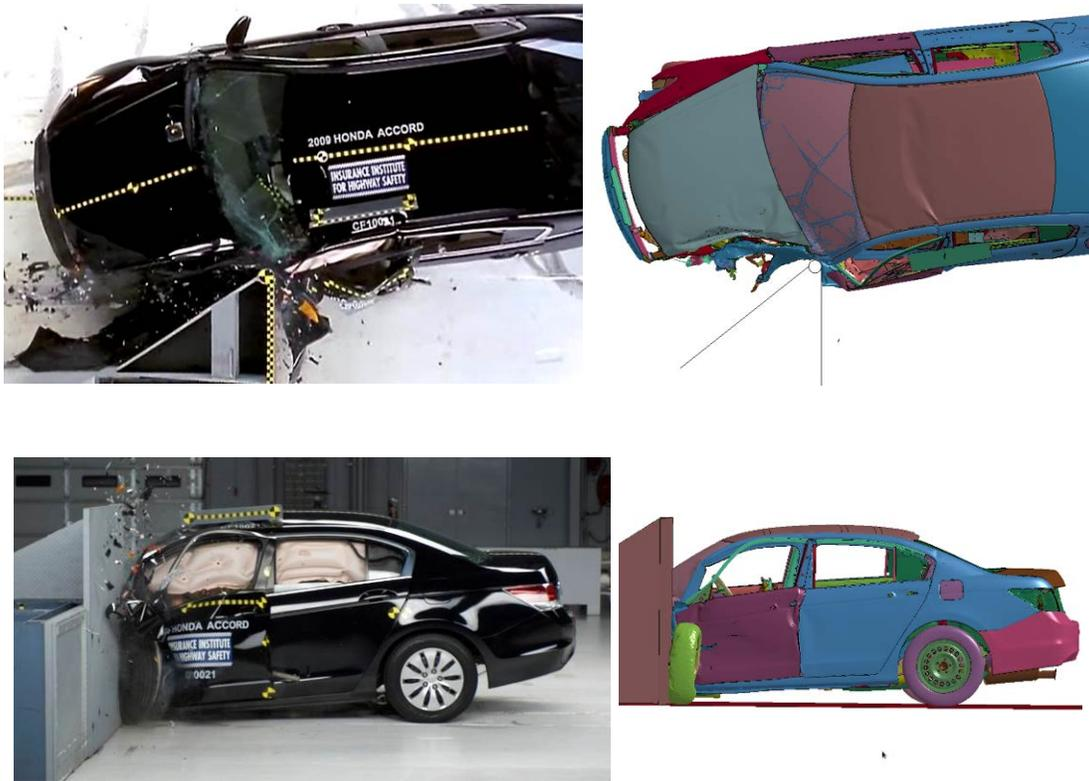
**Figure 78: Post-test laboratory vehicle and model of the 2009 Honda Accord for IIHS SOL test**
