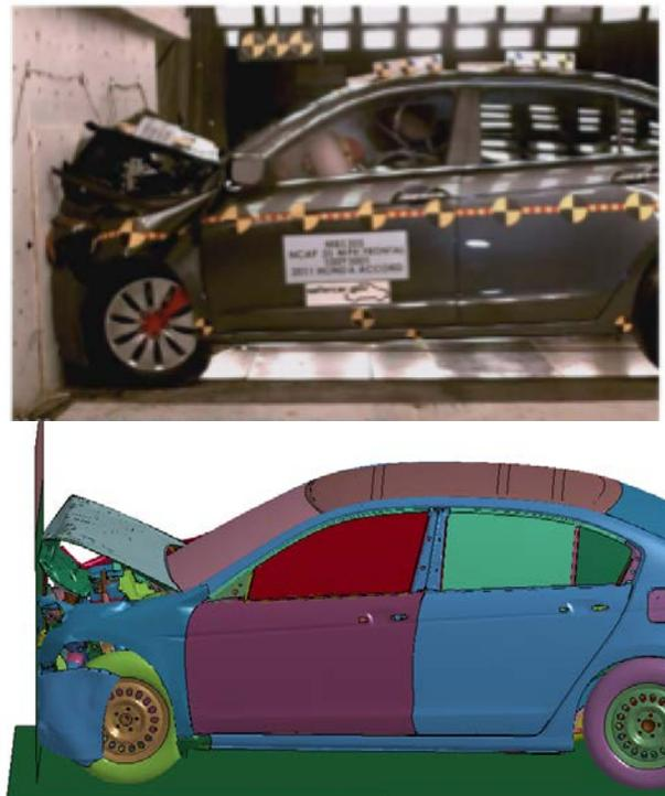
**Figure 43: Post-test laboratory vehicle and model of the 2011 Honda Accord for NCAP frontal barrier test**
