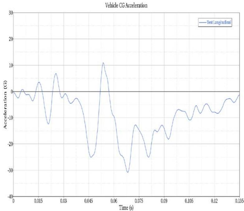
**Figure 38: Acceleration at the vehicle center of gravity, 2009 Honda Accord SOL test**
