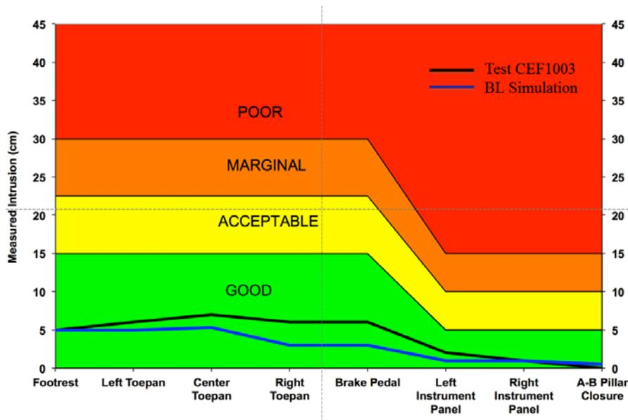
**Figure 75: Maximum intrusion in laboratory test and finite element simulation of baseline Honda Accord in IIHS frontal deformable barrier test using IIHS intrusion rating scheme**
