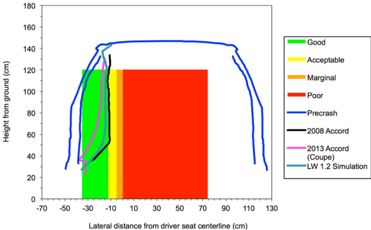
Figure 136: LWV 1.2 is in the “Good” region for the IIHS lateral test
