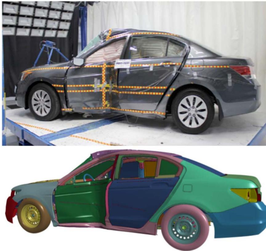
Figure 124: Post-crash vehicles for the actual laboratory crash and the simulation in lateral pole test
