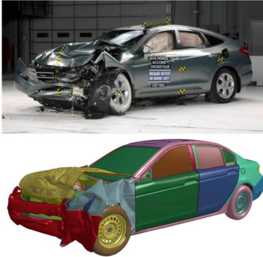
**Figure 138: Post-crash vehicles for the MY2011 BL Honda Crosstour actual laboratory crash and the simulation for LWV 1.2 in the IIHS 40 percent offset frontal test**
