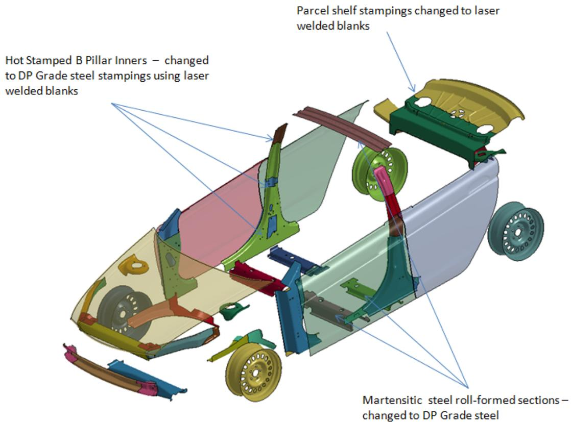
Figure 91: Modified parts from 1.0 to 1.1 design
