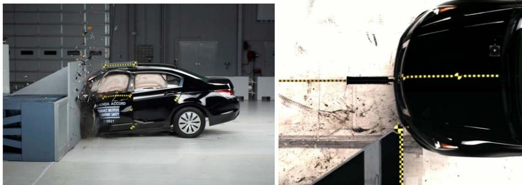
**Figure 35: Two views of the fixed rigid barrier used in IIHS test CF 10021**
