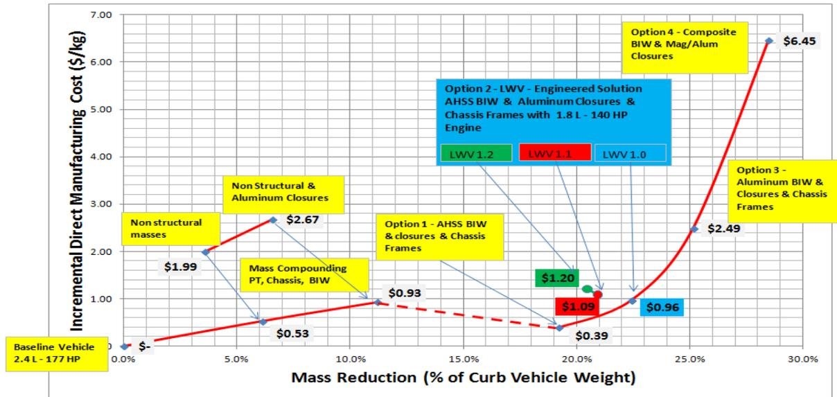
Figure 99: LWV 1.0, LWV 1.1 and LWV 1.2 mass savings versus costs premium (with Powertrain costs) curve
