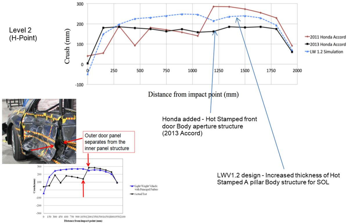
Figure 117: Exterior crush for level 2, approximately the mid-door level in NCAP MDB side test
