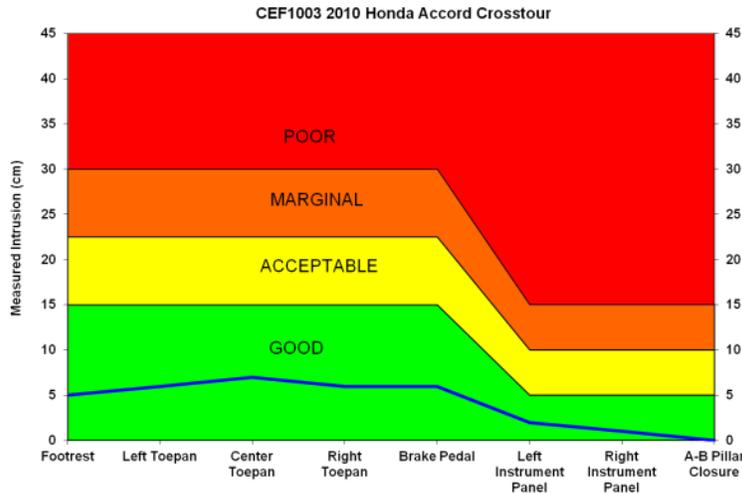
Figure 31: Honda Crosstour was rated “Good” in the IIHS frontal offset test<sup>48</sup>
