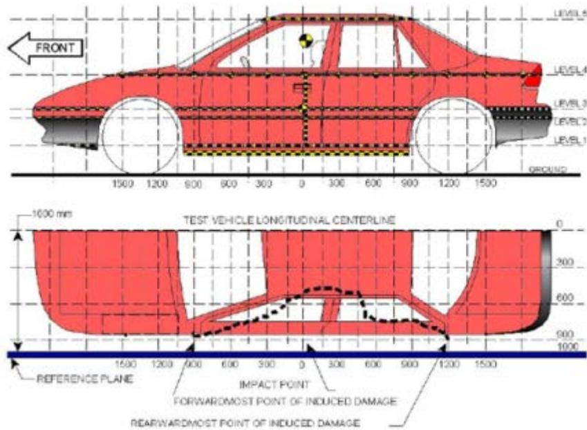
Figure 17: Diagram used for recording crush in side impact with rigid pole<sup>28</sup>
