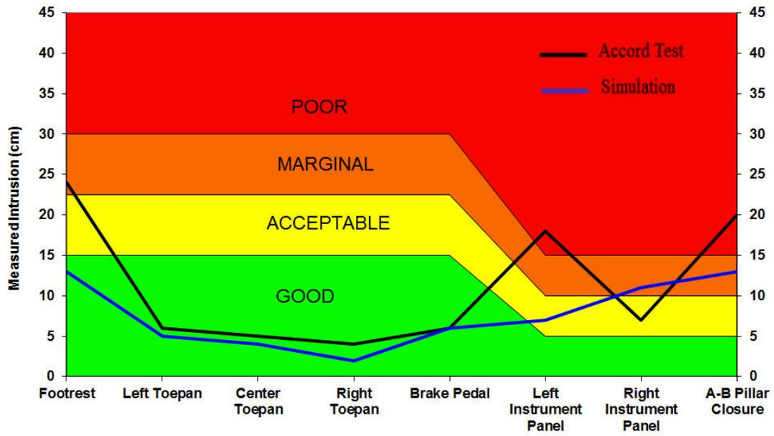
Figure 82: Maximum intrusion in laboratory test and finite element simulation in IIHS SOL frontal impact
