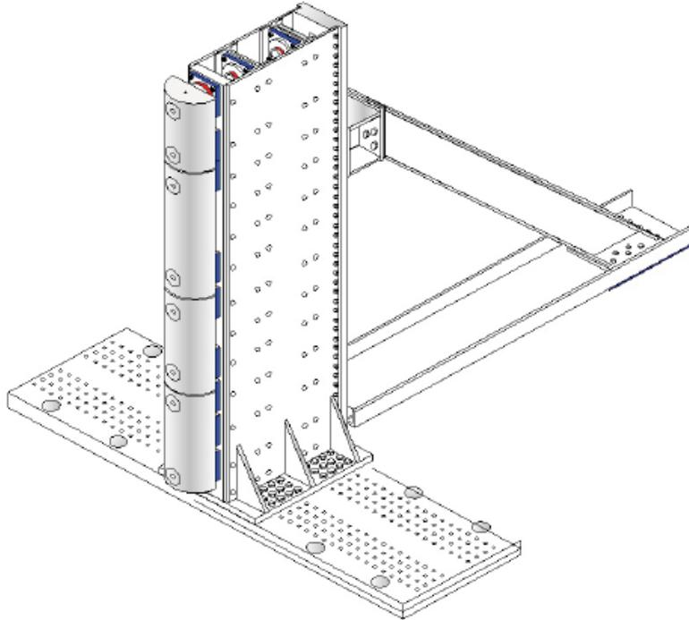
**Figure 14: Fixed, rigid pole 254 mm (10 inches) in diameter, used for NCAP side pole test<sup>23</sup>**
