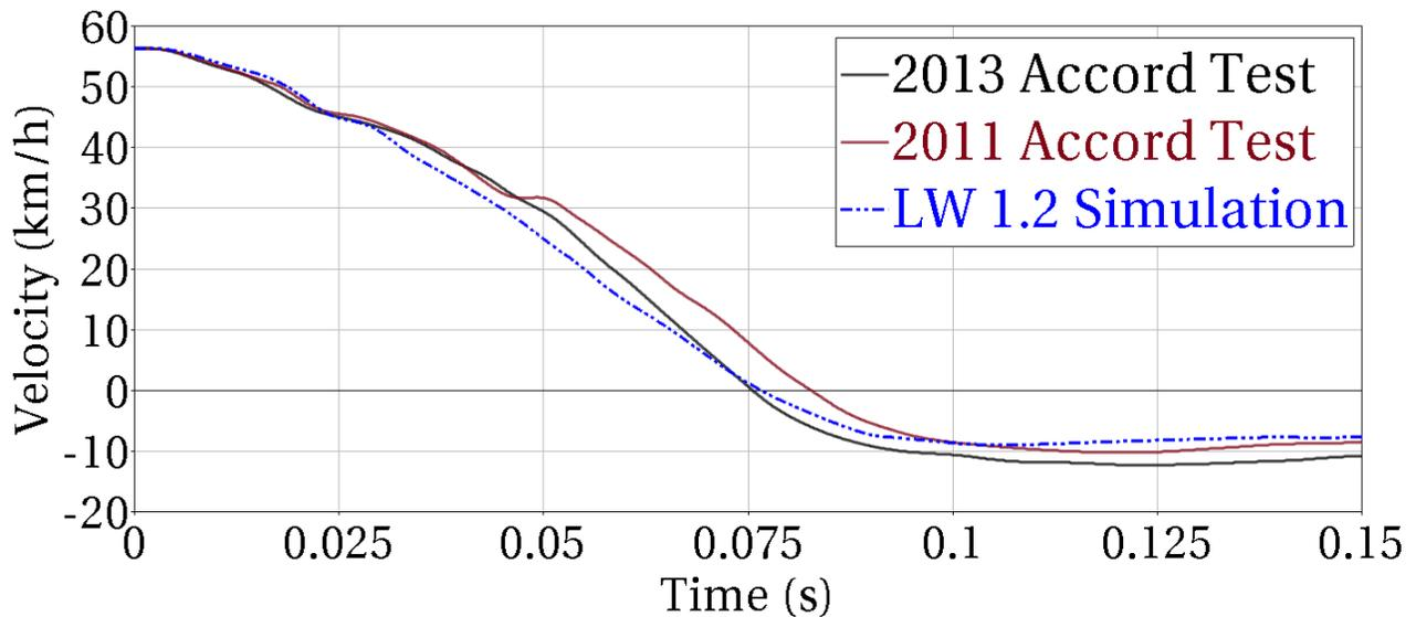
**Figure 111: Velocity of MY2011 and MY2013 Accord and LWV 1.2 for left-rear sill in rigid wall crash**
