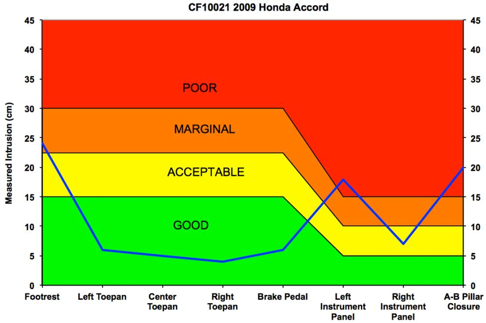
**Figure 36: Occupant compartment intrusion for 2009 Honda Accord SOL test**
