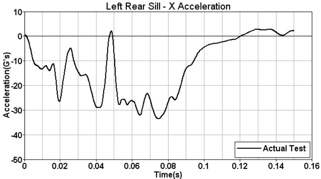
**Figure 6: Crash pulse from frontal NCAP test of Honda Accord 2011**
