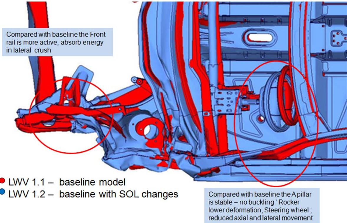
**Figure 96: Comparison structural deformation Baseline LWV 1.1 versus LWV 1.2 with SOL design changes**
