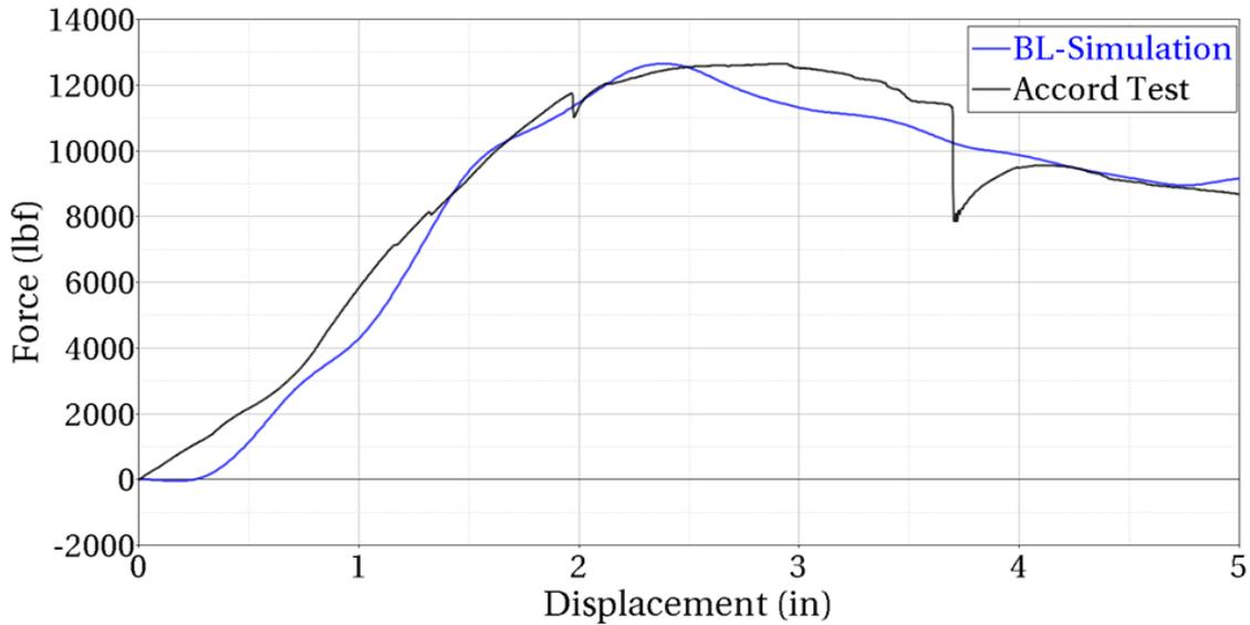
**Figure 63: Model and Test #SWR 0936 IIHS Side Force Versus Platen Displacement Overlay**
