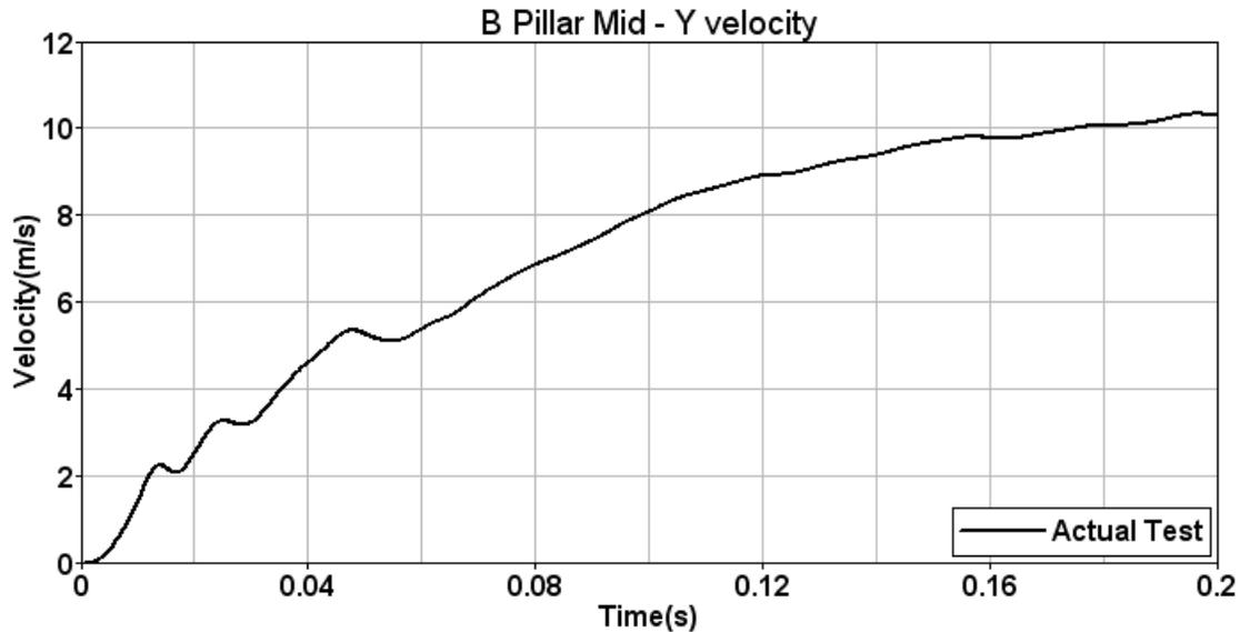
Figure 16: Velocity versus time for the left middle B-pillar for the side NCAP test with the rigid pole<sup>27</sup>
