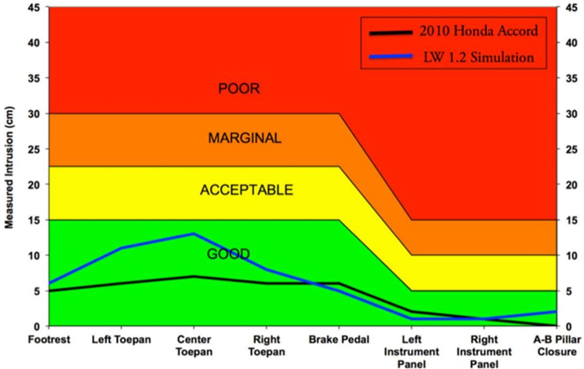
Figure 140: Intrusions of MY2010 Crosstour and the LWV 1.2 on the IIHS structural measuring scheme
