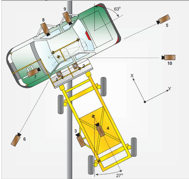
Figure 10: Orientation of trolley to struck vehicle in NCAP side test with moving deformable barrier<sup>16</sup>
