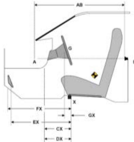
**Figure 8: Scheme for driver compartment intrusion measurement<sup>13</sup>**
