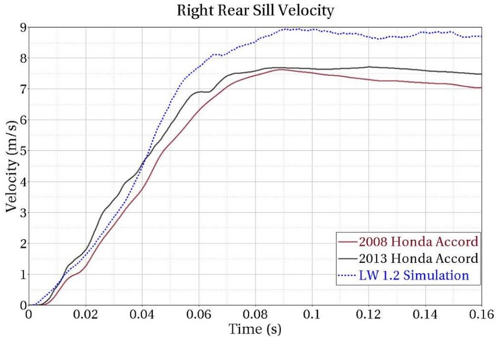
Figure 135: Velocity versus time plot at the right-rear sill on the non-struck side of MY2008 and MY2013 Accord and LWV 1.2
