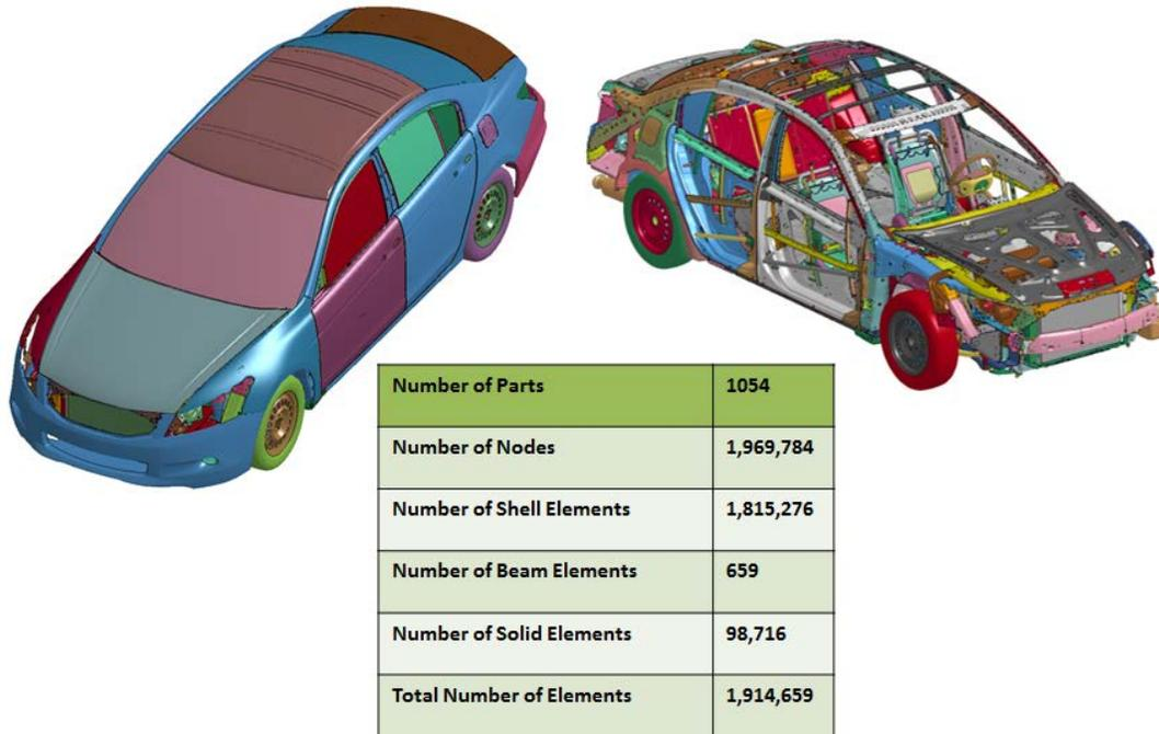
**Figure 40: Model characteristics of 2011 Honda Accord finite element model**
