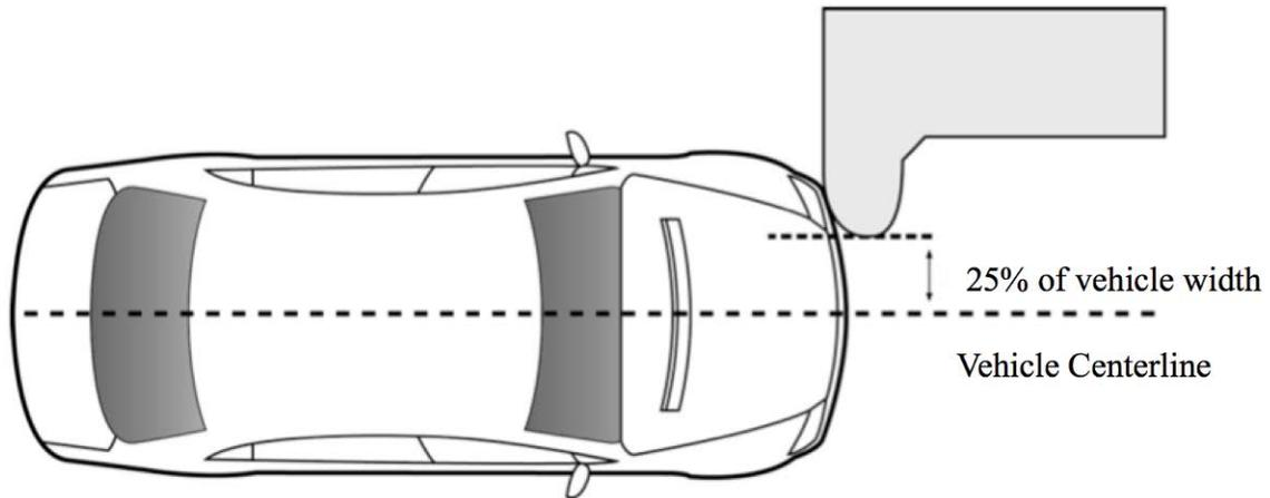
**Figure 33: Vehicle overlay on flat 150 small-overlap barrier**
