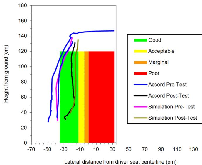
**Figure 51: Model and Test #7098 B-Pillar Inner Intrusion Profile**
