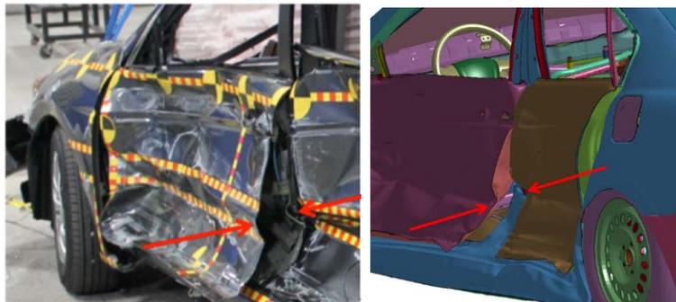
**Figure 53: Model and Test #7098 Level 2 Struck-Side Intrusion Profile**
