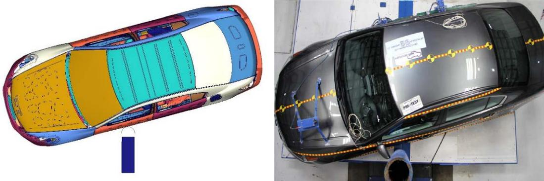
**Figure 55: Model and Test #7077 NCAP Pole Test Setup**
