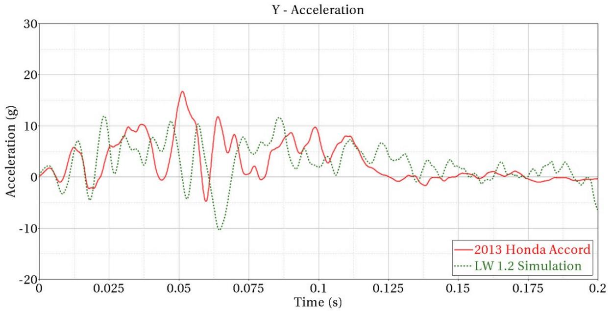
**Figure 103: Crash pulse in the y-direction for the center of gravity of the MY2013 Honda Accord and the LWV 1.2 in IIHS small-overlap impact**
