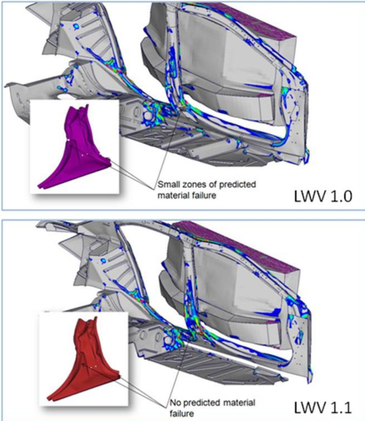
**Figure 86: Side Crash – eliminated material failure by using lower strength higher ductility steel grades**
