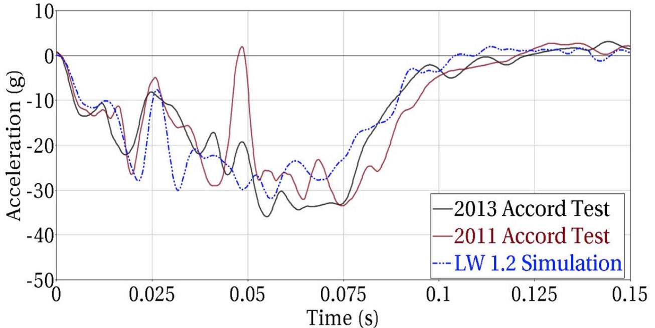
**Figure 109: Acceleration pulse of MY2011 and MY2013 Honda Accord and LWV 1.2 for left-rear sill in rigid-wall crash**
