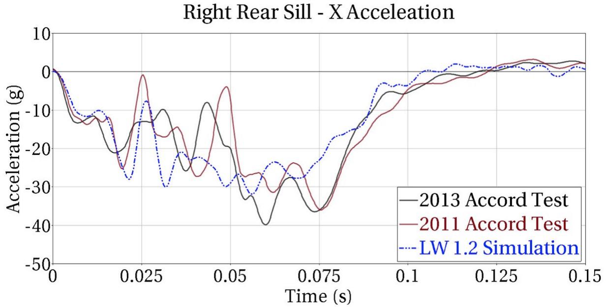
Figure 112: Acceleration pulse of MY2011 and MY2013 Accord and LWV 1.2 for right-rear sill in rigid wall crash
