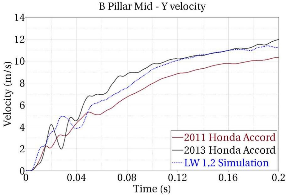
Figure 125: Velocity versus time for the mid-B-pillar in the lateral pole test
