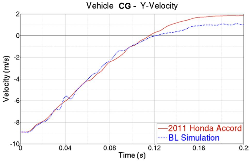
Figure 57: Model and Test #7077 Vehicle CG Velocity
