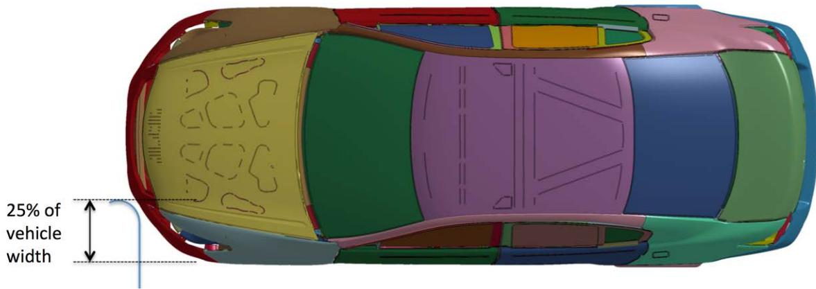
**Figure 100: LS-DYNA set-up for IIHS 25 percent offset small-overlap of the LWV 1.2**
