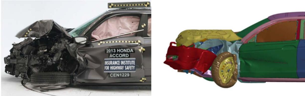
**Figure 101: Post-crash vehicles for the MY2013 Honda Accord actual laboratory crash and the simulation for LWV 1.2 in the IIHS small-overlap test**
