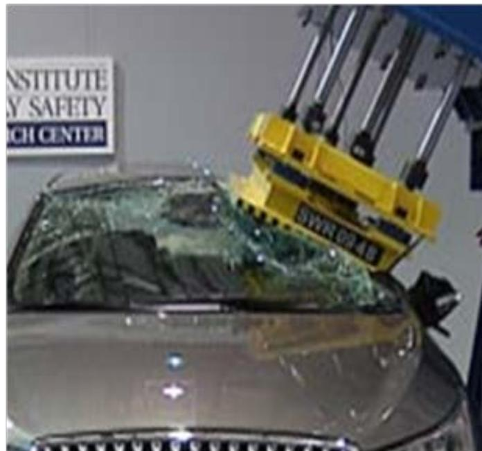
Figure 19: Test set-up for IIHS roof crush test<sup>31</sup>
