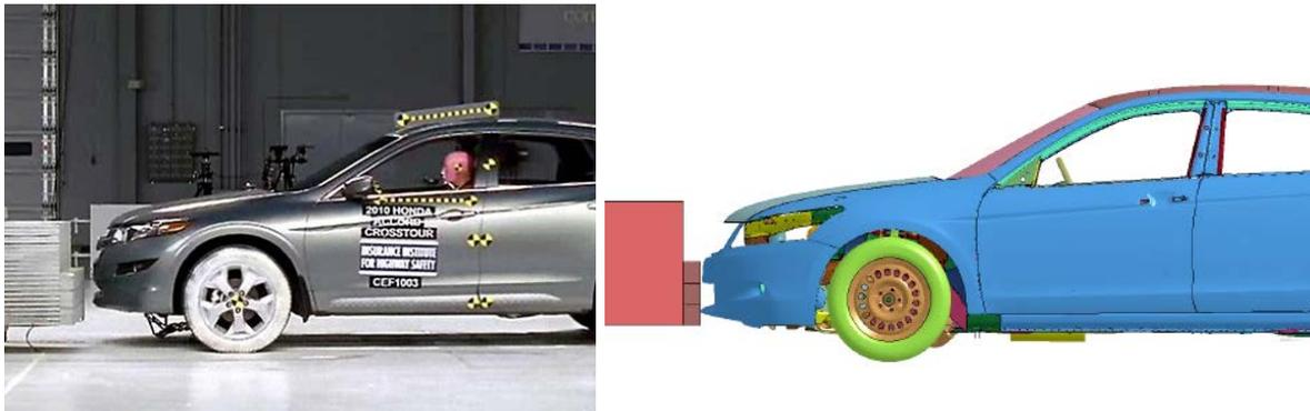
**Figure 71: Pre-test laboratory vehicle and model of the 2011 Honda Accord for IIHS frontal deformable barrier test**
