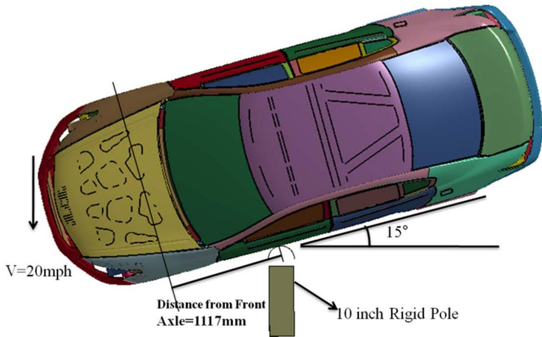
Figure 123: LS-DYNA set-up for the NCAP side pole test
