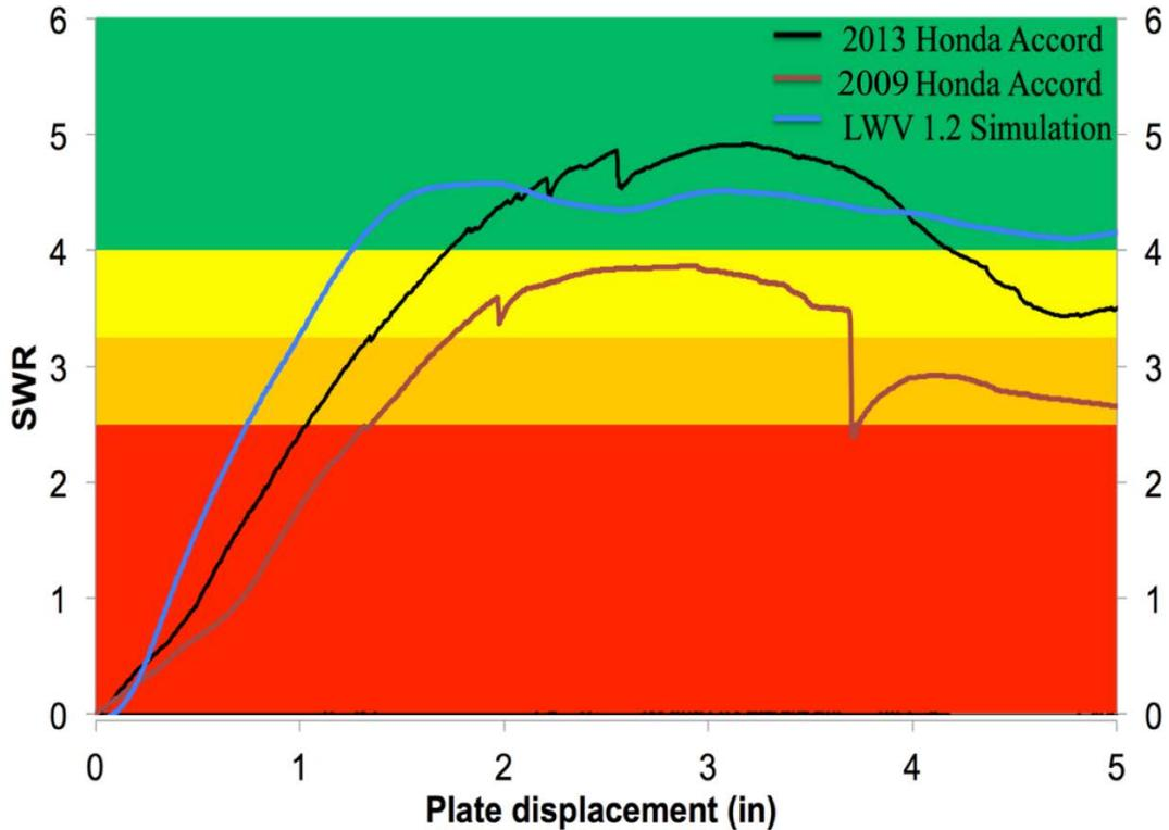
Figure 132: Force divided by curb weight versus platen displacement for MY2009 and MY2013 Honda Accord and LWV 1.2 in IIHS roof crush test
