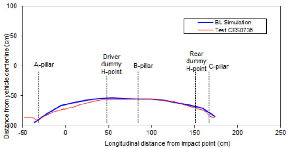
Figure 67: Model and Test #CES 0735 IIHS Side Intrusion Test and Model Overlay
