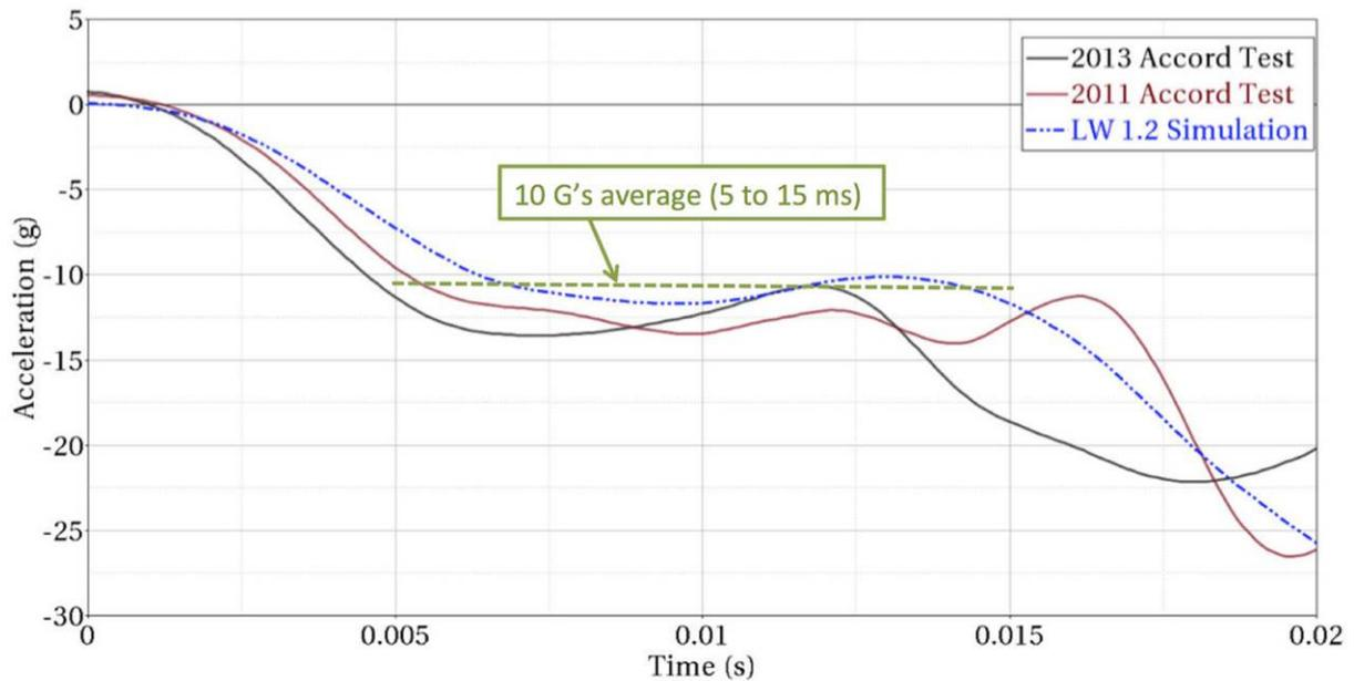
**Figure 110: Acceleration pulse of MY2011 and MY2013 Honda Accord and LWV 1.2 for left-rear sill in rigid wall crash 0 to 20 ms**
