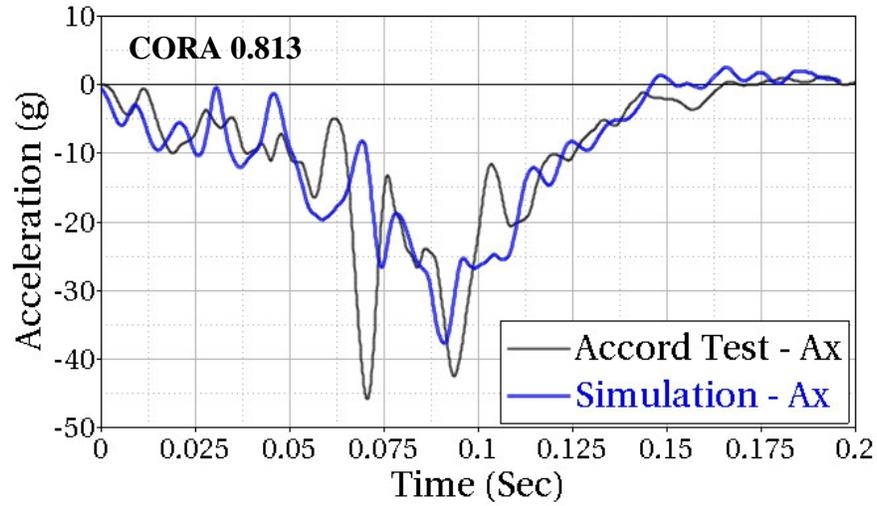
**Figure 73: Comparison of center of gravity accelerations for laboratory test and simulation for IIHS frontal deformable barrier test**
