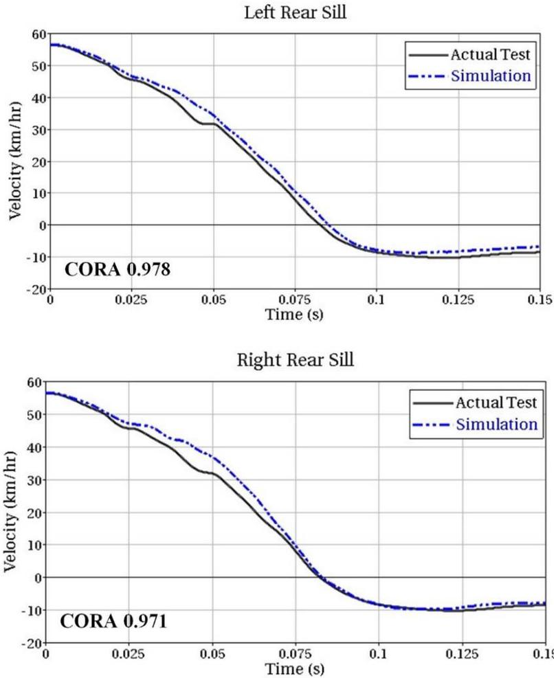
**Figure 45: Comparison of left and right rear seat X velocity for laboratory test and simulation for NCAP frontal crash test**
