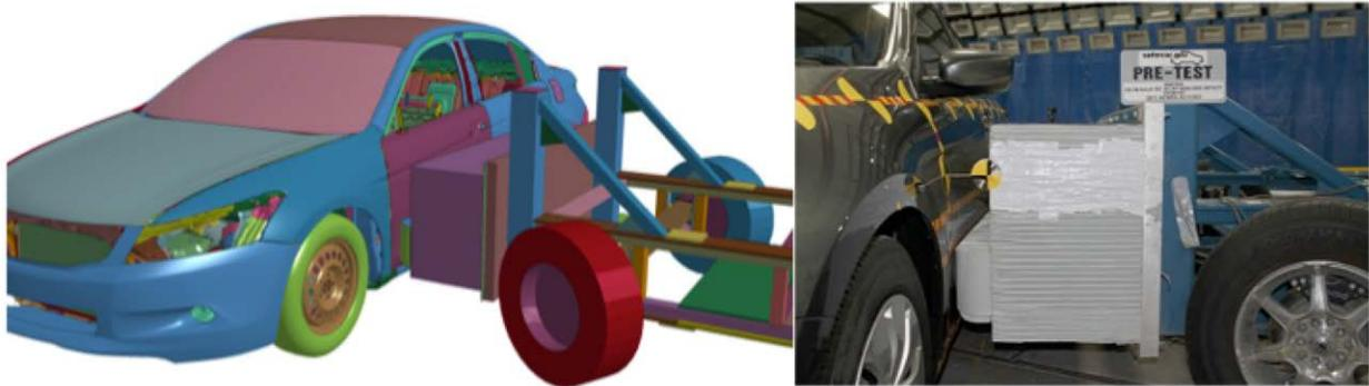
**Figure 48: Model and Test #7098 Lateral NCAP MDB Test Setup**
