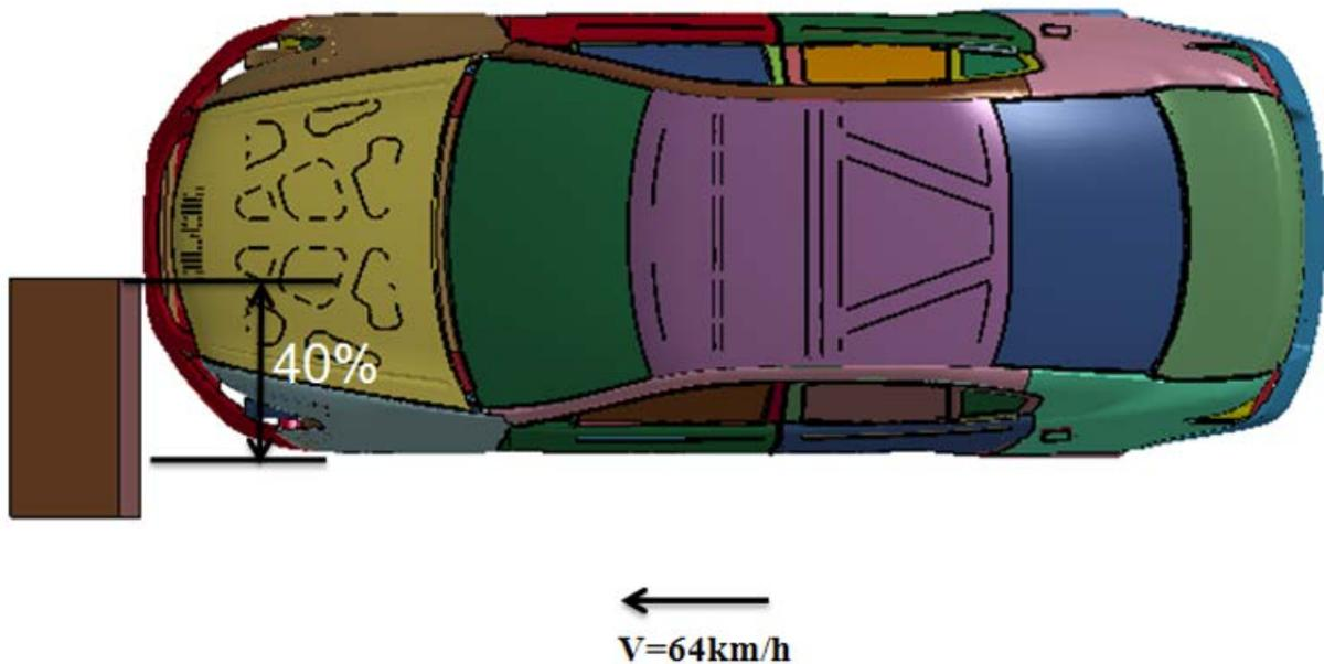
**Figure 137: LS-DYNA set-up for the 40 percent offset frontal crash test into a deformable barrier of the LWV 1.2**
