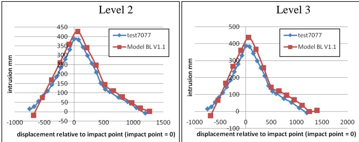
Figure 59: Model and Test #7077 Level 2 and 3 Struck-Side Intrusion Profile
