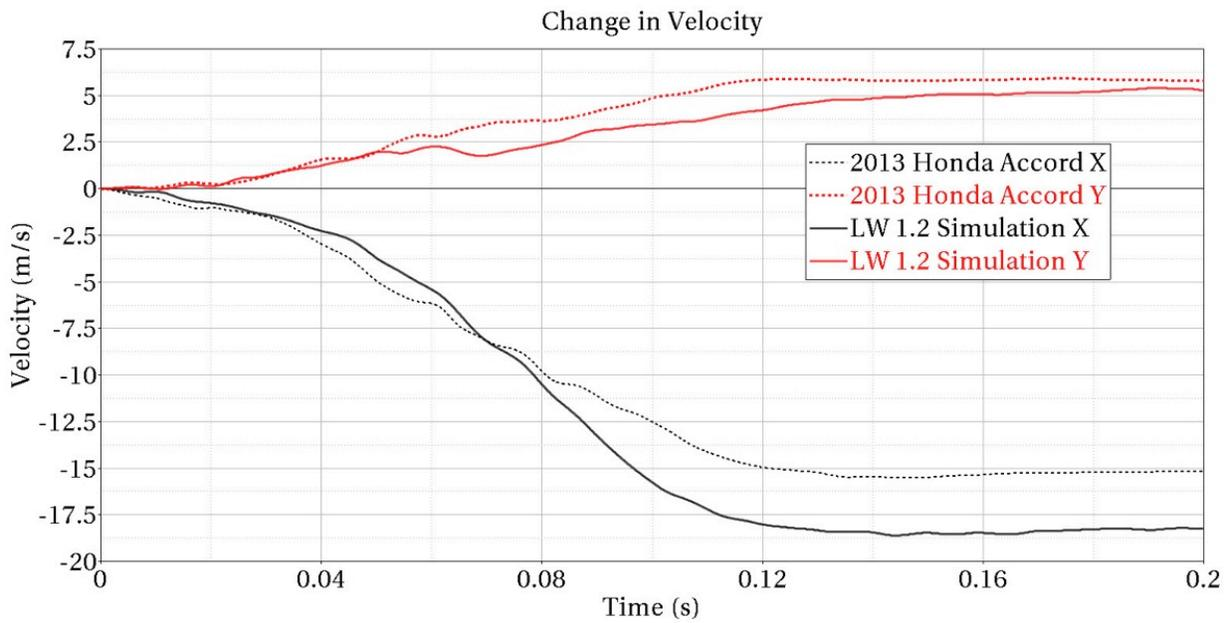
**Figure 104: Change in velocity in x- and y-direction of MY2013 Accord and LWV 1.2**
