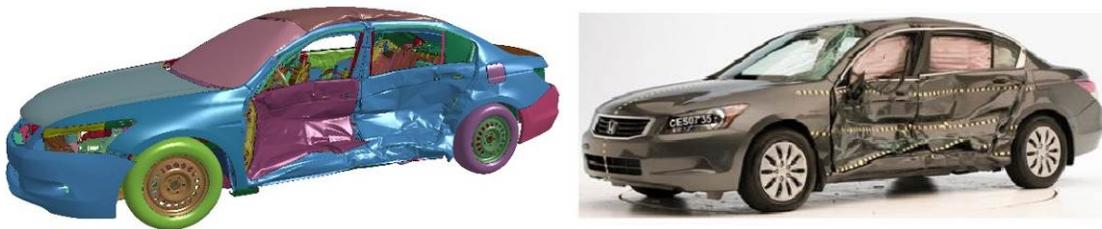
Figure 66: Model and Test #CES 0735 IIHS Lateral MDB Post Test
