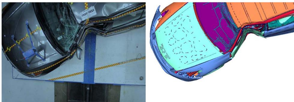
**Figure 56: Model and Test #7077 Lateral NCAP Pole Post Test**
