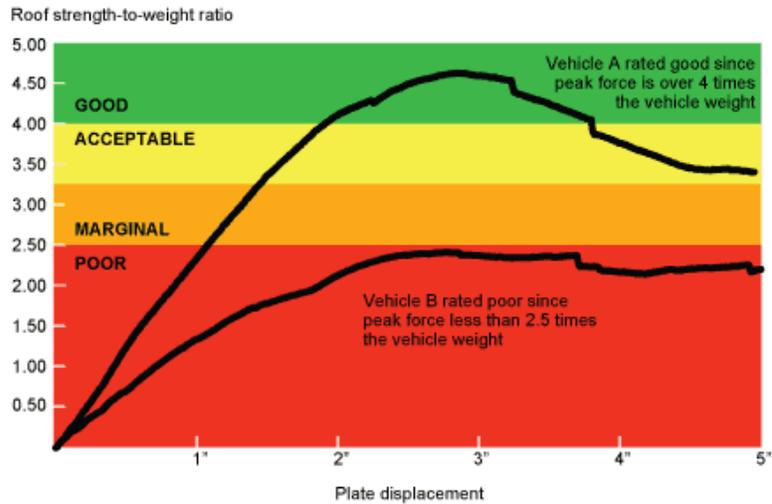
Figure 20: IIHS Sample data comparing test results for vehicles rated “Good” and “Poor”<sup>32</sup>
