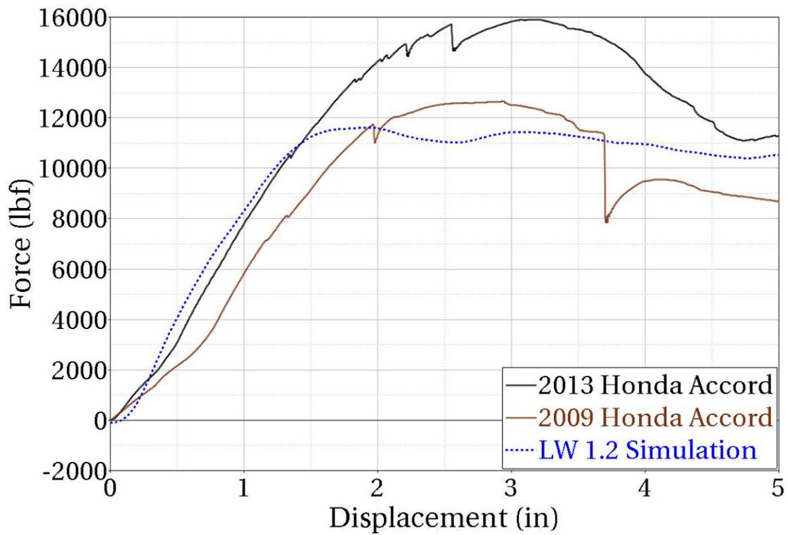
Figure 131: Force versus platen displacement for MY2009 and MY2013 Accord and LWV 1.2 in IIHS roof crush test
