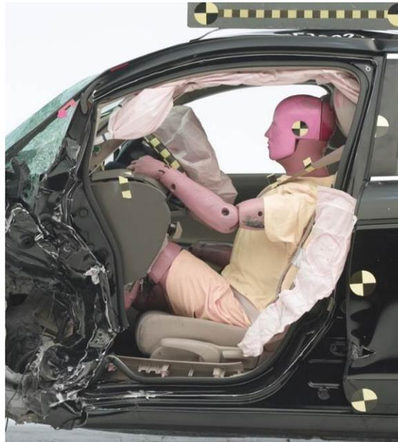
**Figure 37: Dummy and vehicle interior, post-crash, 2009 Honda Accord SOL test**
