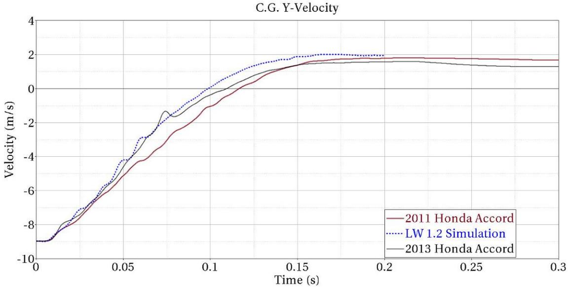
Figure 126: Lateral velocity at the center of gravity of LWV 1.2 and MY2011 and MY2013 Accords in the NCAP side pole test
