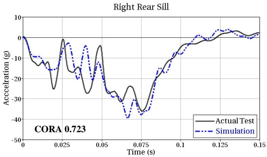
**Figure 44: Comparison of left and right rear seat X accelerations for laboratory test and simulation for NCAP frontal crash test**
