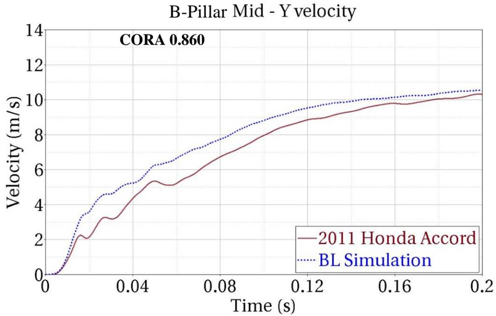
Figure 58: Model and Test #7077 Struck-Side Mid-B-Pillar Velocity
