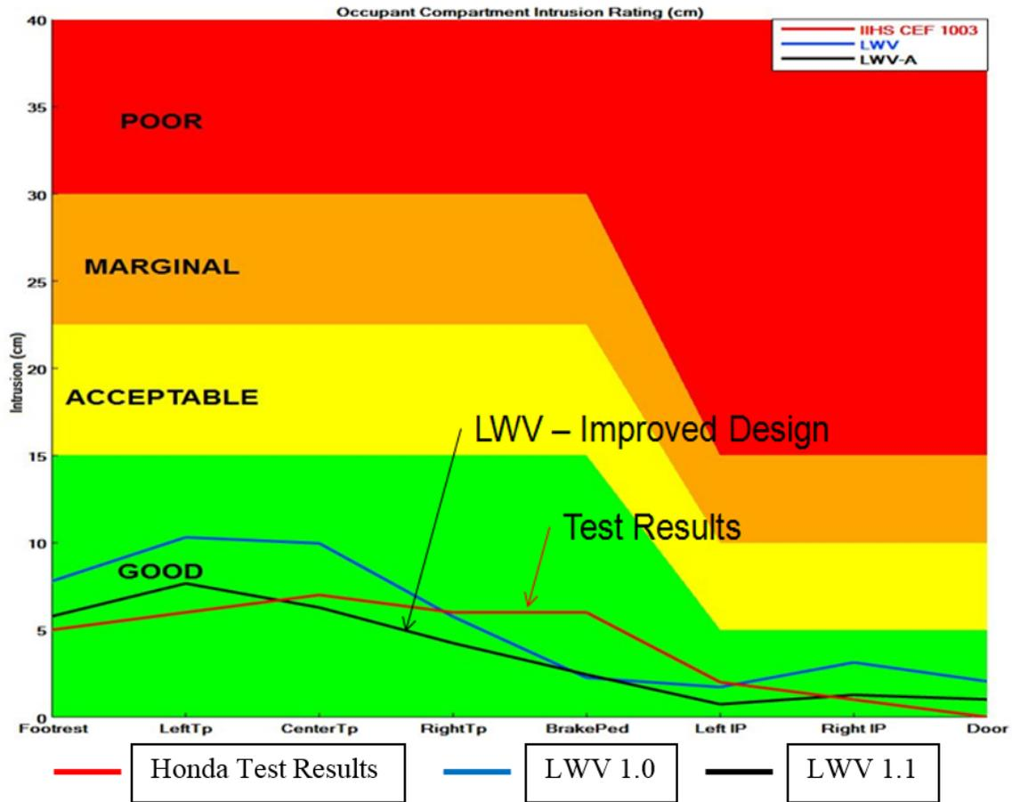
Figure 85: IIHS Offset Barrier – reduced passenger compartment intrusions LWV 1.1 improved design
