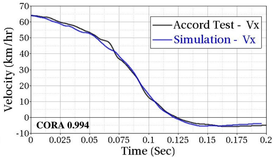
**Figure 74: Comparison of velocity at the center of gravity for laboratory test and simulation for IIHS frontal deformable barrier test**
