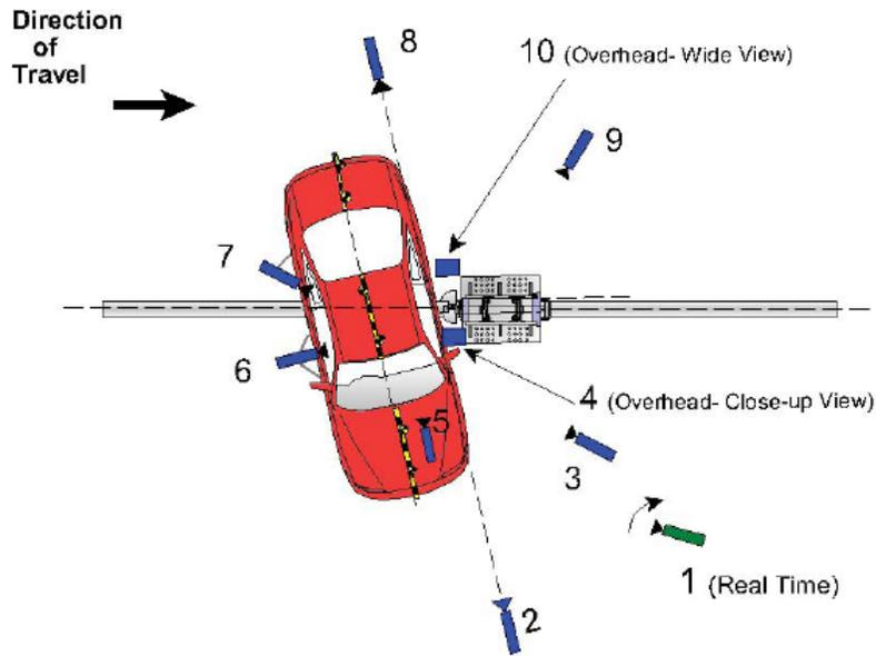
Figure 15: Complete test set-up for NCAP side pole test<sup>26</sup>
