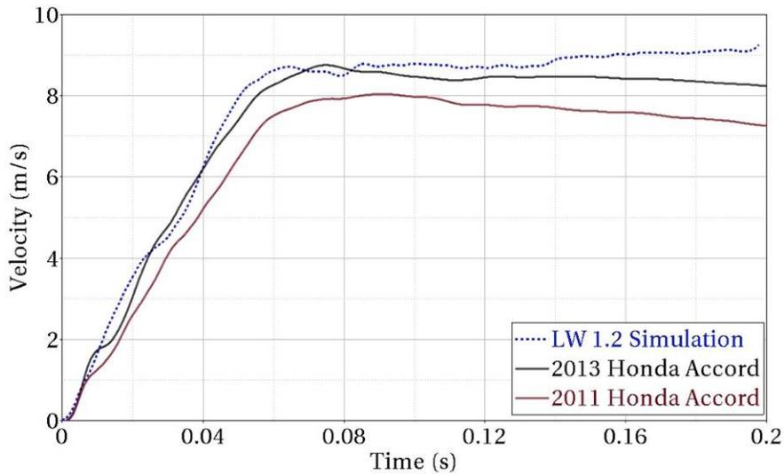
**Figure 122: Lateral velocity at the center of gravity of MY2011 and MY2013 Accord and LWV 1.2 in NCAP side barrier test**
