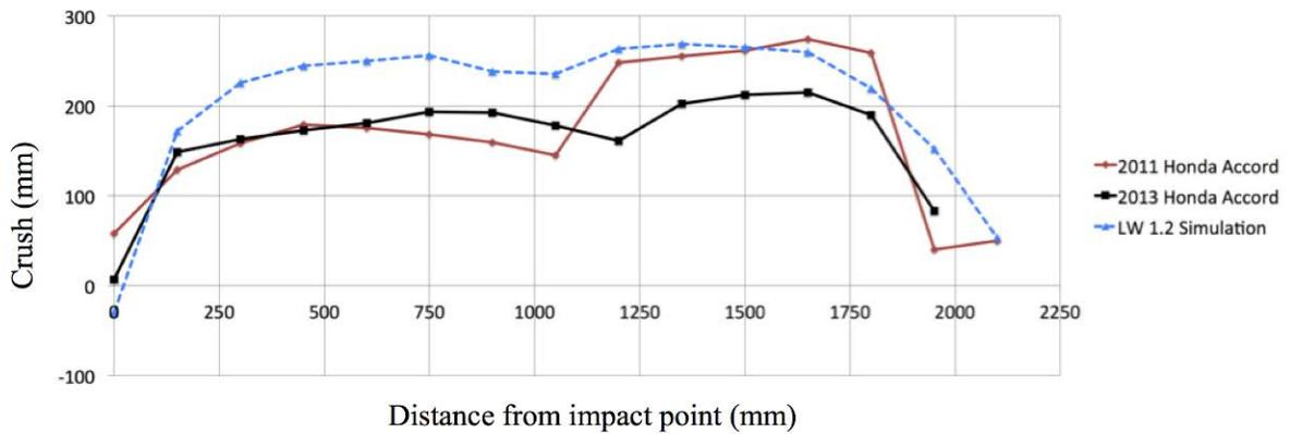
Figure 118: Exterior crush for level 3, approximately the mid-door level in NCAP MDB side test
