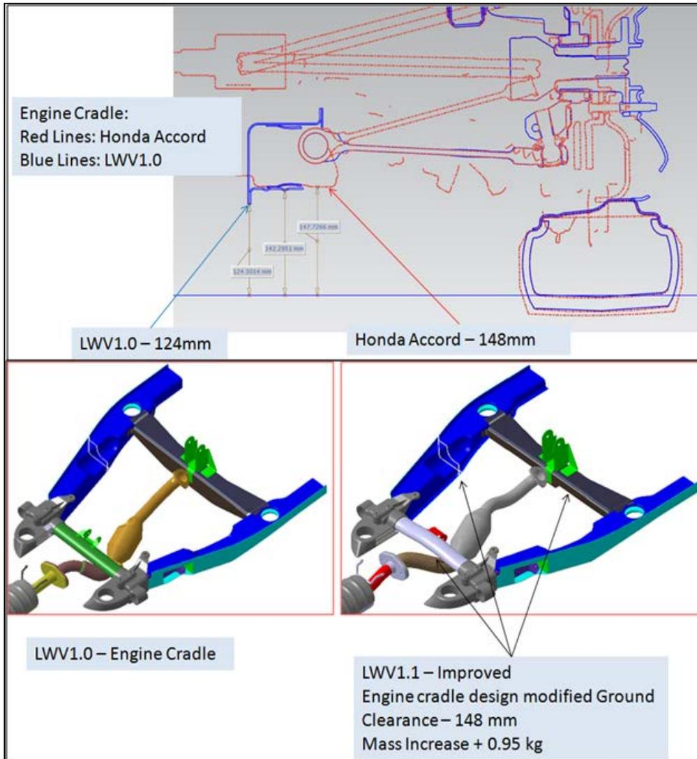
**Figure 89: Ground clearance increased by modification to engine cradle**
