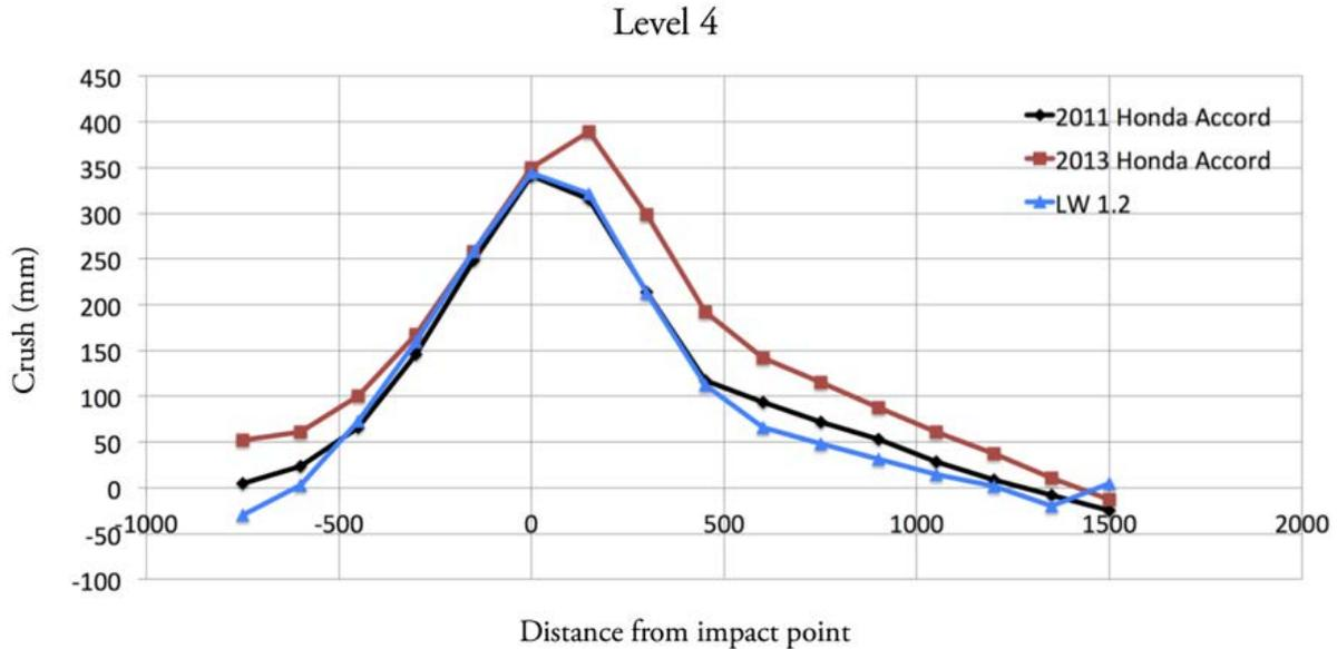
**Figure 129: Exterior crush for level 4, approximately window sill level in the lateral pole test**
