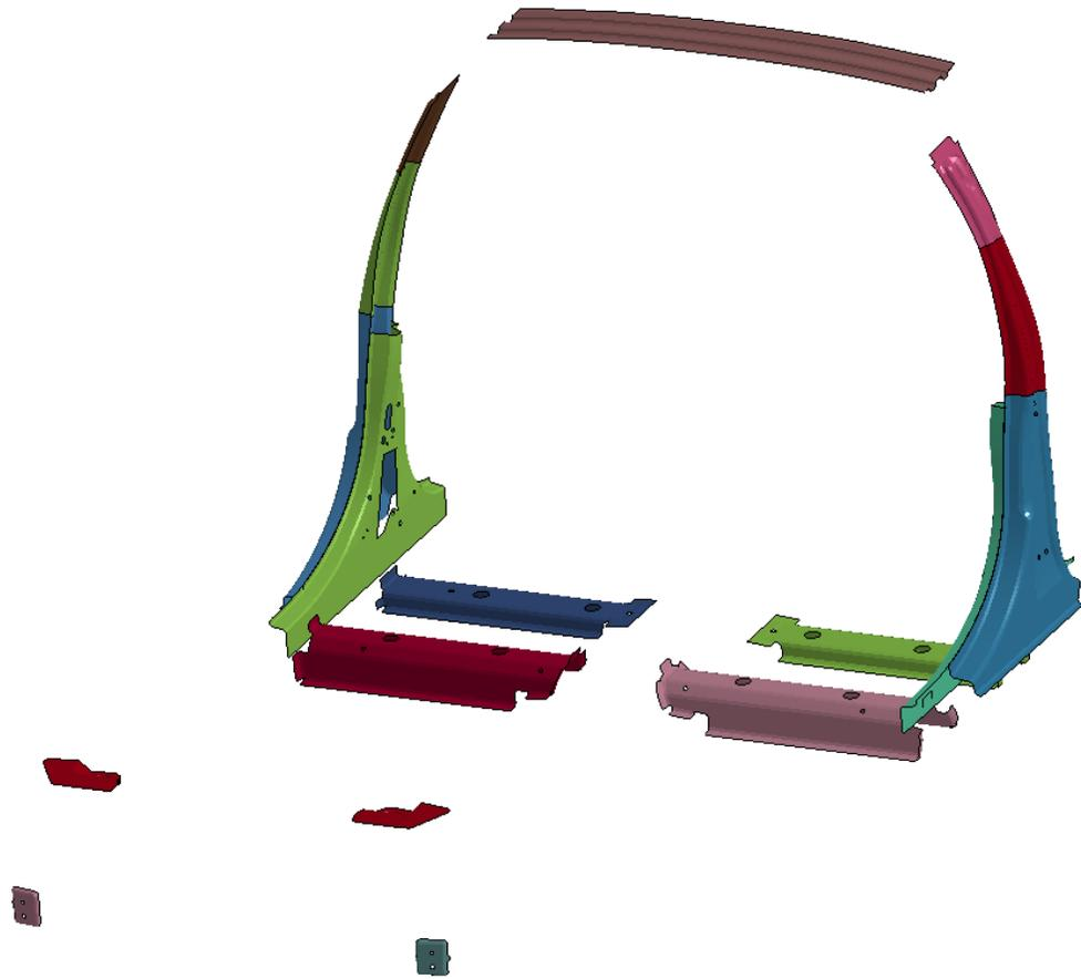
Figure 153: Parts with materials changed from high-strength to lower-strength steels
