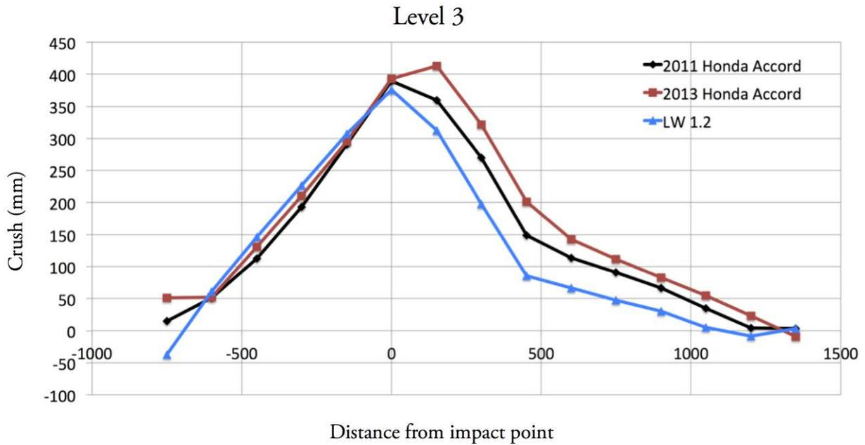
**Figure 128: Exterior crush for level 3, approximately the mid-door level in the lateral pole test**
