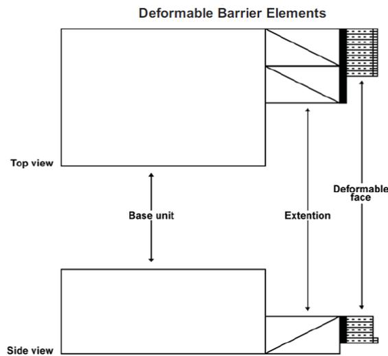
Figure 29: Deformable barrier used in IIHS frontal 40 percent offset barrier test<sup>45</sup>
