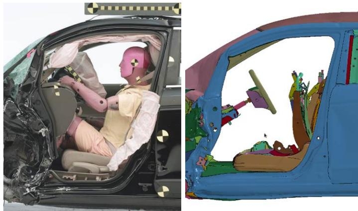
**Figure 79: Occupant compartment deformation profile for laboratory test and simulation for IIHS SOL test**
