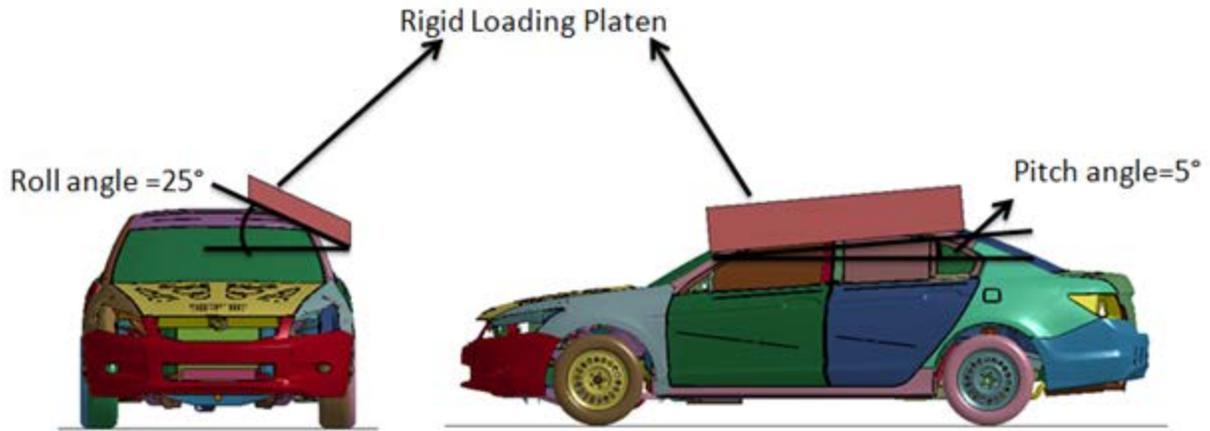
Figure 130: LS-DYNA set-up for the IIHS roof crush test
