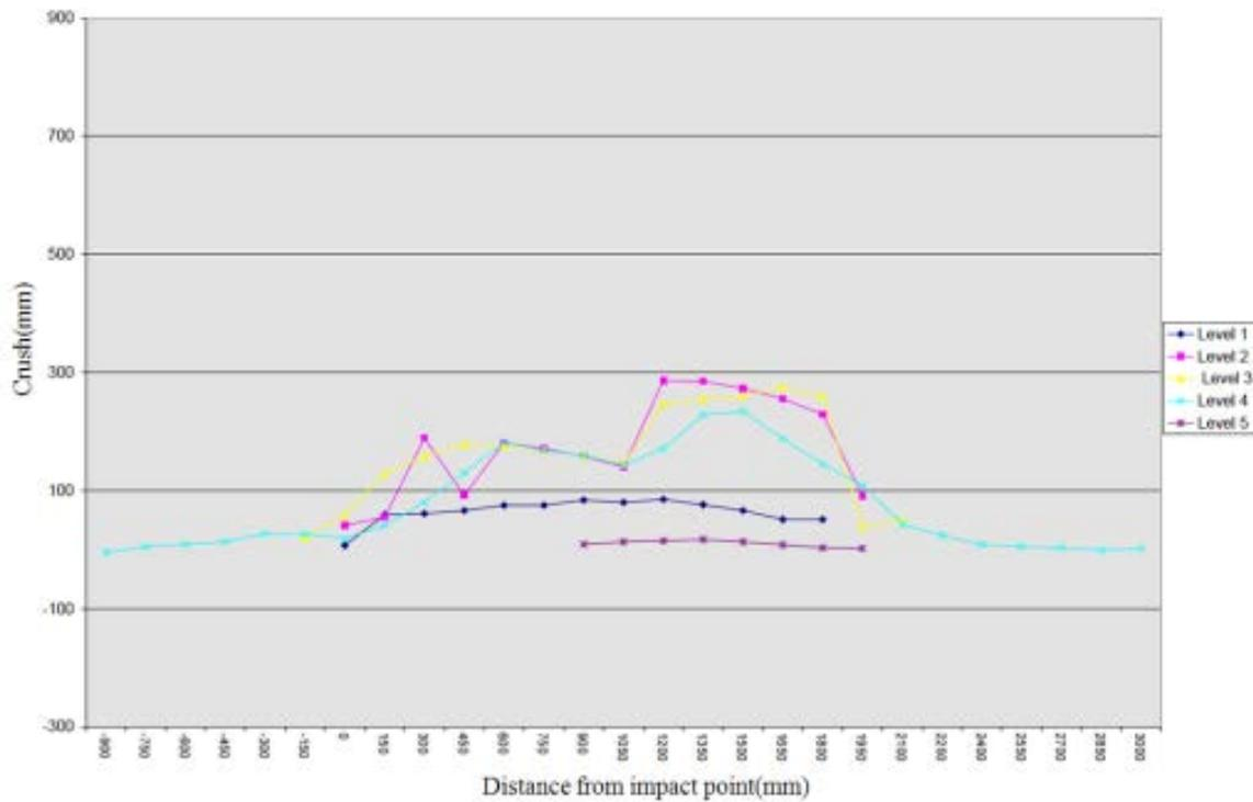
Figure 13: Measurements of crush of Honda Accord 2011 in NCAP moving barrier side test<sup>21</sup>
