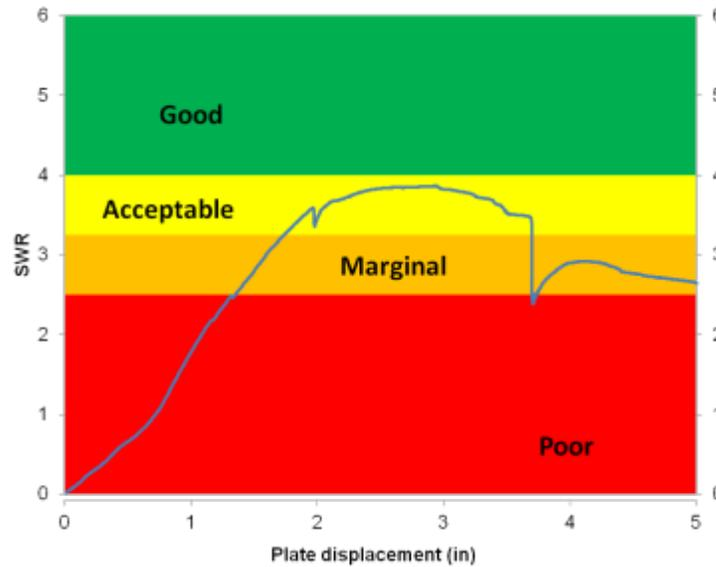
Figure 22: Honda Accord was rated “acceptable” in the IIHS roof crush test<sup>35</sup>
