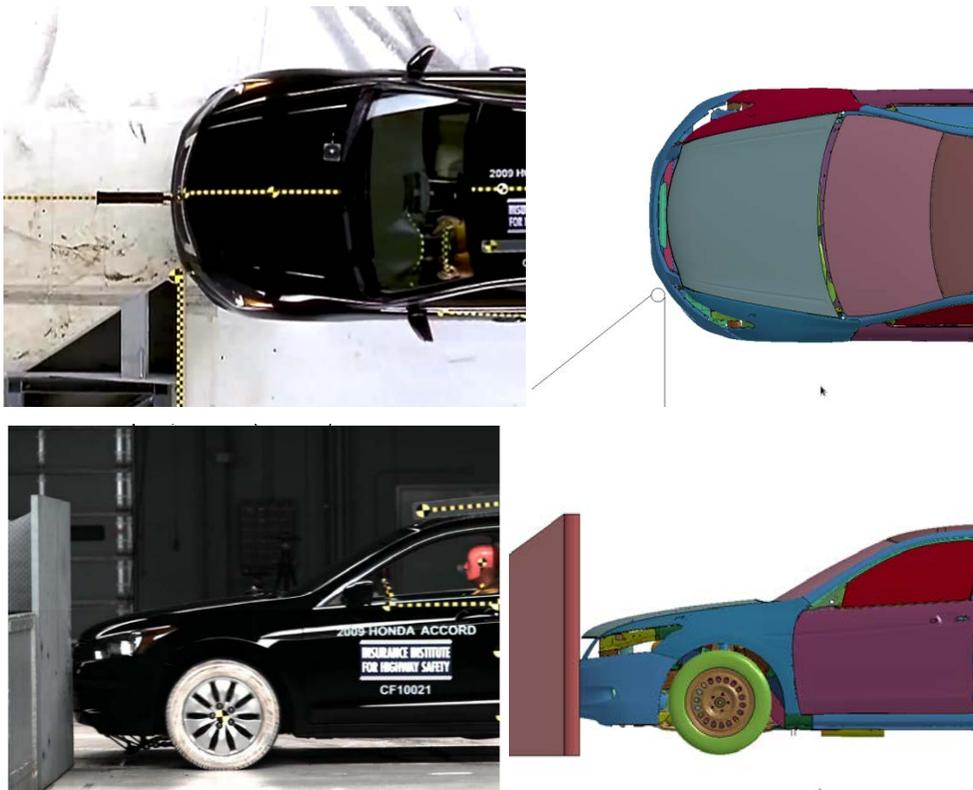
**Figure 77: Pre-test laboratory vehicle and model of the 2009 Honda Accord for IIHS SOL test**
