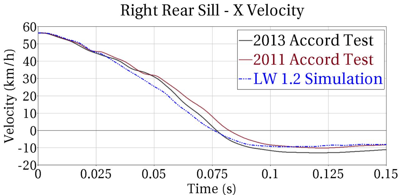
Figure 113: Velocity of MY2011 and MY2013 Honda Accord and LWV 1.2 for right-rear sill in rigid wall crash
