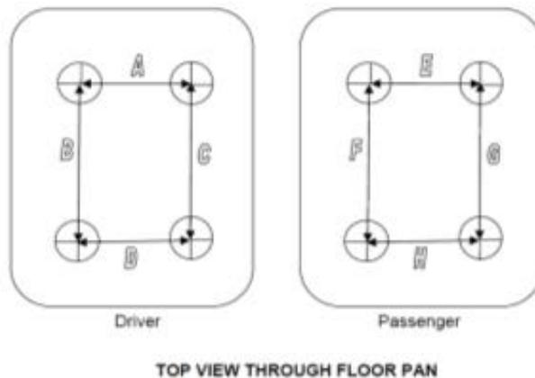
**Figure 7: Scheme used to measure under-body floorboard deformation<sup>12</sup>**
