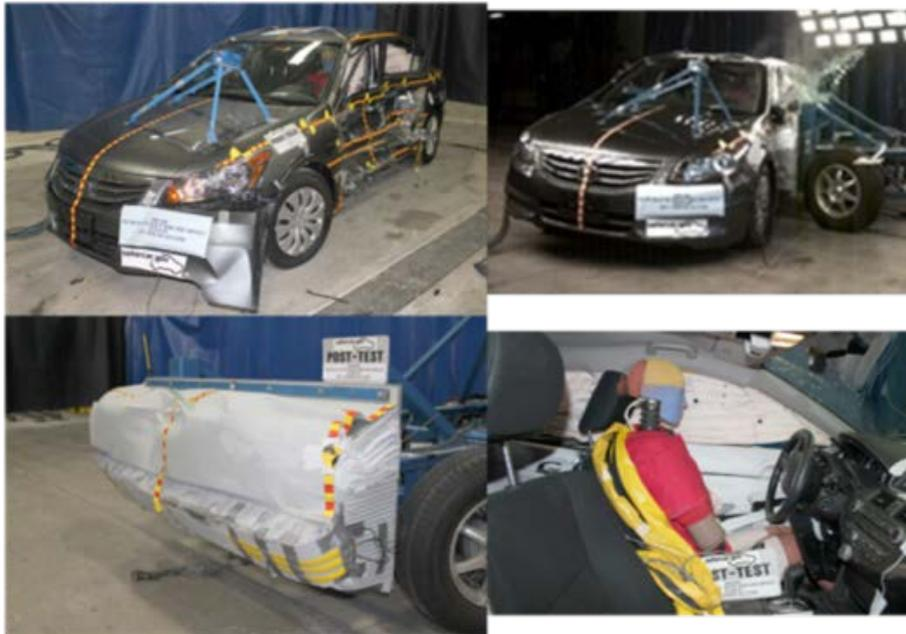
Figure 11: Test set-up and the post-crash vehicle of the NCAP side impact test with moving deformable barrier<sup>17</sup>
