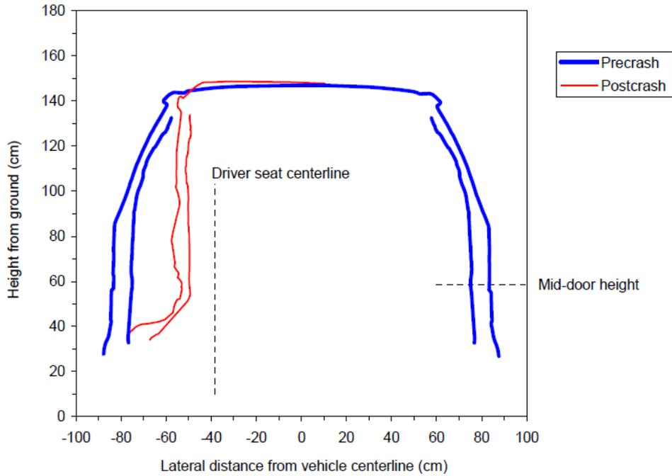
Figure 25: B-pillar exterior and interior profile for 2008 Honda Accord<sup>40</sup>
