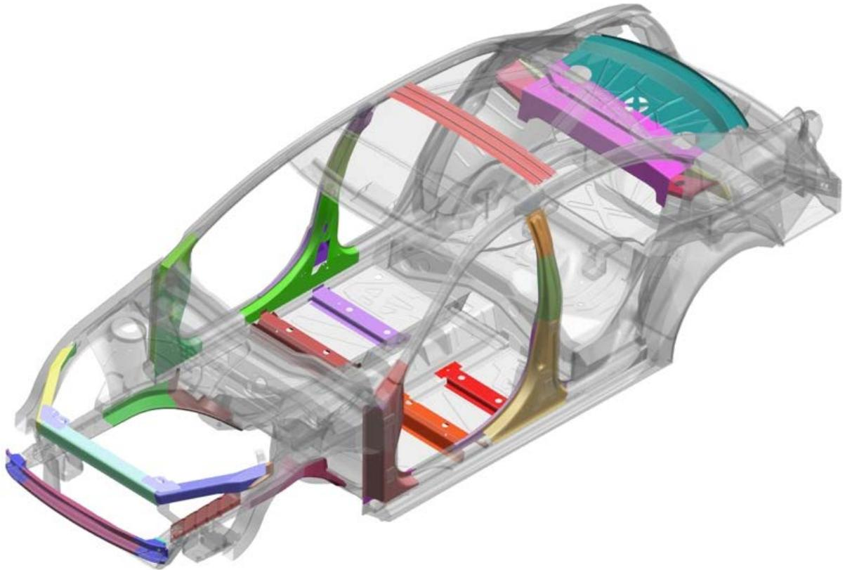
**Figure 84: Changes to body structure – thickness and steel grades were changed for the highlighted panels**
