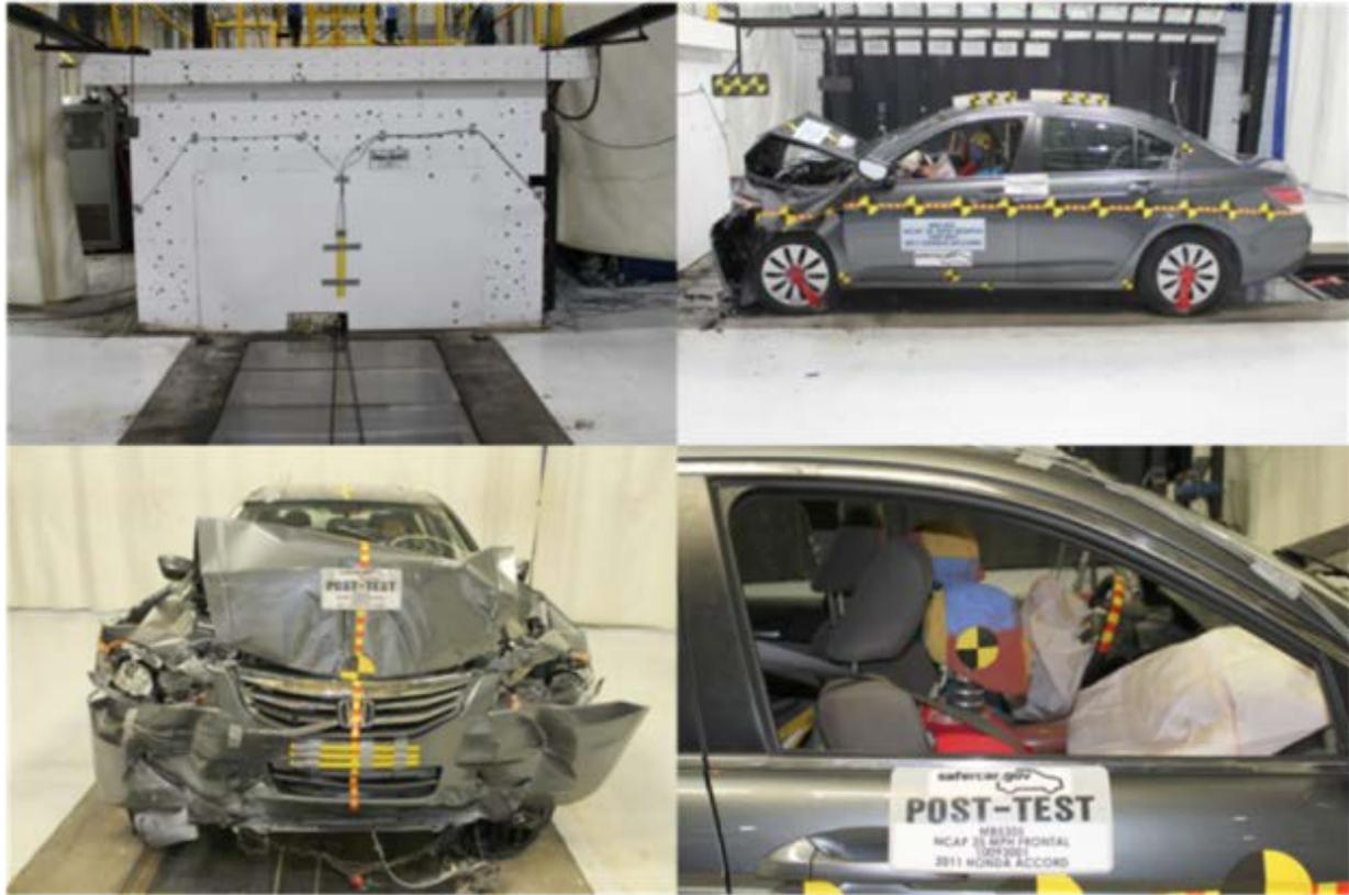
**Figure 5: Test set-up and the post-crash vehicle of the NCAP frontal crash<sup>8</sup>**
