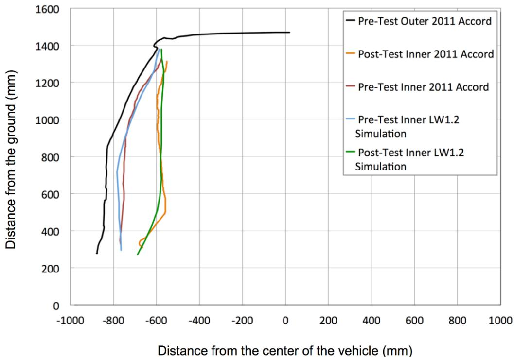
**Figure 119: Pre- and post-crush and intrusion for the LWV 1.2 in the NCAP lateral test**
