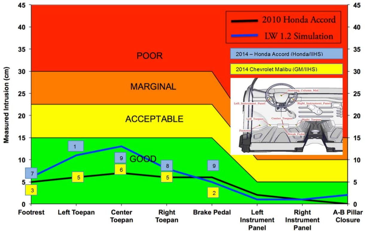
Figure 141: LWV 1.2 IIHS Moderate Overlap Frontal Impact – Intrusion Comparisons with 2014 Accord and Malibu
