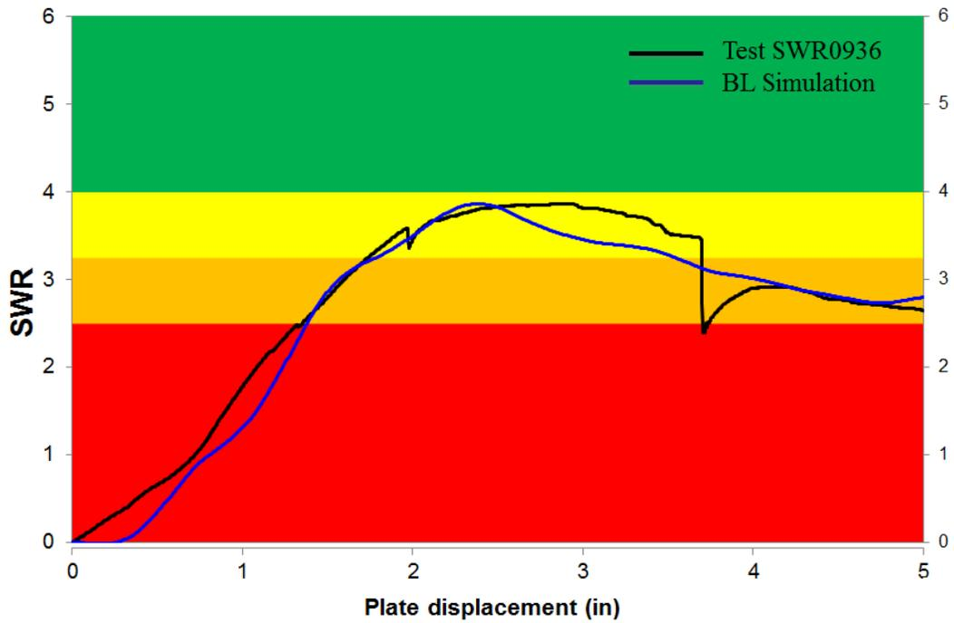
Figure 62: Model and Test #SWR 0936 IIHS Side SWR Versus Platen Displacement Overlay
