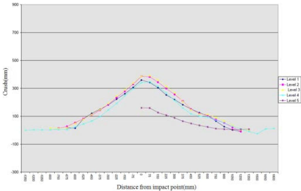
Figure 18: Measurements of crush of Honda Accord 2011 in NCAP rigid pole side test<sup>29</sup>
