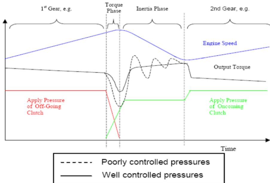
**Figure 30 – Generic Shift Process for Automatic Transmission**
