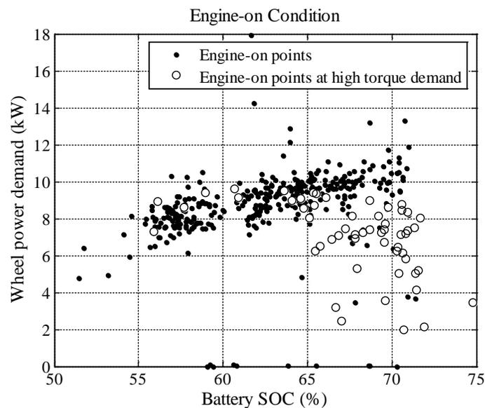
**Figure 39 – Engine-On Condition – 2010 Prius Example Based on 25 Test Cycles**
