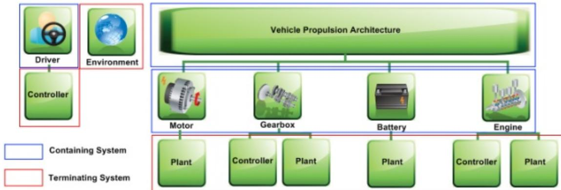
**Figure 6 – Class Diagram of Container and Terminating Systems**
