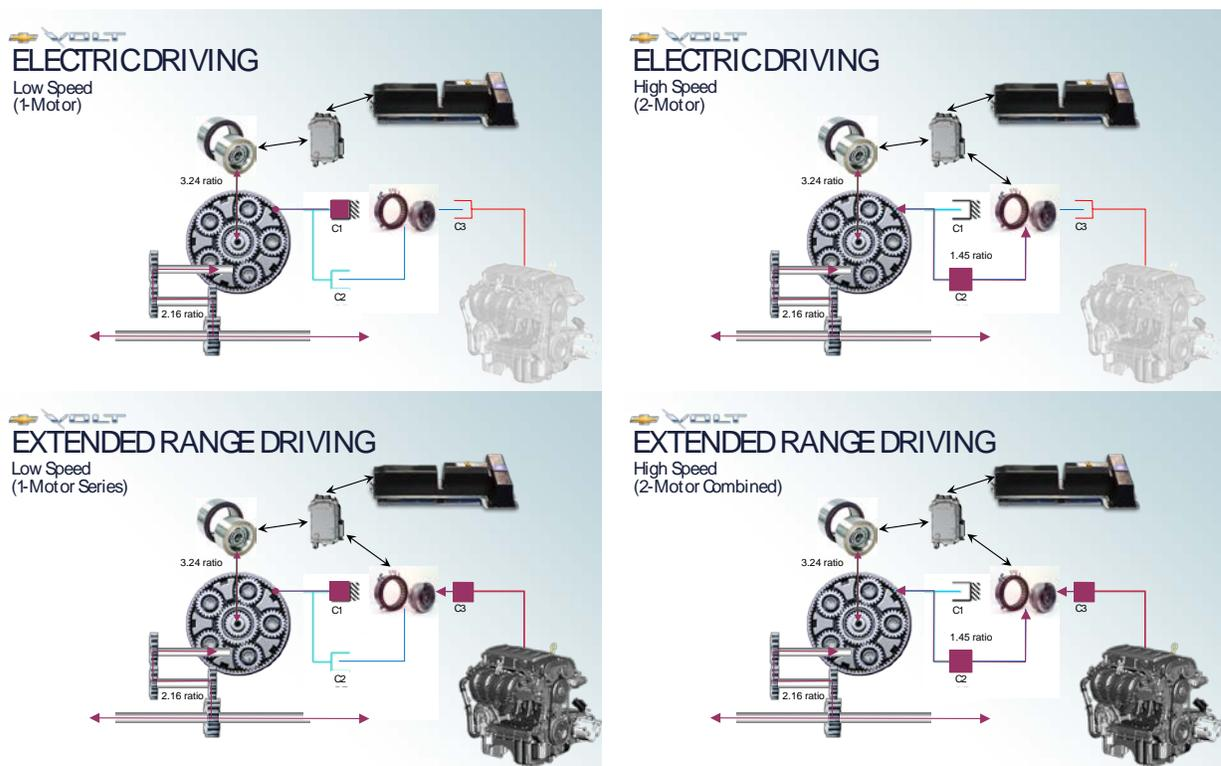
Figure 42 – Voltec Operating Modes [www.gm.com]
