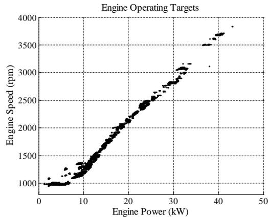
**Figure 41 – Example of Engine Operating Target – 2010 Prius Example Based on 25 Test Cycles**
