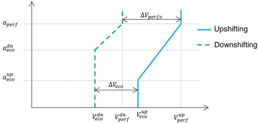
Figure 29 – Design of Upshifting and Downshifting Speed Curves for Two Adjacent Gears
