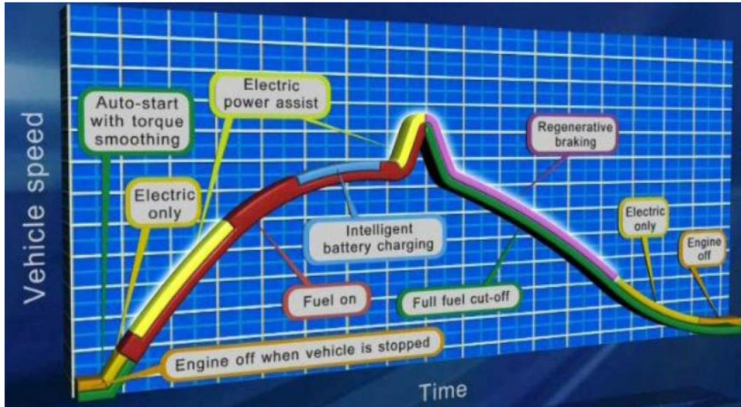
**Figure 23 – Hybrid Electric Vehicle Principles [source: [www.gm.com](http://www.gm.com)]**
