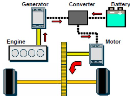
**Figure 19 – Series Hybrid Electric Vehicle**
