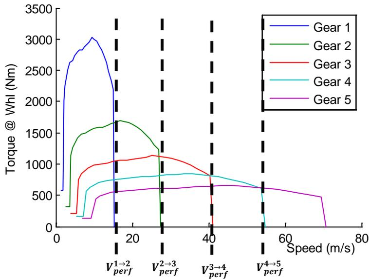
Figure 28 – Maximum Engine Torque at Wheels and Performance Upshift Speeds
