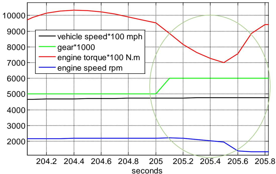
**Figure 31 – Torque Hole in Autonomie during Shifting Event**
