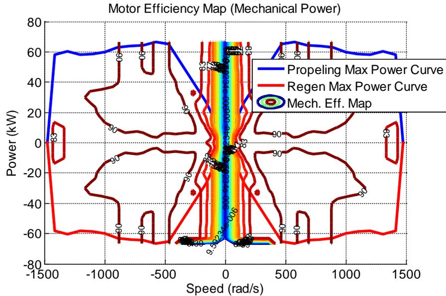
Figure 38 – Electric Machine Map for Full HEV
