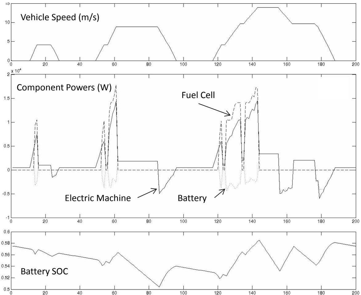
**Figure 43 – Component Operating Conditions of a Fuel Cell Vehicle on the Urban European Drive Cycle using Dynamic Programming**
