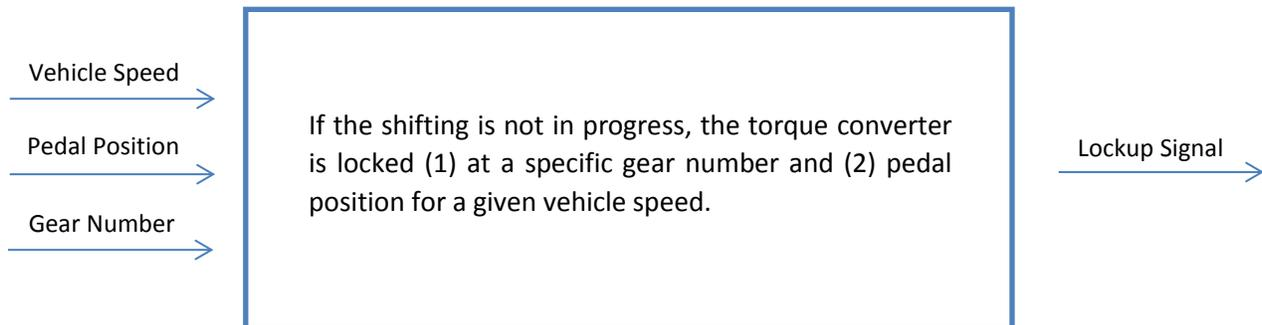
**Figure 36 – Torque Converter Lockup Control Algorithm**
