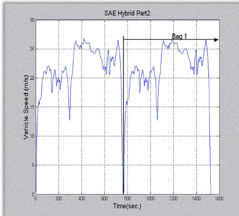
**Figure 47 - The highway cycle for a hybrid vehicle (Only the results from the second cycle were used)**
