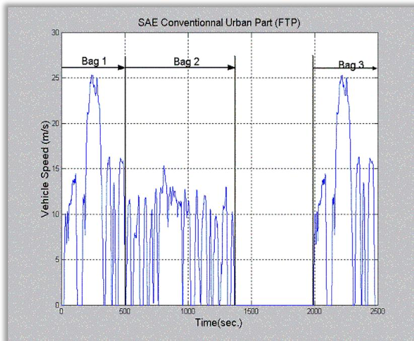
**Figure 44 - The urban cycle for a non-hybrid vehicle**
