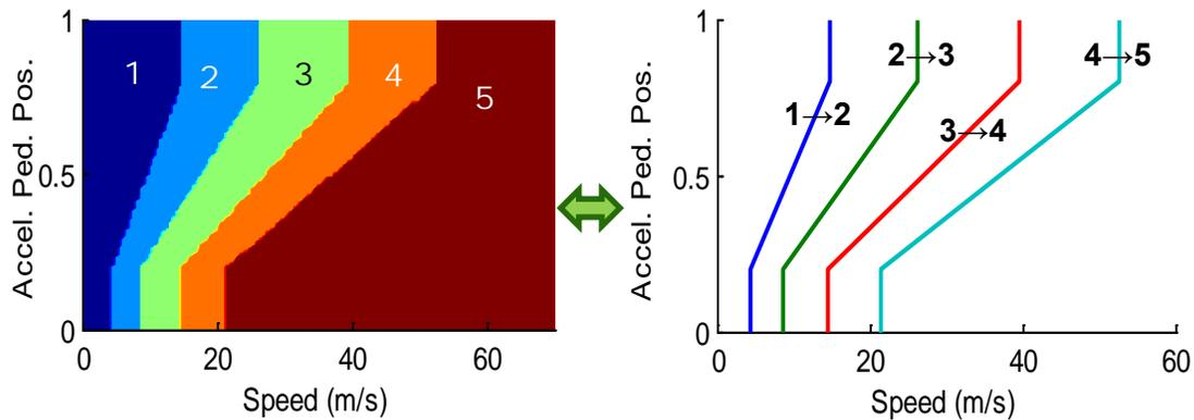
Figure 26 – Upshifting Gear Map (left), Upshifting Vehicle Speeds (right)
