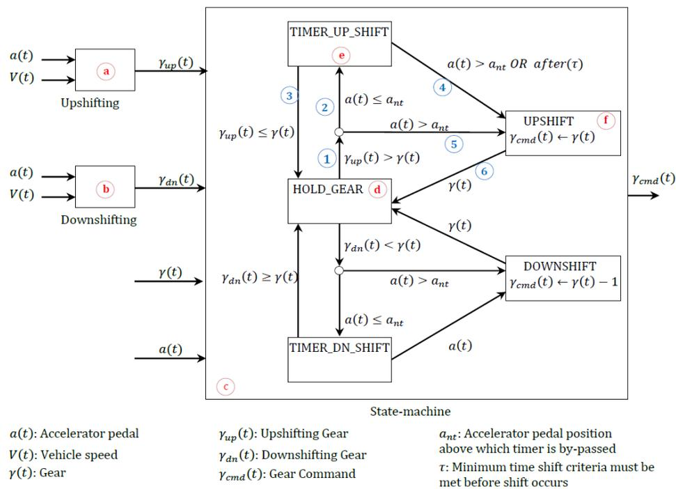
**Figure 25 – Shifting Controller Schematic**
