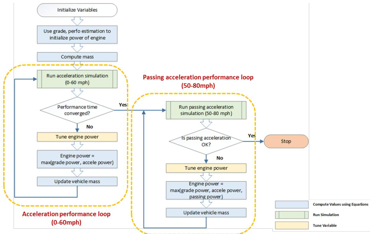
**Figure 57 – Conventional Powertrain Sizing Algorithm**
