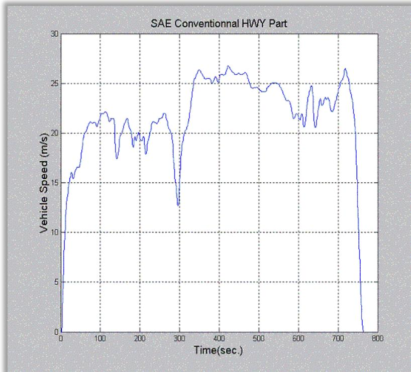
**Figure 45 - The highway cycle for a non-hybrid vehicle**
