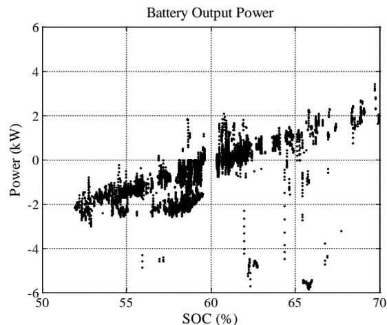
**Figure 40 – SOC Regulation Algorithm – 2010 Prius Example Based on 25 Test Cycles**
