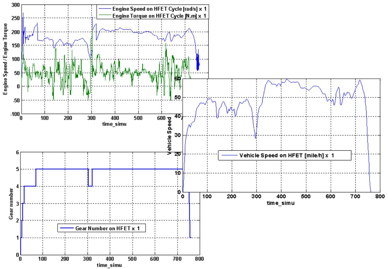
Figure 65 – Engine Speed, Engine Torque, Gear Number, and Vehicle Speed Time-Based Signals on HFET Cycle.
