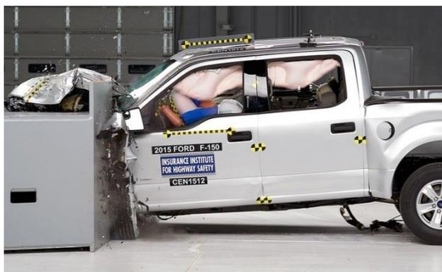
**Figure B.31 Aluminum F150 Crew Cab Performances in IIHS Small Overlap Crash Test<sup>71</sup>**
