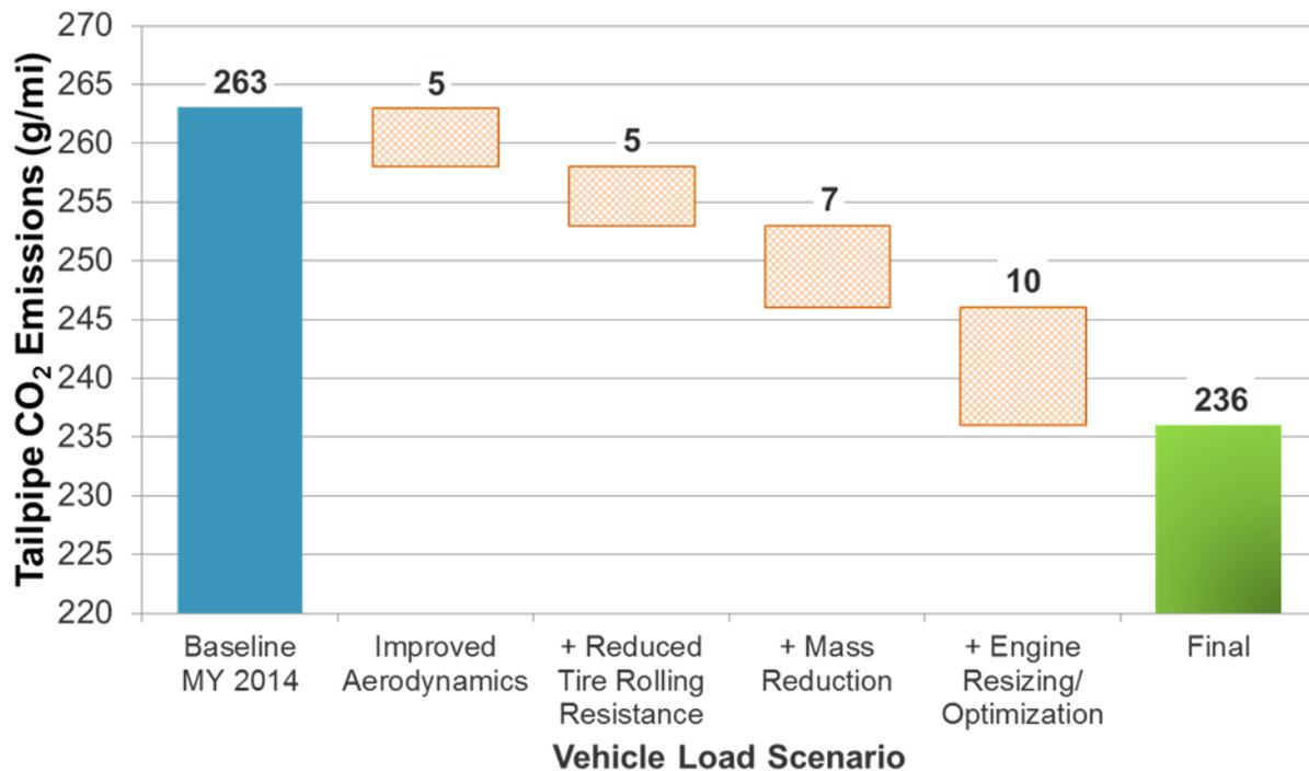
**Figure A.1 Potential Reduction in CO<sub>2</sub> Emissions by Adoption of Best-In-Class MY2014 Technologies**
