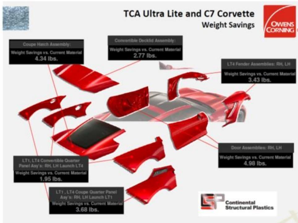
Figure B.46 Part -By Part Weight Savings Realized By Improving the SMC Formulation Used In the C7 Corvette
