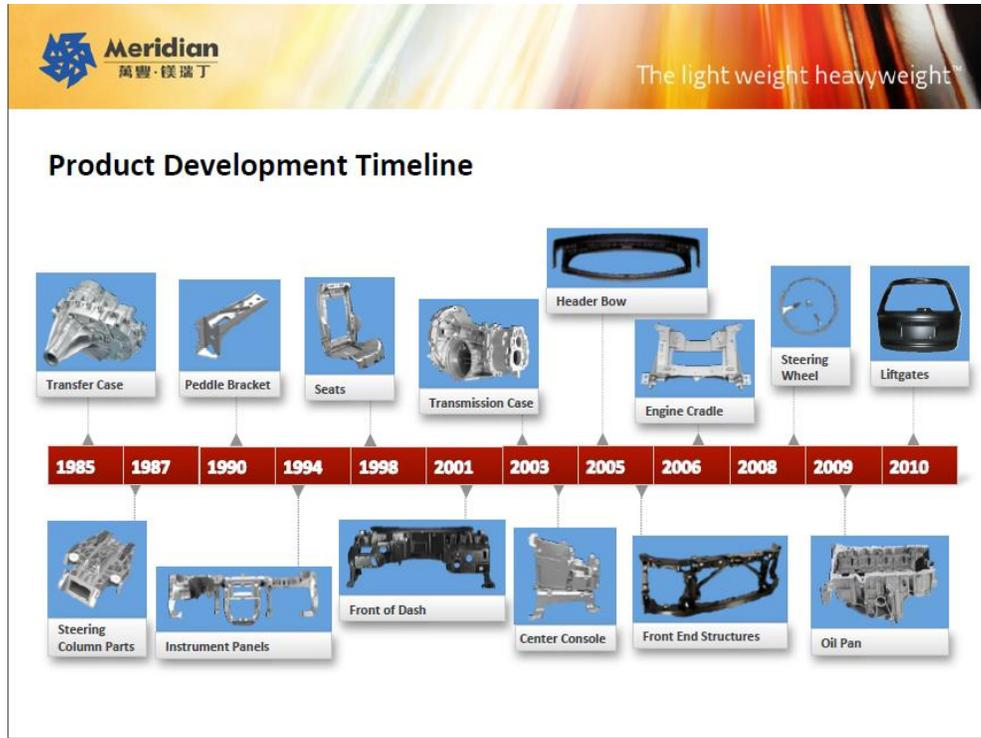
Figure B.38 Product Development Timeline for Magnesium Automotive Components, Meridian<sup>82</sup>
