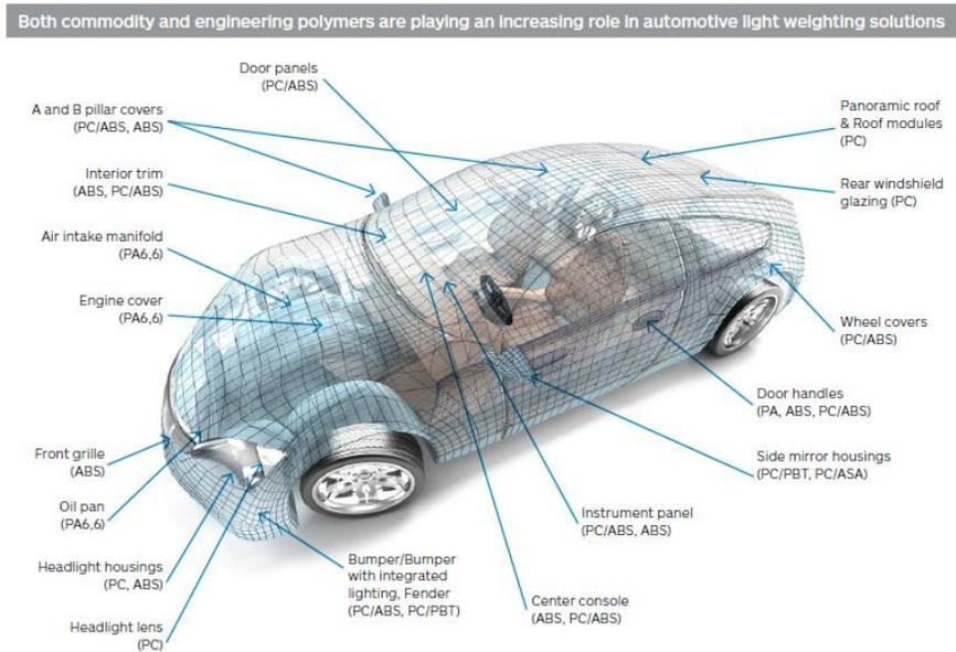
Figure B.48 Commodity and Engineering Polymers are Playing an Increasing Role in Automotive Light Weighting Solutions<sup>99</sup>
