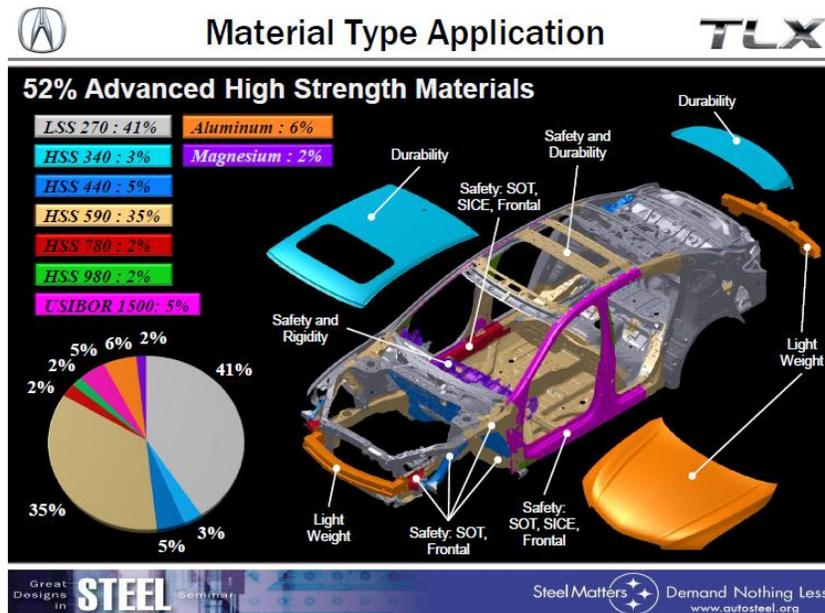
Figure B.7 Material Type Application for the Acura TLX Presented at 2015 Great Designs in Steel<sup>25</sup>
