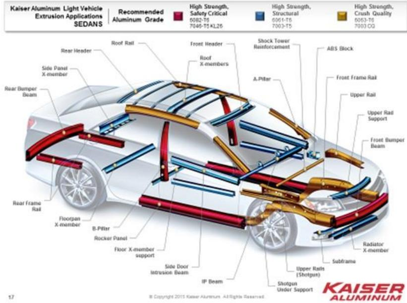
Figure B.25 Kaiser Aluminum Light Vehicle Extrusion Applications in Sedans<sup>63</sup>
