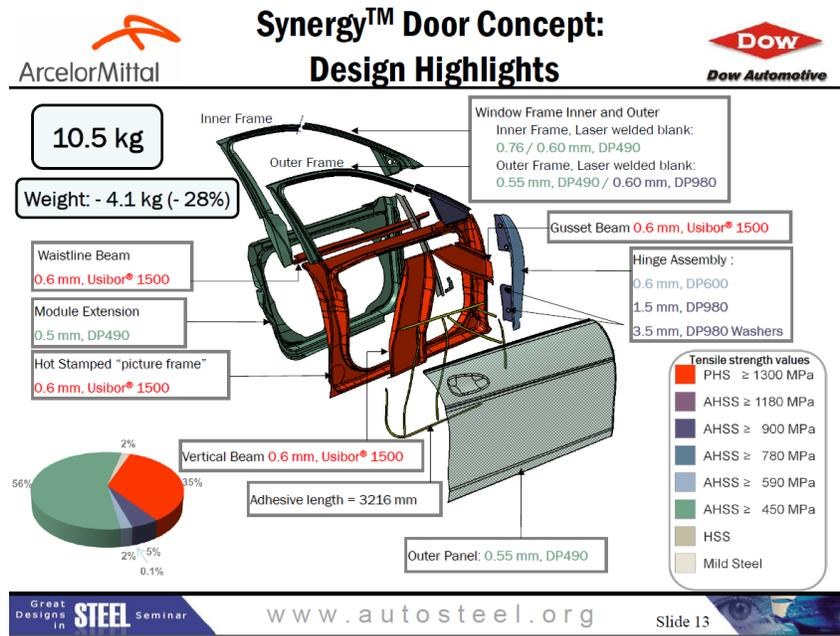
Figure B.4 Arcelor Mittal's Synergy Door Concept Design Highlights<sup>15</sup>
