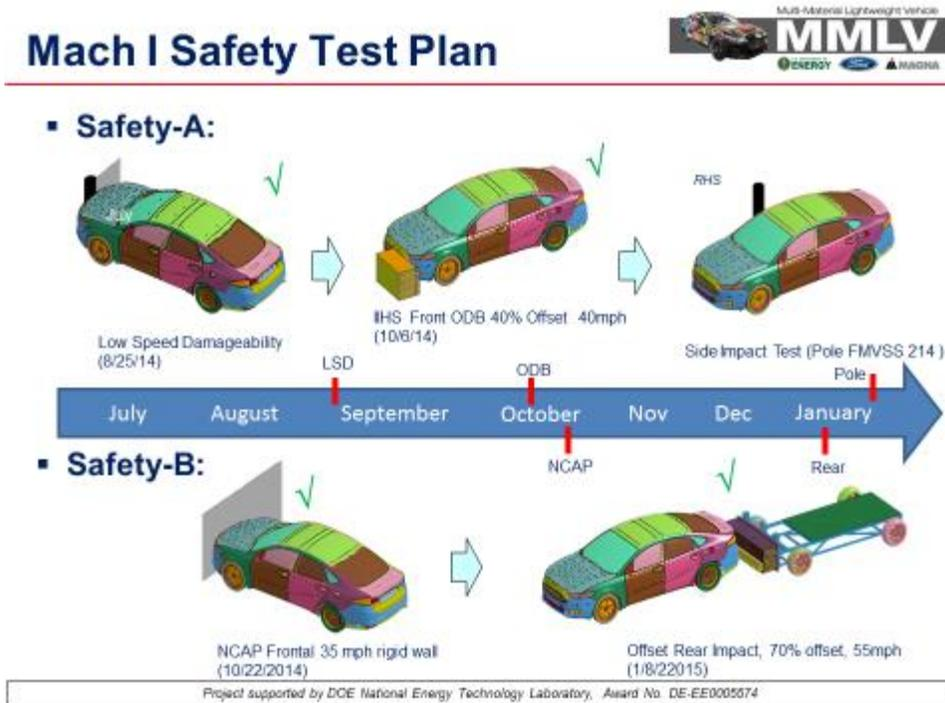
Figure B.58 Mach I Crash Safety Test Plan<sup>139</sup>
