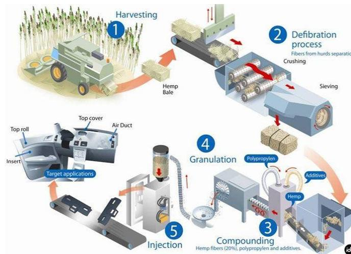
**Figure B.49 NAFILean Biomass Source for Fibers and Introduction into the Automobile<sup>114</sup>**
