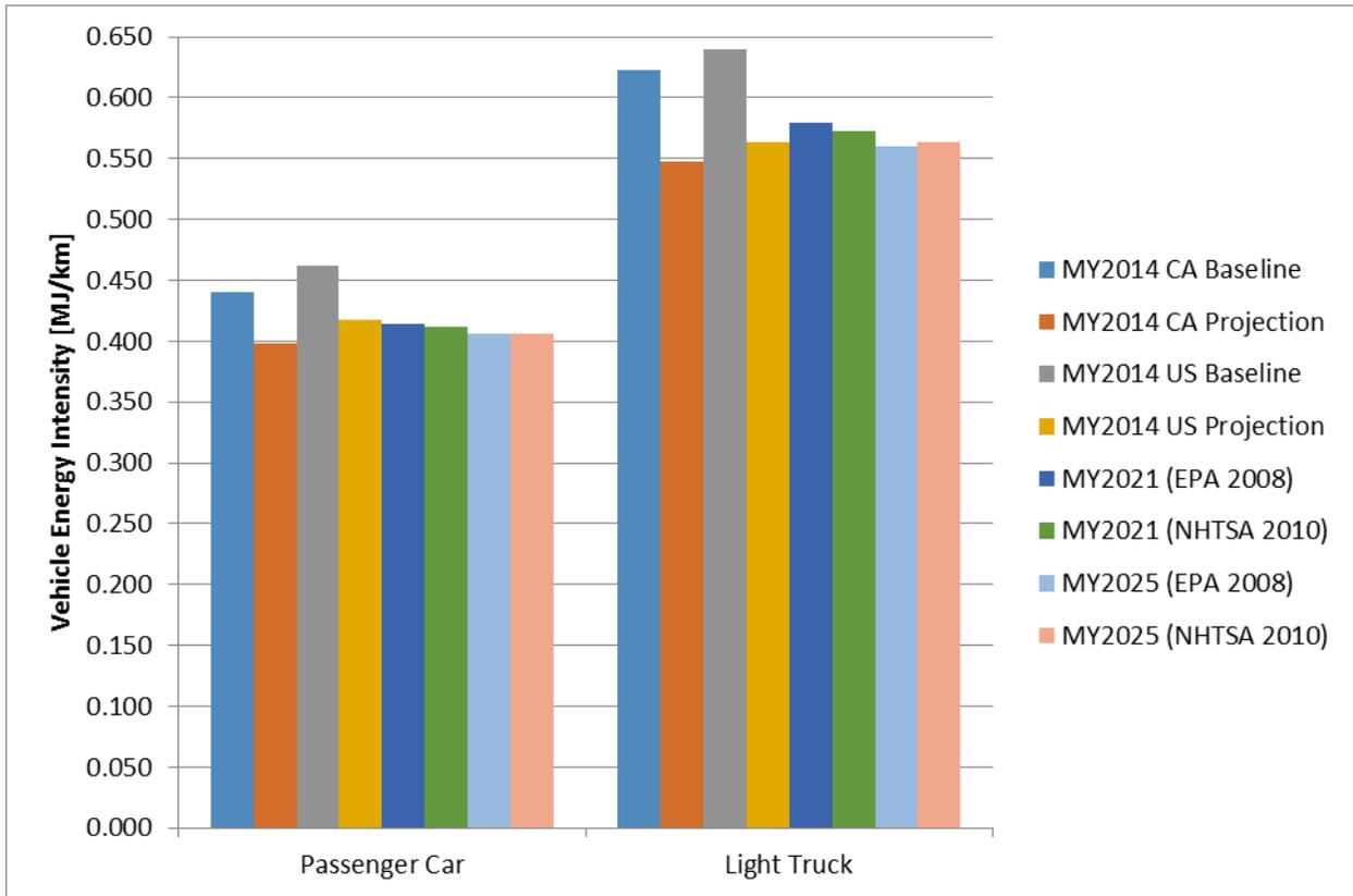
**Figure A.2 Sales-Weighted Vehicle Energy Intensity**
