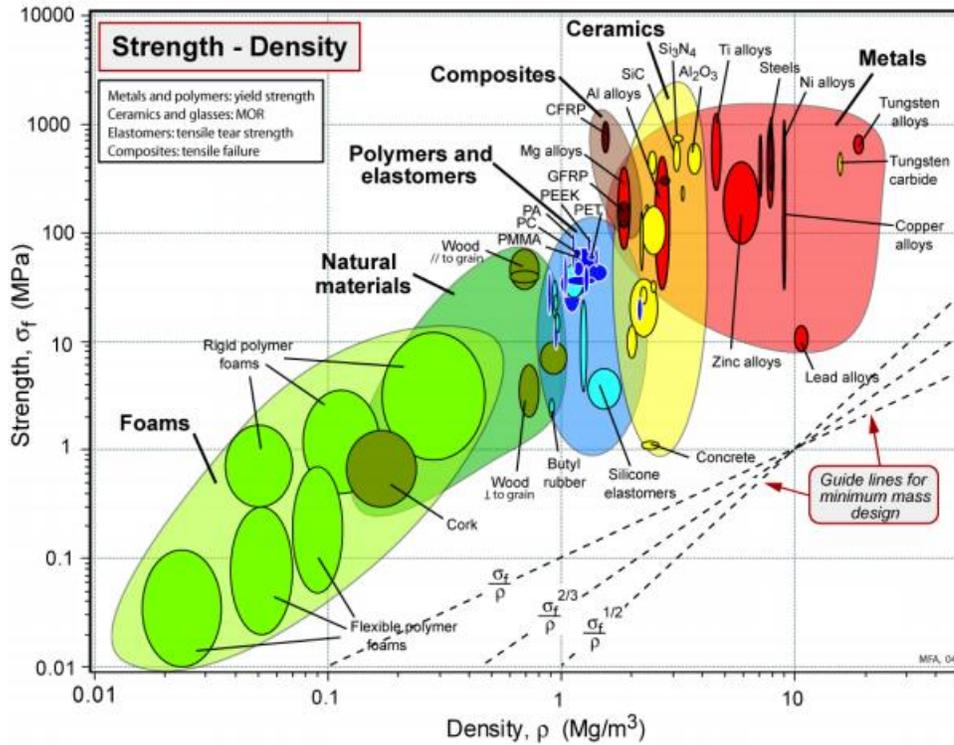
Figure B.1 Ashby Plot for Material Strength-Density<sup>7</sup>
