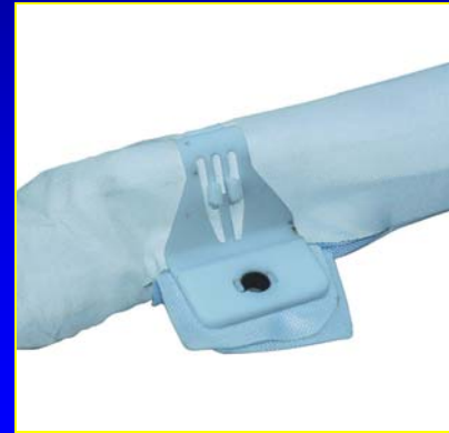
Roof Rail-AB Modul (Detail)
