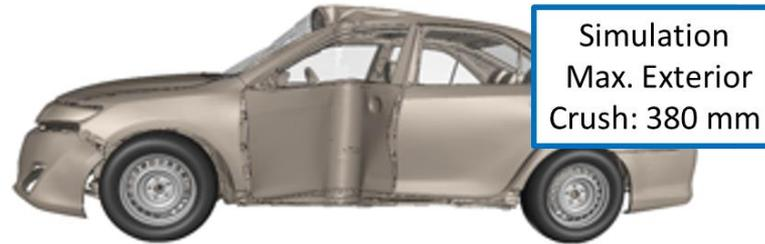
Test and simulation showed excellent correlation with respect to vehicle pulse, and maximum exterior vehicle deformation
