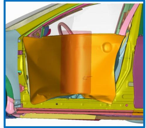
Test and simulation showed good correlation with respect to resistance force versus intrusion, initial, intermediate, and peak force values
