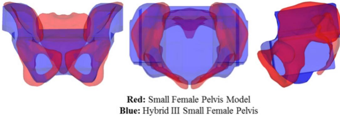
**Figure 2. Comparison of symmetric SFPM geometry and Hybrid III geometry.**
