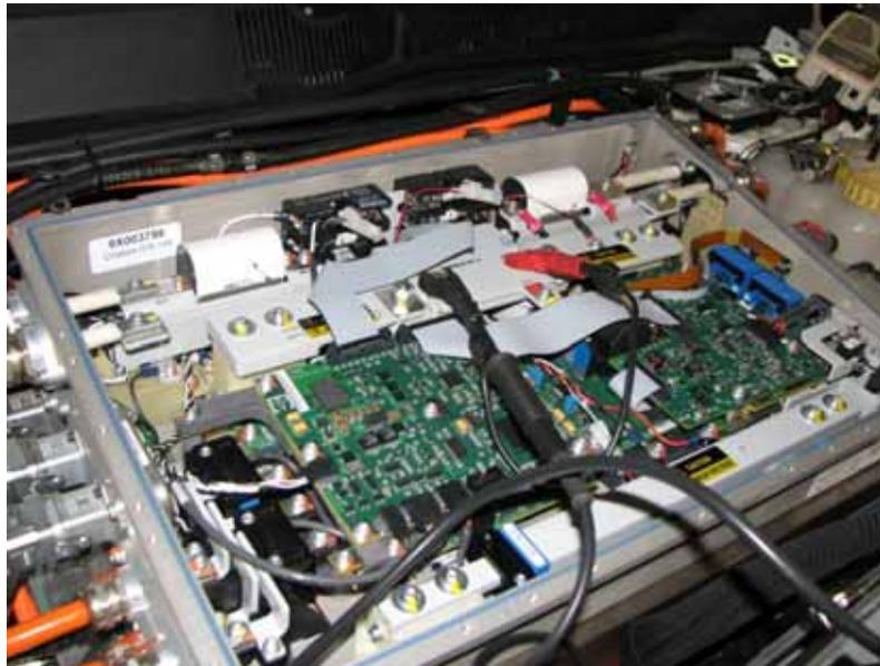
**Figure 2. Megohmmeter Equinox connections.**
