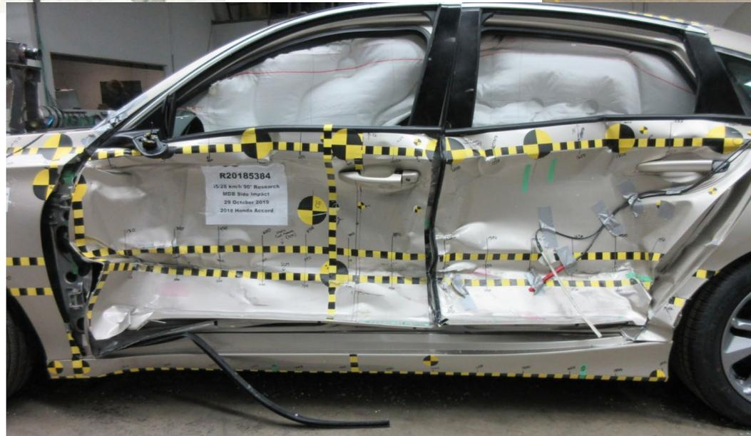
MDB impact location in test at Lab 3 was rearward of target
