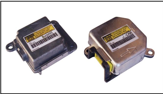
Figure 1 - SDM-G (left) and SDM-R (right)
