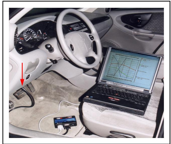
Figure 3 - CDR Connected to DLC
