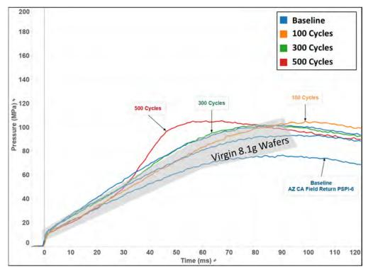
Figure 17. Closed chamber test pressure-time histories for field returned 2004 propellant cycled (2-95°C, 3 hours/cycle) in 77 mL chambers. (The baseline data were obtained from the population of PSPI-6 field samples [8.1 g wafers] that were used in the subsequent cycling.)
