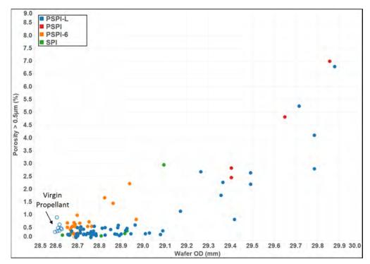
Figure 9. MIP porosity above 0.5 μm pore diameter versus OD for propellant wafers from different inflator designs. (The nominal OD for virgin wafers is 28.6 mm, as denoted by the hollow circles.)
