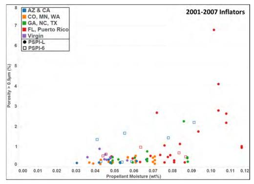
Figure 7. MIP porosity versus propellant moisture for 2001-2007 inflators from selected states.
