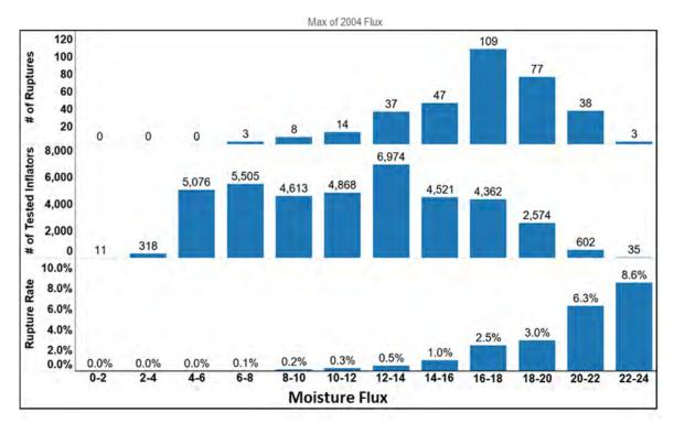
Figure 21. Rate of PSPI-L inflator rupture in Takata testing as compared to the calculated 2004 propellant moisture flux. No ruptures occurred below 7.6% moisture flux as calculated using the parameters specified in the model.
