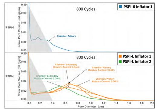
Figure 13. MIP pore size distribution of virgin inflators cycled 800 times (2-80°C, 4 hours/ cycle).
