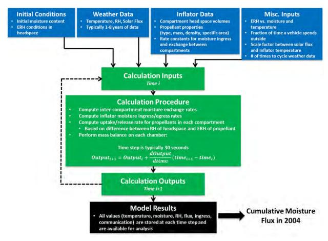
Figure 18. Summary of the inputs, assumptions, and calculation procedure in the Exponent numerical model for tracking moisture movement in the inflator.
