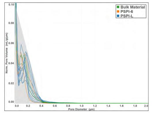
Figure 5. MIP pore size distribution for a variety of virgin 2004 propellants. (Bulk material refers to pressed 2004 propellant received directly from Takata prior to assembly into any inflators. Similarly, test material for PSPI-6 and PSPI-L was extracted from virgin inflators.)
