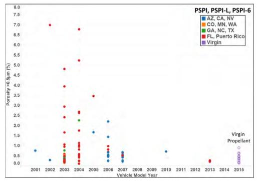
Figure 8. MIP porosity (for pore size above 0.5 μm) in 2004 wafers from inflators of different model year and location of operation.
