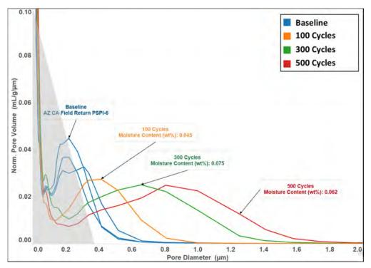
Figure 16. MIP pore size distribution of field returned 2004 propellant cycled (2-95°C, 3 hours/cycle) in 77 mL chambers. (The baseline data were obtained from the population of 2007 model year Arizona and California field samples that were used in the subsequent cycling.)
